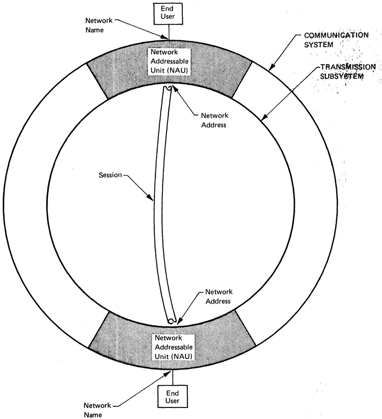
Figure 2-3. Basic SNA structure
