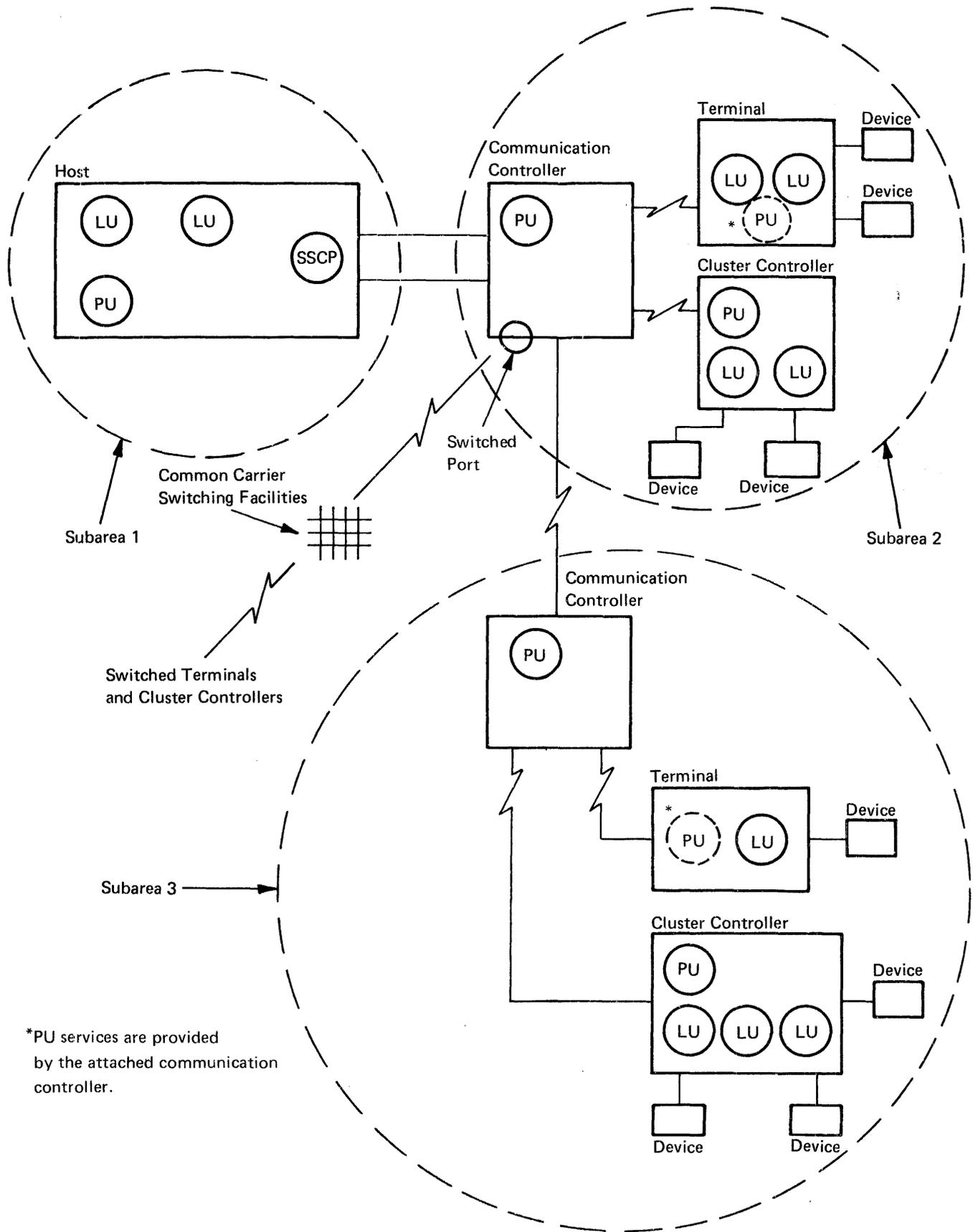
Figure 3-3. Physical Configuration of Subareas
