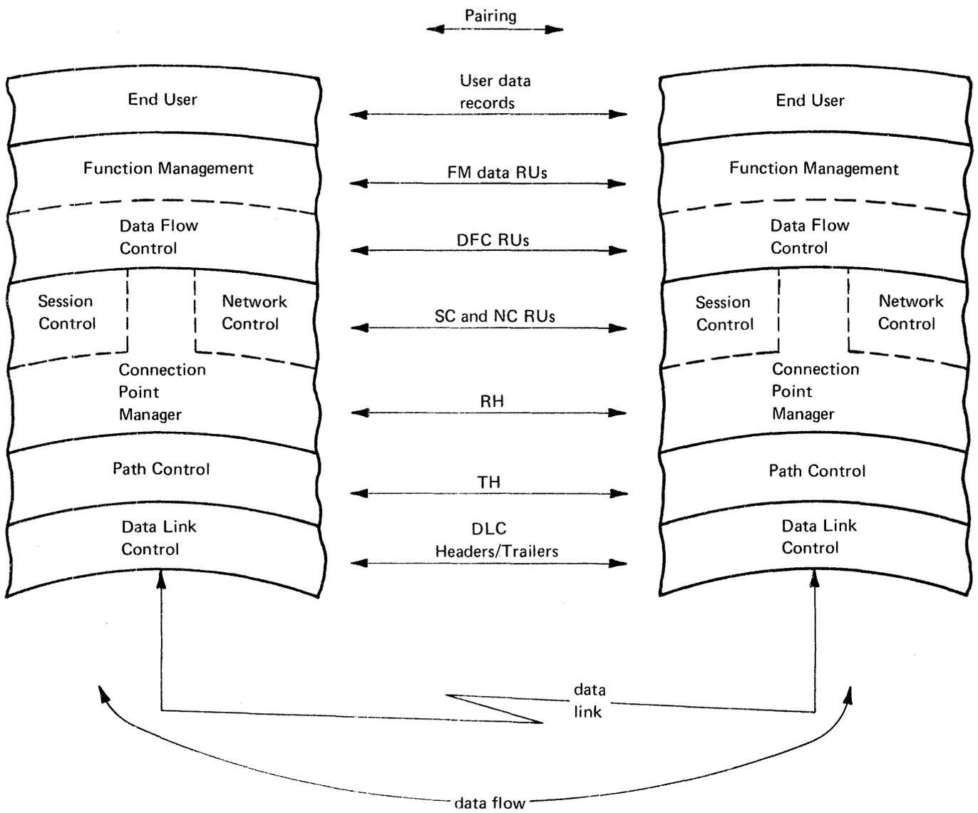
Figure 4-1. SNA Internal Communication
