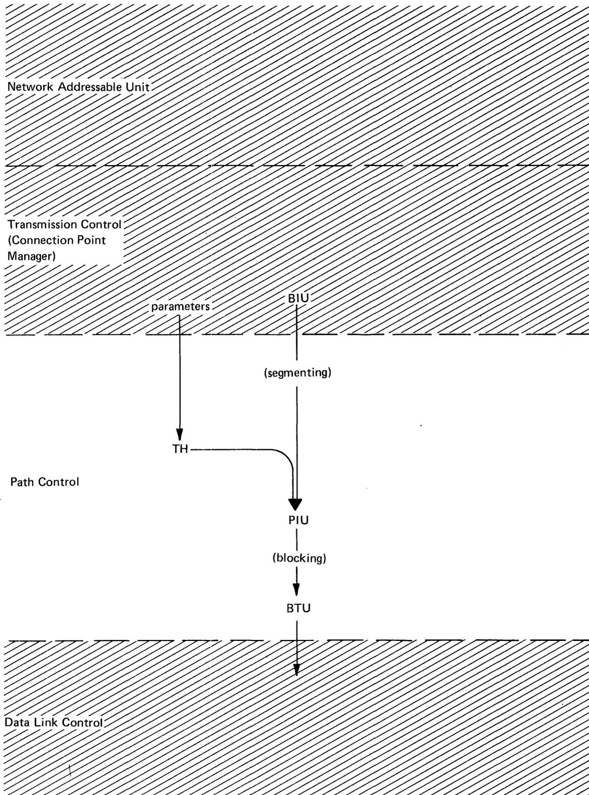
Figure 2-9. Path Information Unit (PIU) and Basic Transmission Unit (BTU)
