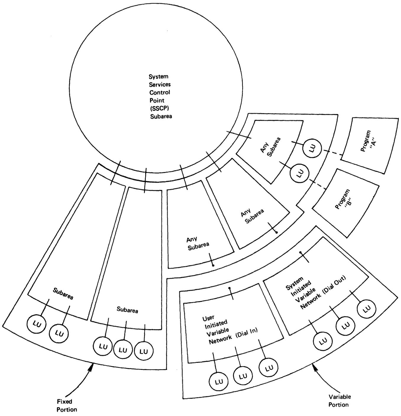
Figure 3-2. Logical Configuration of Subareas
