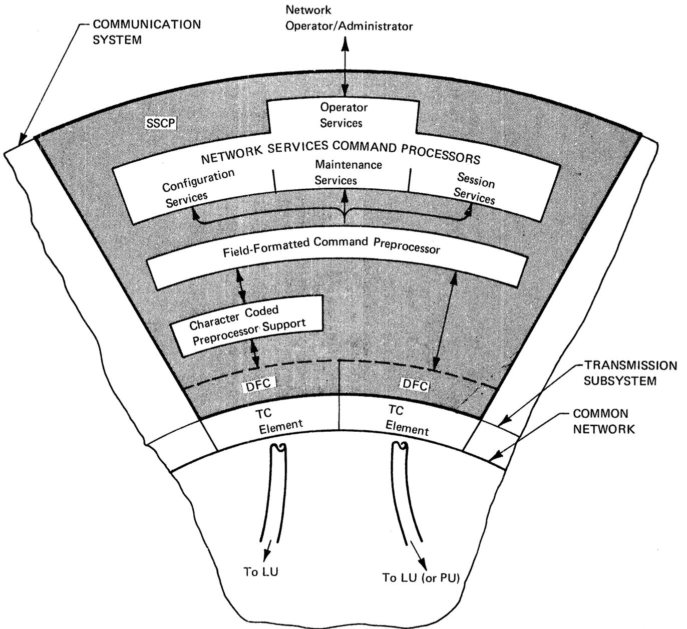
Figure 2-15. System Services Control Point (SSCP)
