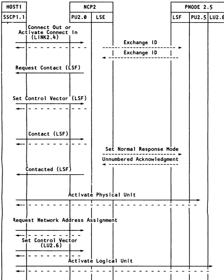
Activating a Peripheral Node Attached via a Switched SDLC Link
