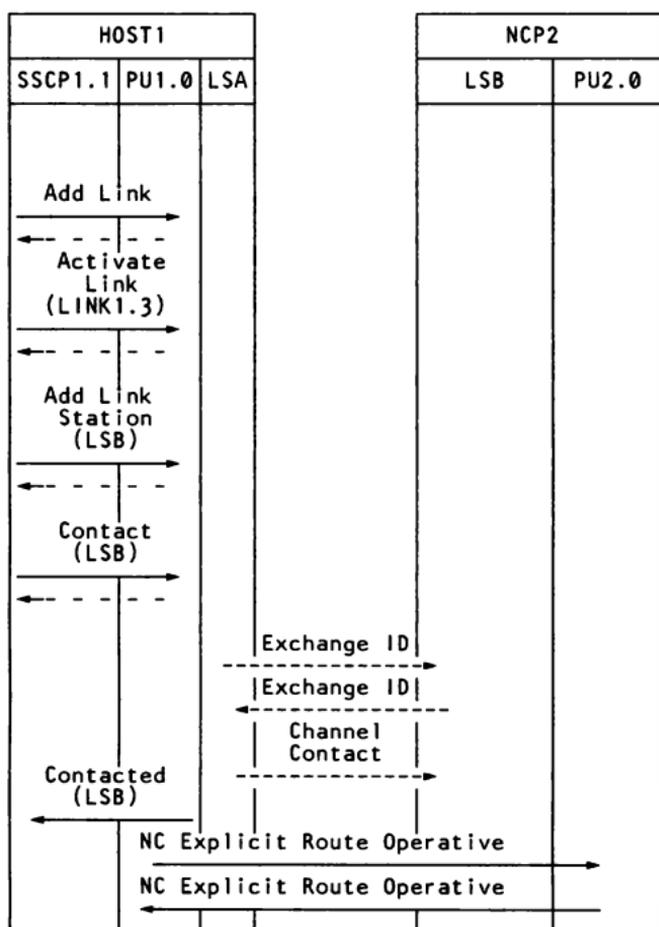
Activating a Host Node, a Channel-Attached Subarea Node, and the Channel Between Them
