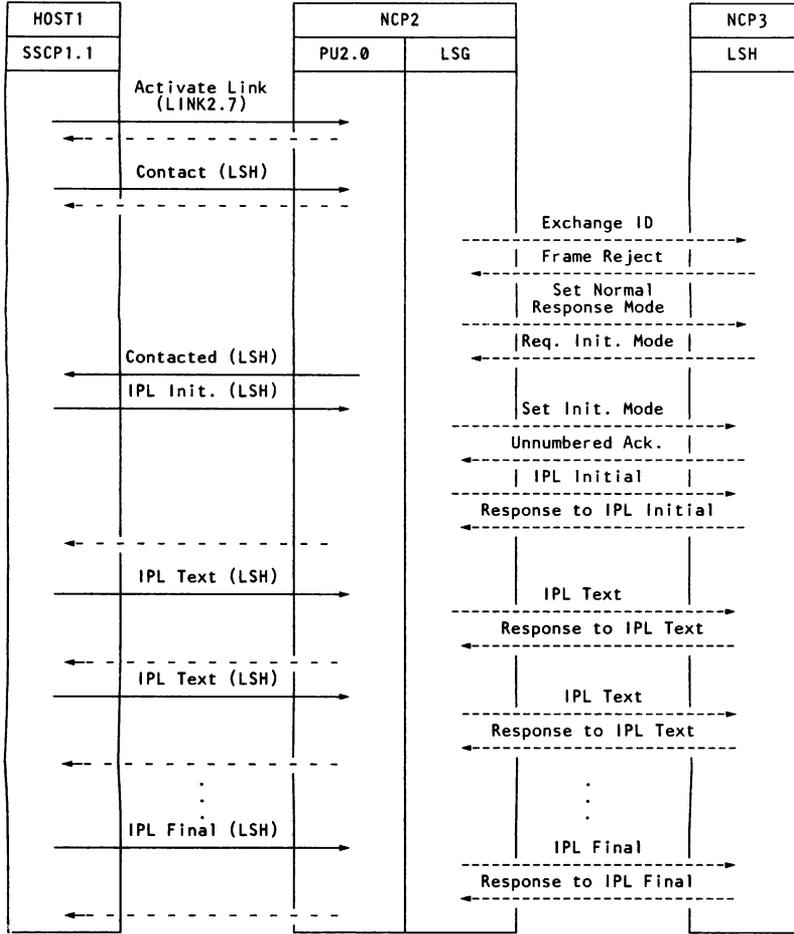
Loading a 3705 Communications Controller with an NCP
