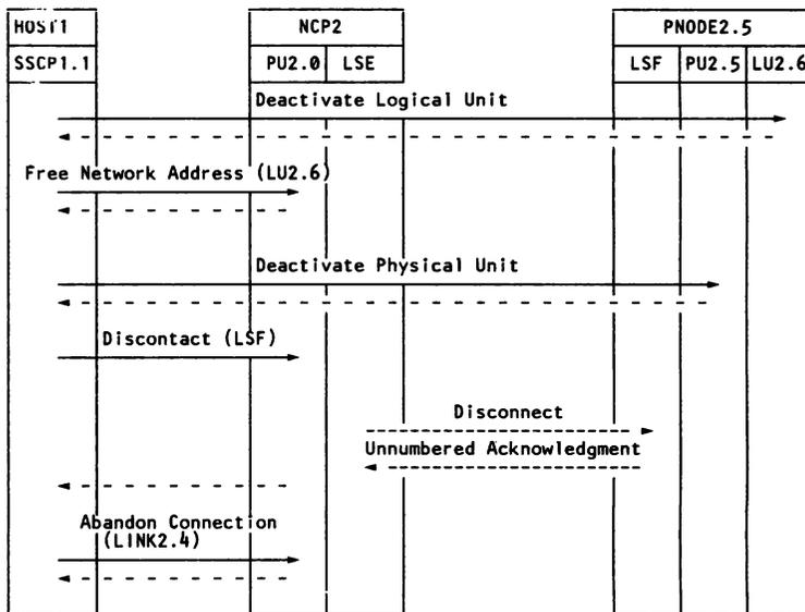
Deactivating a Peripheral Node Attached via a Switched SDLC Link
