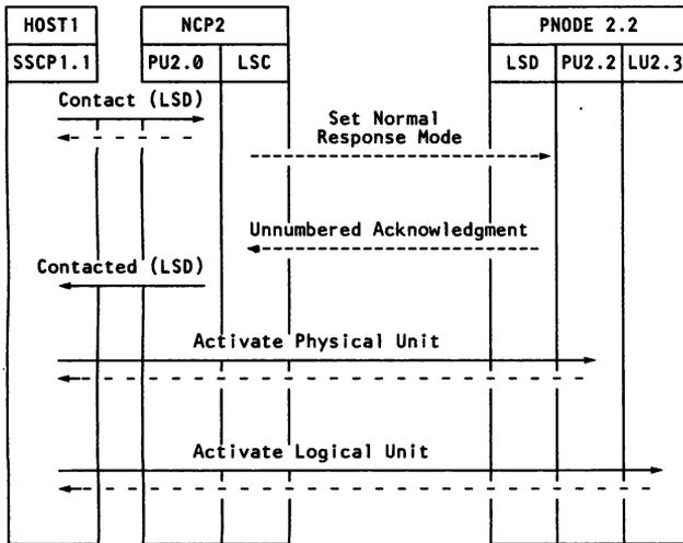
Activating a Peripheral Node Attached via a Nonswitched SDLC Link
