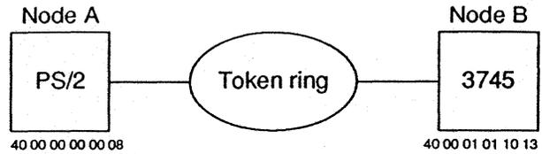
1. The first series of flows show LLC TEST frames sent by the PS/2 (using SAP "04" for SNA path control) to SAP "00" (a null SAP) of the destination address of the 37x5 TIC. This LLC TEST frame is sent as a non-Broadcast frame to locate the 37x5 TIC on the ring. (See page 11 for an explanation of these locally administered addresses.)
