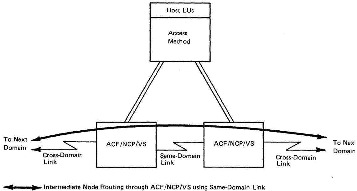
Figure 3-10. Intermediate Node Routing Between Local Communications Controllers in the Same Domain
