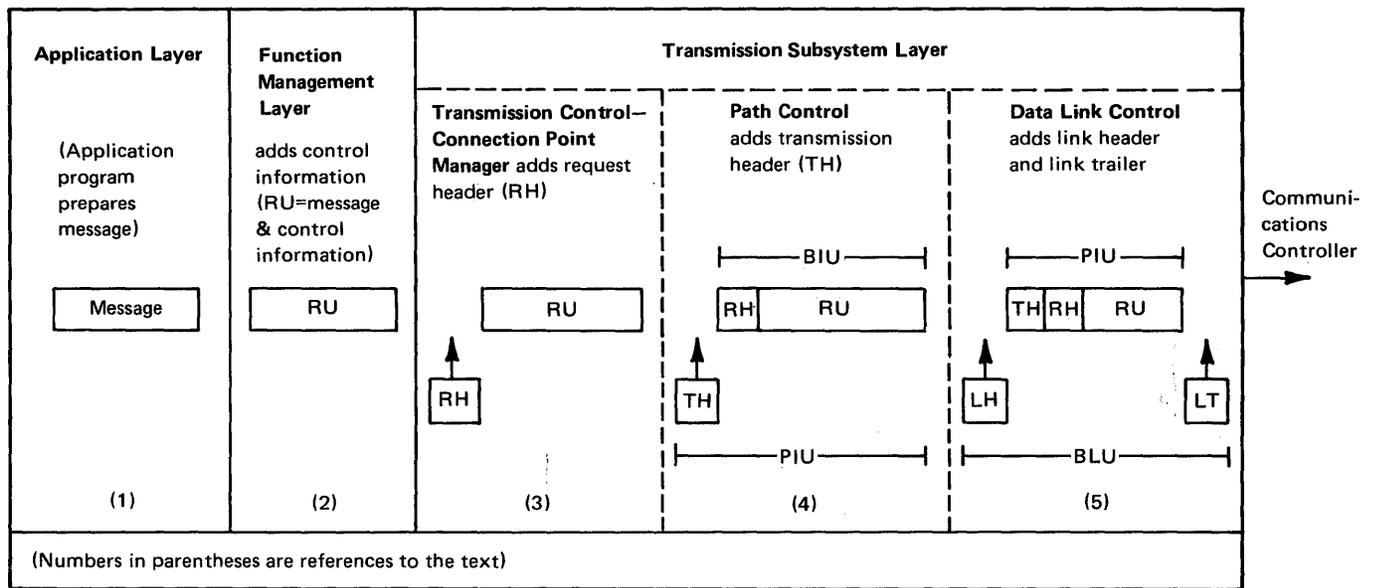
Figure 2-2. Data Flow through Network Layers
