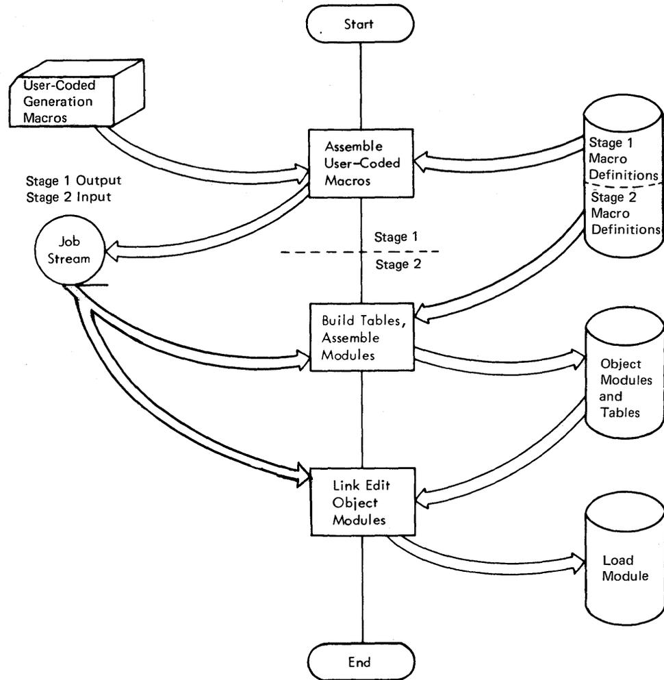
Figure 4-1. Example of the Program Generation Procedure under OS/VS
