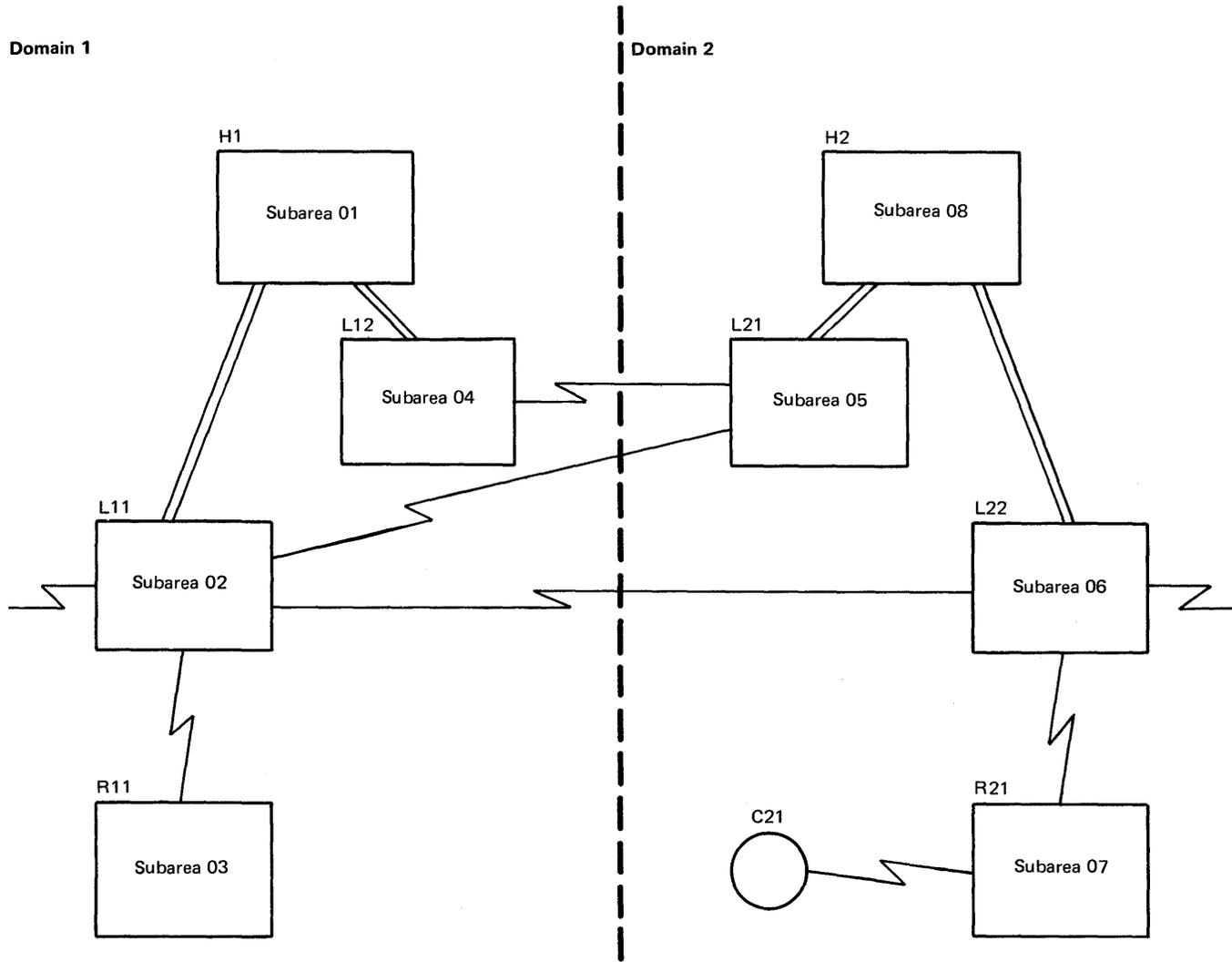
Figure 3-8. Configuration Having Multiple Paths between Domains
