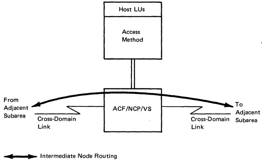
Figure 3-9. Intermediate Node Routing by ACF/NCP/VS
