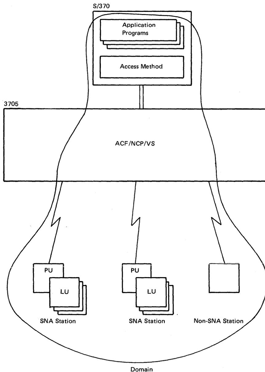
Figure 2-3. ACF/NCP/VS in a Single-Domain Network
