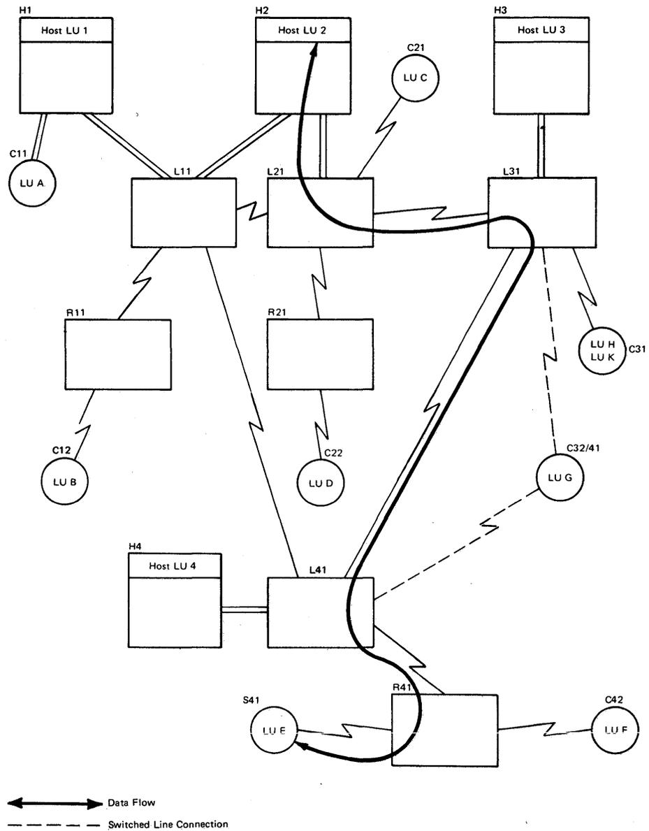
Figure 3-13. Data Flow through an Intervening Domain
