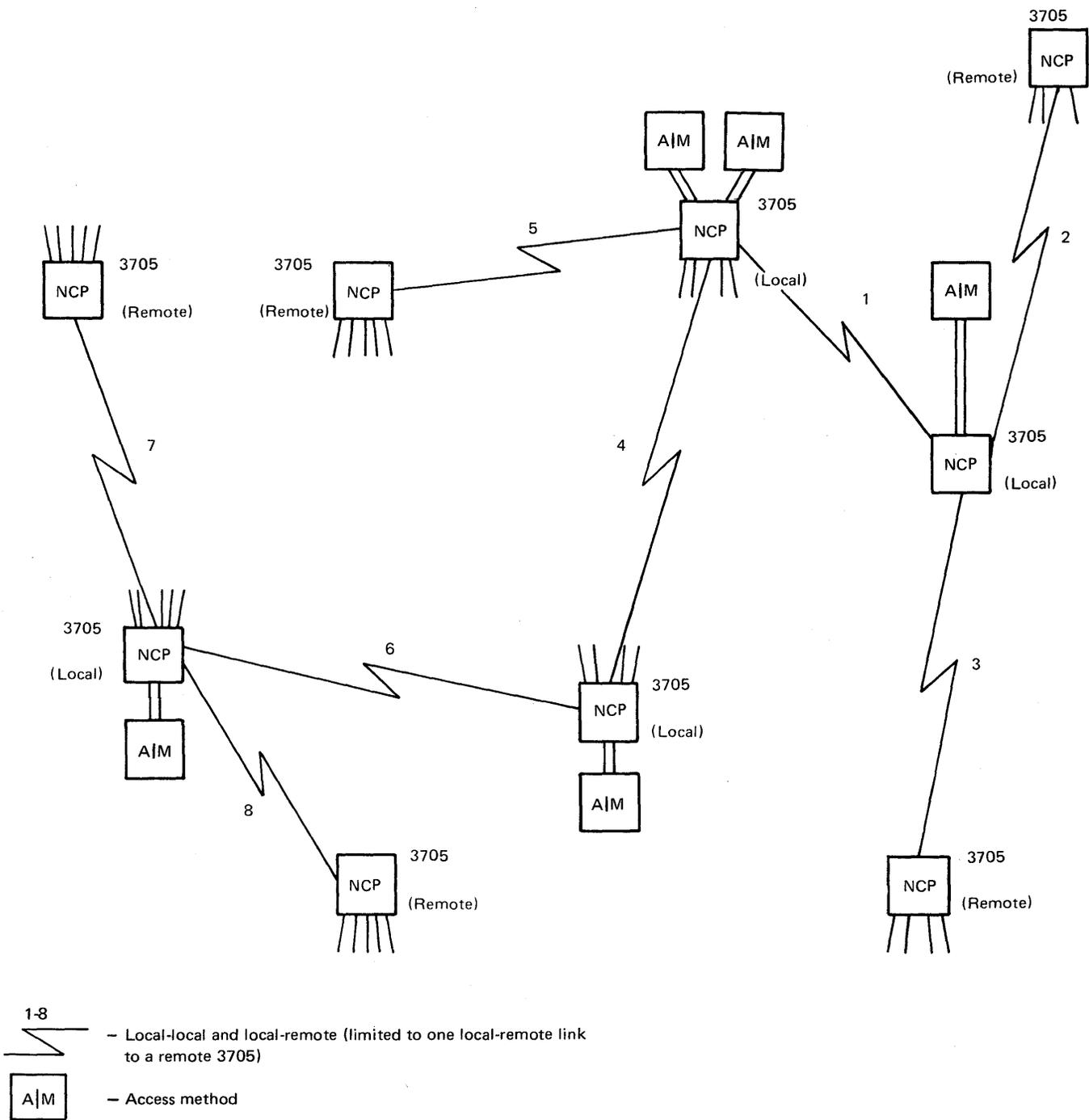
Figure 6-5. Example of a Network Controlled by ACF/NCP/VS Release 2
