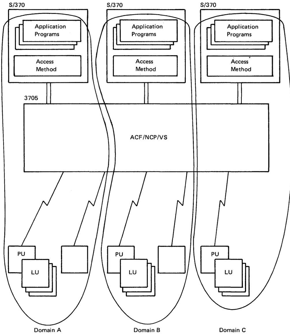
Figure 2-4. ACF/NCP/VS in Multiple Single-Domain Networks
