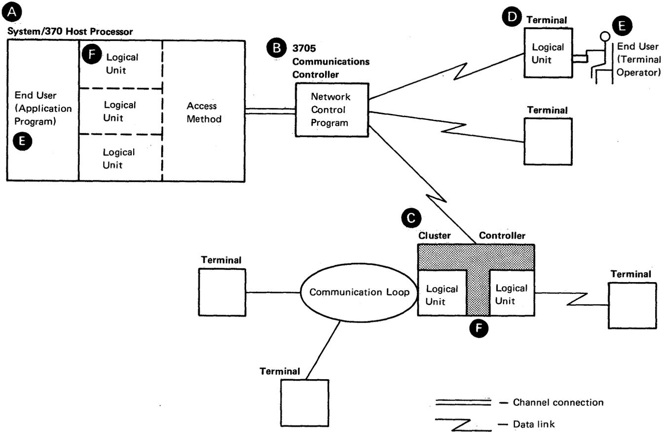
Figure 1-1. Example of a Data Communication Network
