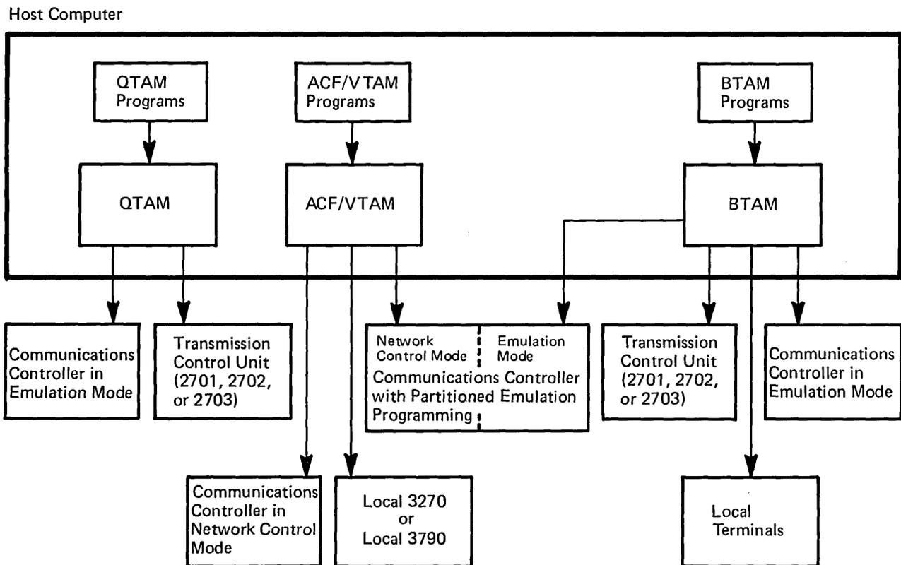
Figure 6-1. ACF/VTAM with Other Telecommunications Access Methods in DOS/VS
