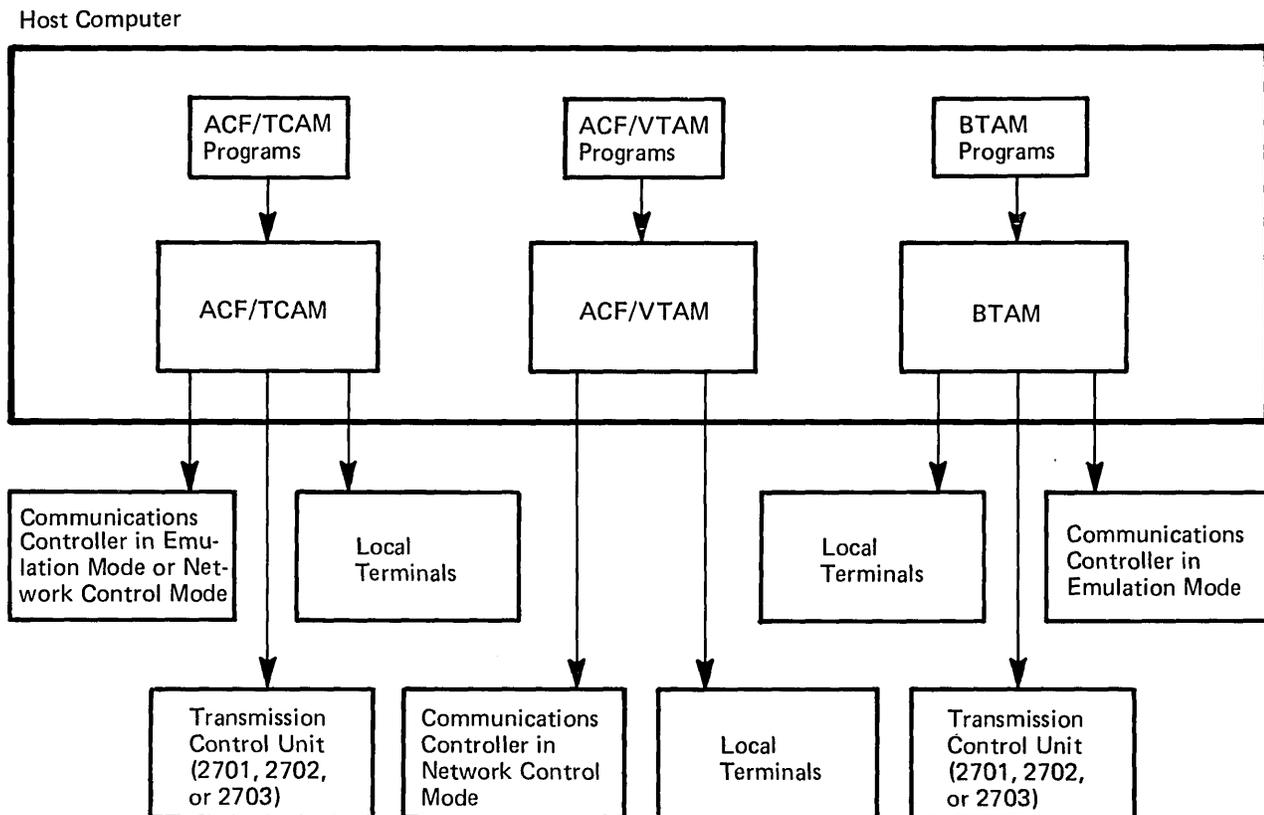
Figure 6-2. ACF/VTAM with Other Telecommunications Access Methods in OS/VS
