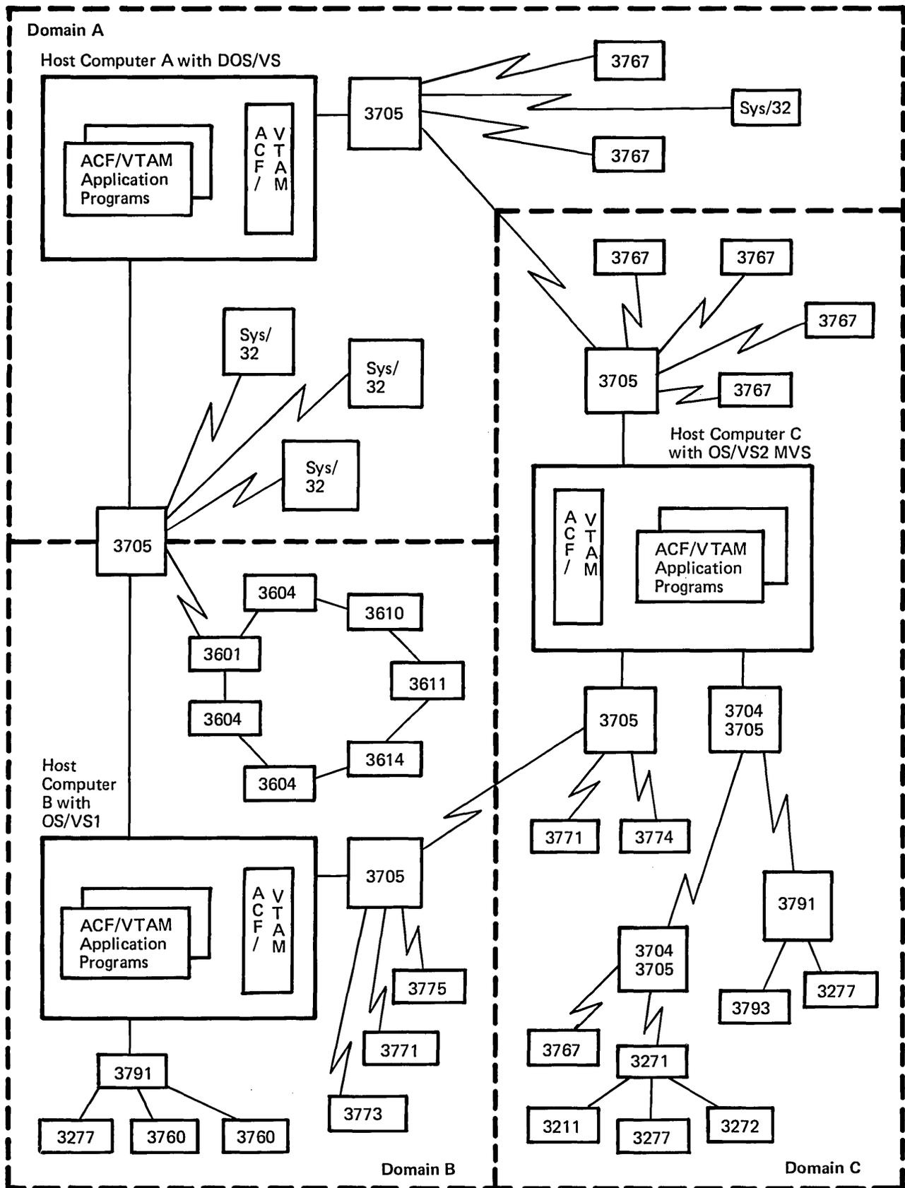
Figure 2-2. A Multiple-Domain ACF/VTAM Network
