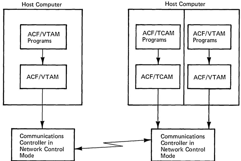
Figure 6-3. ACF/VTAM with Other Telecommunications Access Methods in a Multiple-Domain Network
