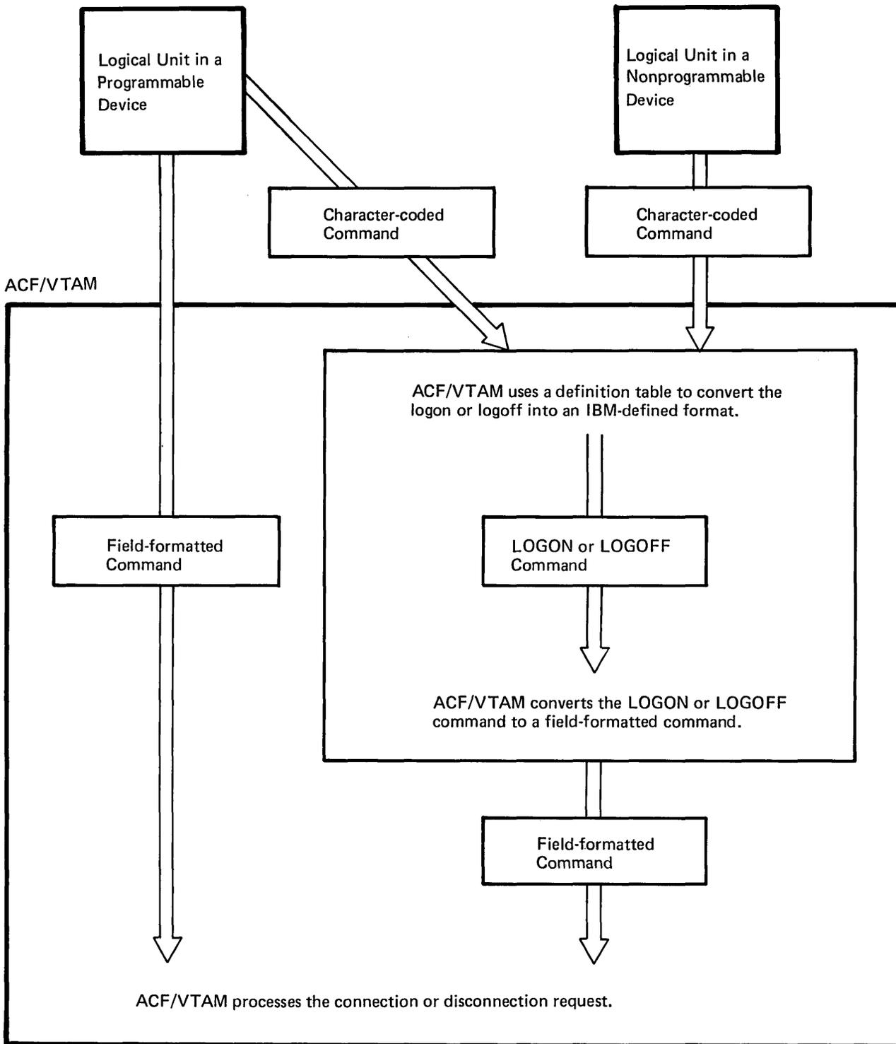
Figure 3-1. Processing Connection and Disconnection Requests from Logical Units
