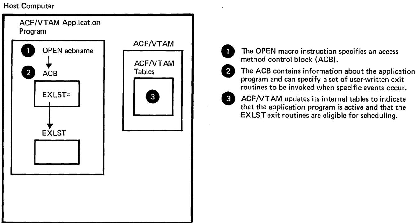
Figure 5-1. Identifying an Application Program to ACF/VTAM
