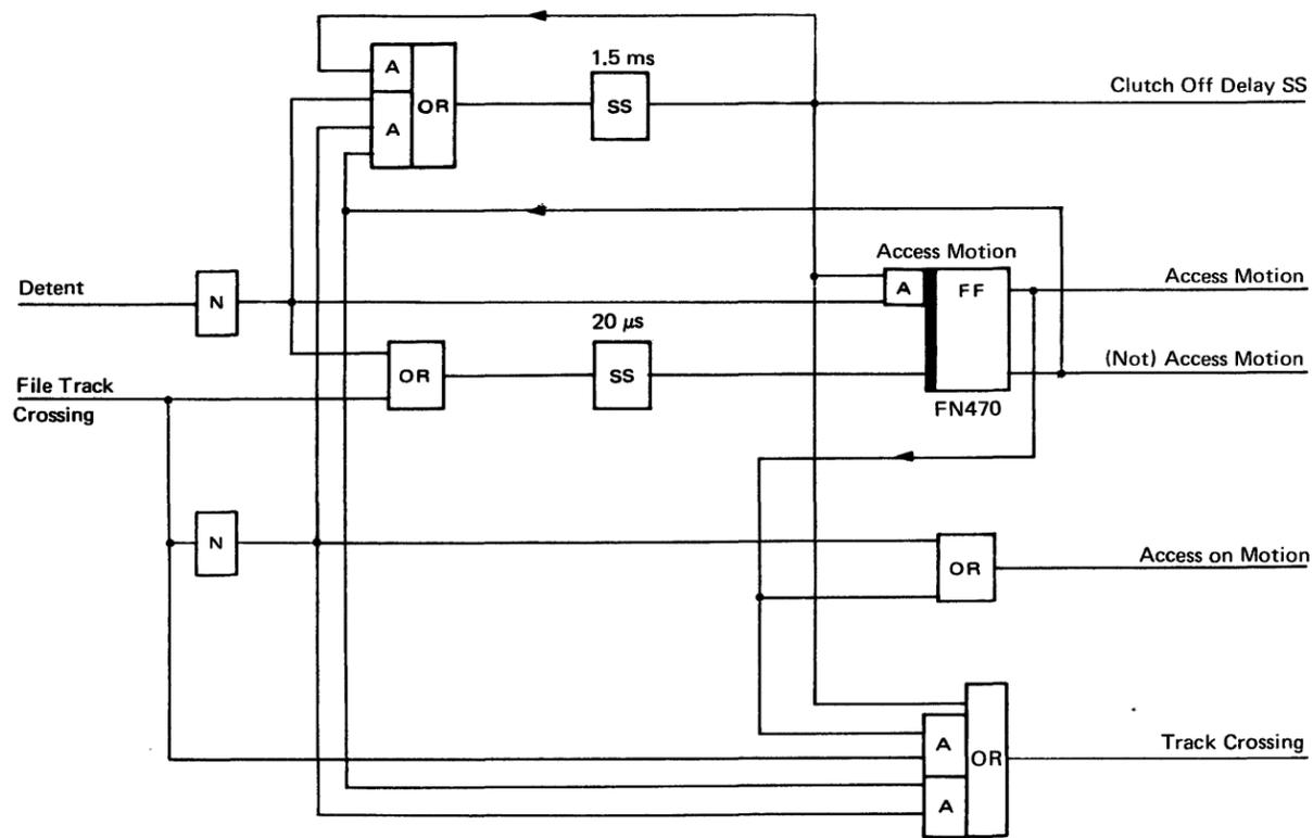
Figure 1-45. Access Control Signals [07506]
