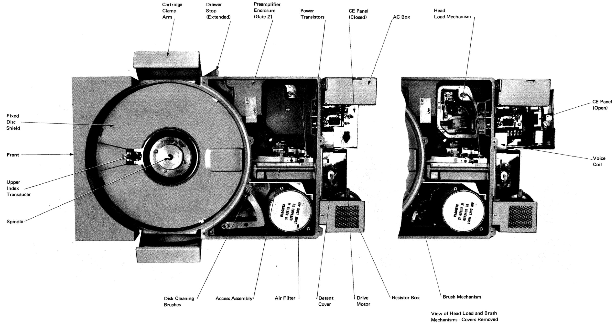
Figure 1-4. Component Layout – Top View [07464]
