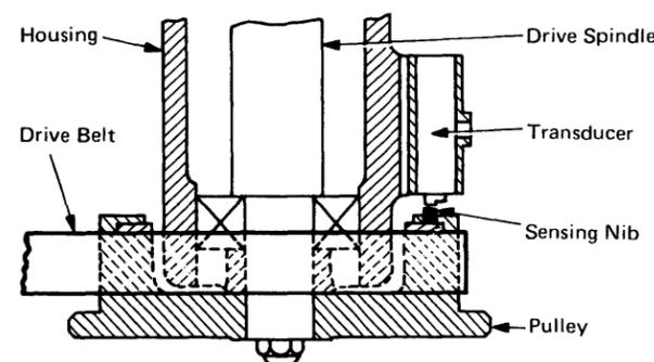
Figure 1-33. Lower Index Transducer [07493]
