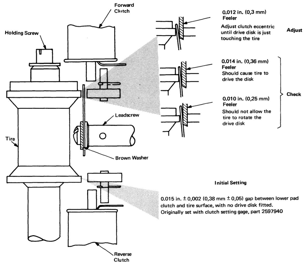
Remove the tire holding screw and withdraw the tire assembly. Take care not to damage the drive disk.
