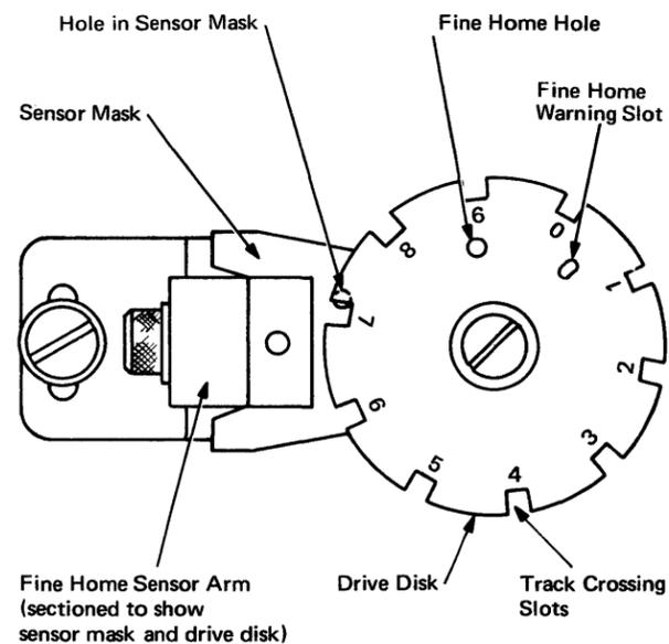
Figure 1-35. Drive Disk and Sensor Mask [07495]
