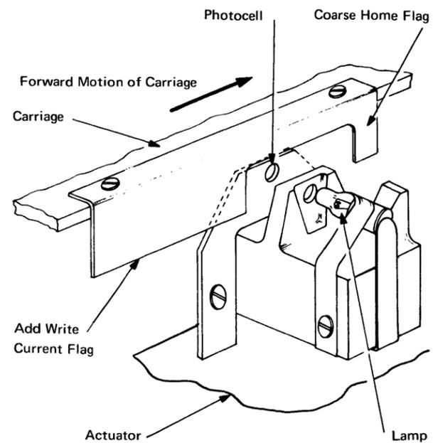
Figure 1-36. Carriage Photocell [07496]
