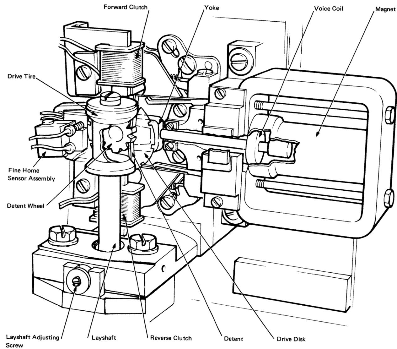
Figure 1-20. Detent Mechanism [07480]
