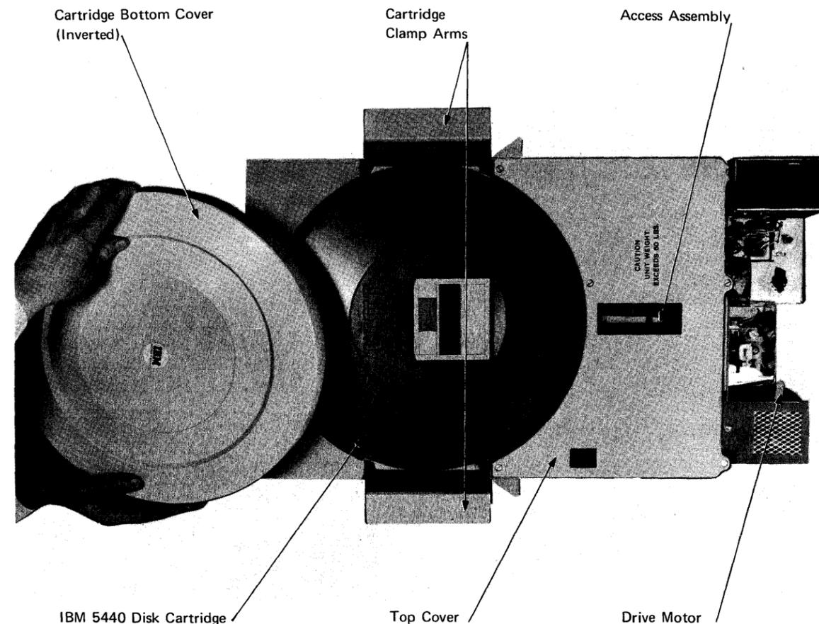
Figure 1-1. IBM 5444 Disk Storage Drive [07461]
