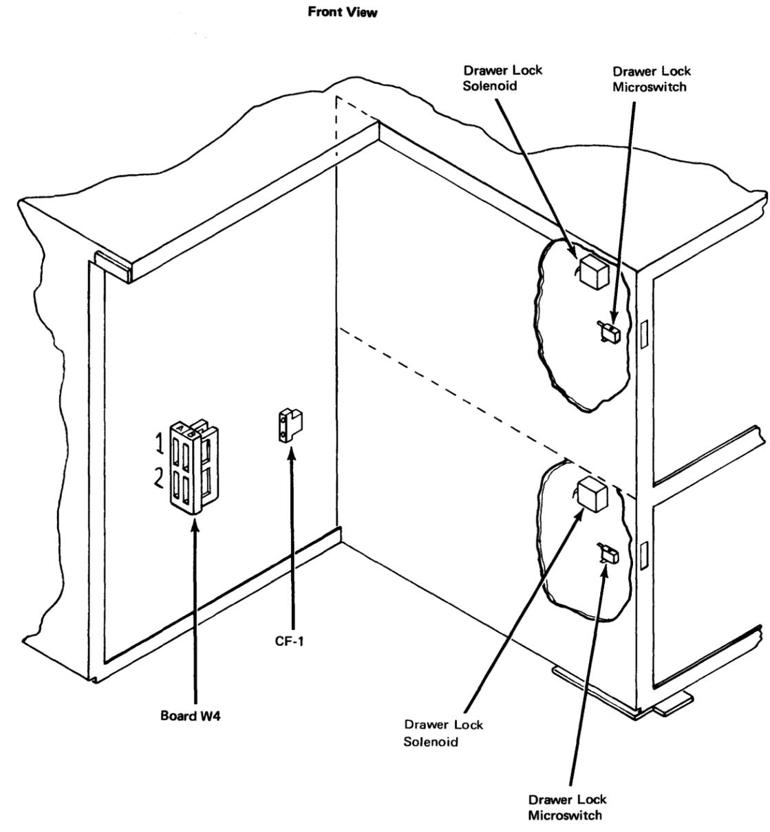
Figure C-3. Disk Enclosure Locations for IBM System/3 [07572]
