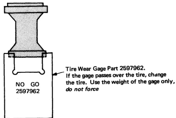
Figure 2-29. Checking Tire Wear [07552]
