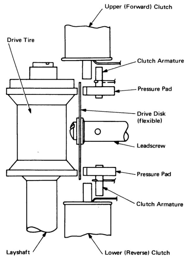
Figure 1-19. Layshaft/Leadscrew Drive [07479]
