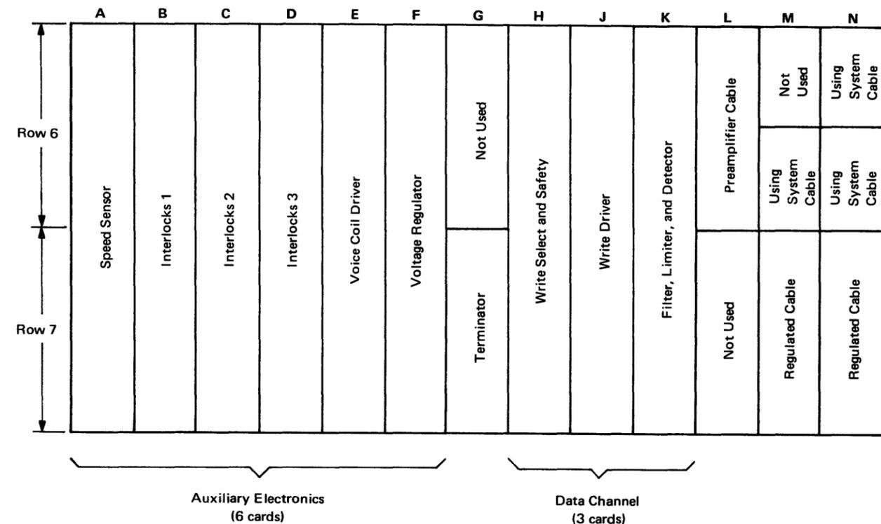
Figure 1-29. Logic Gate Card Layout [07489]
