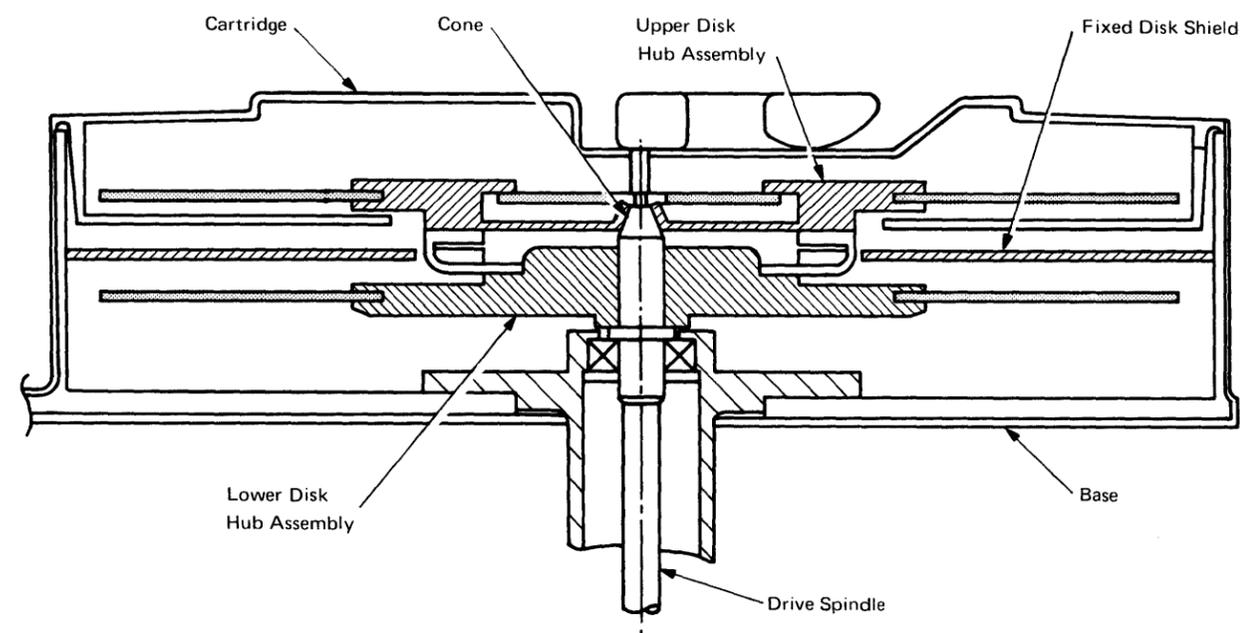
Figure 1-12. Cartridge on Drive Spindle [07472]
