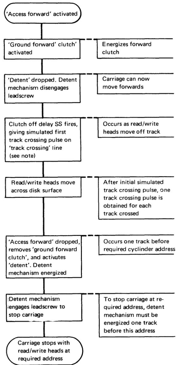
**Note:** The simulated track crossing pulse is an extra pulse which is required because the detent mechanism takes one track to operate; without this extra pulse the carriage would stop at the wrong track.
