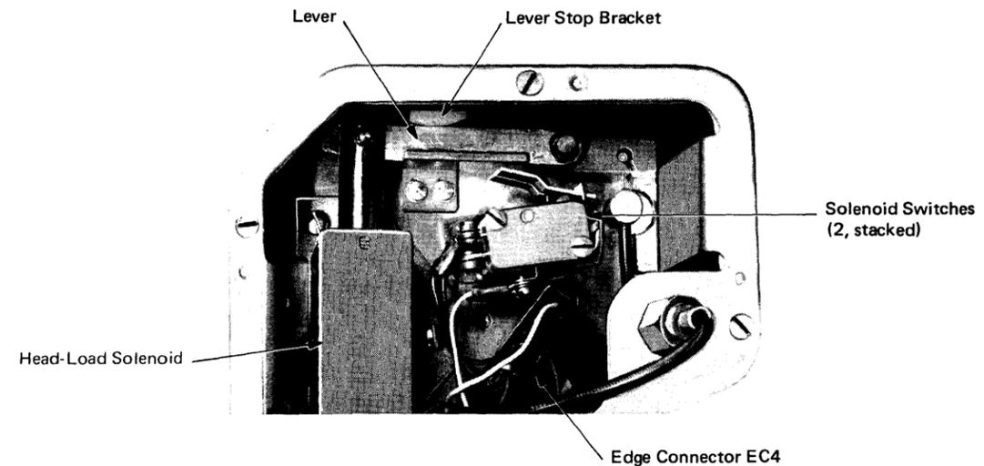
Figure 1-26. Head Load Solenoid Assembly [07486]
