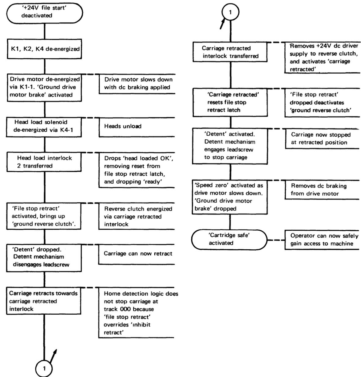
Figure 1-50. Machine Stop Sequence [07511]
