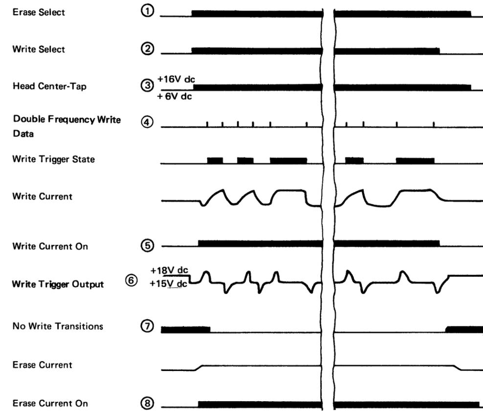
Note: Waveform numbers refer to Write Circuit Logic (Figure 1-58)
