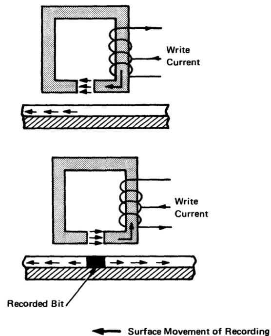
Figure 1-55. Horizontal Recording [07516]
