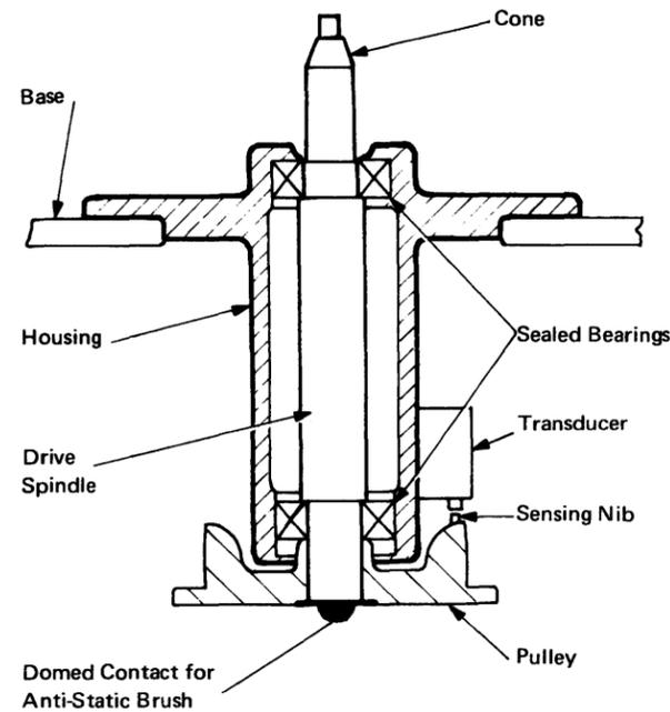
Figure 1-8. Drive Spindle [07468]
