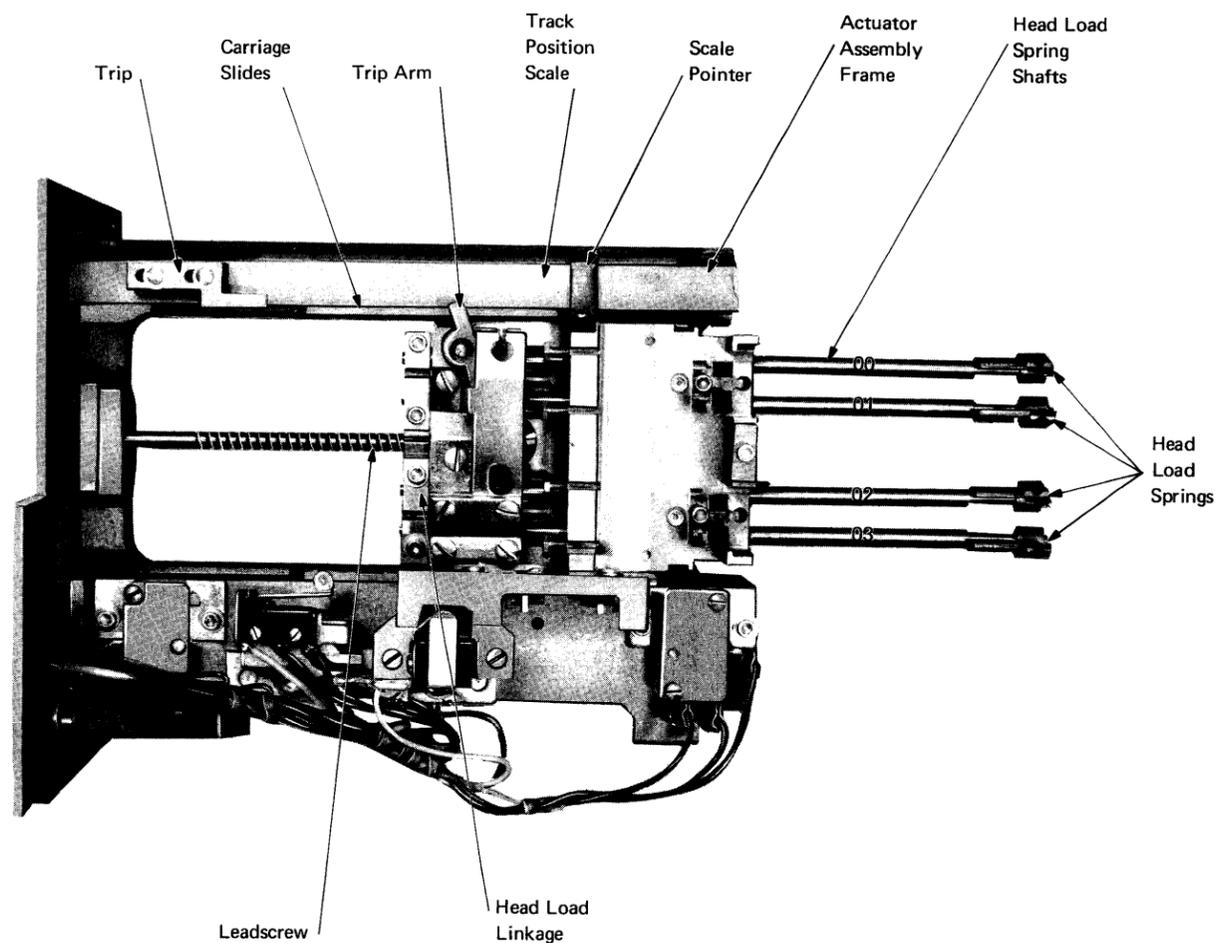
Figure 1-17. Carriage and Actuator Assembly – Without Heads [07477]
