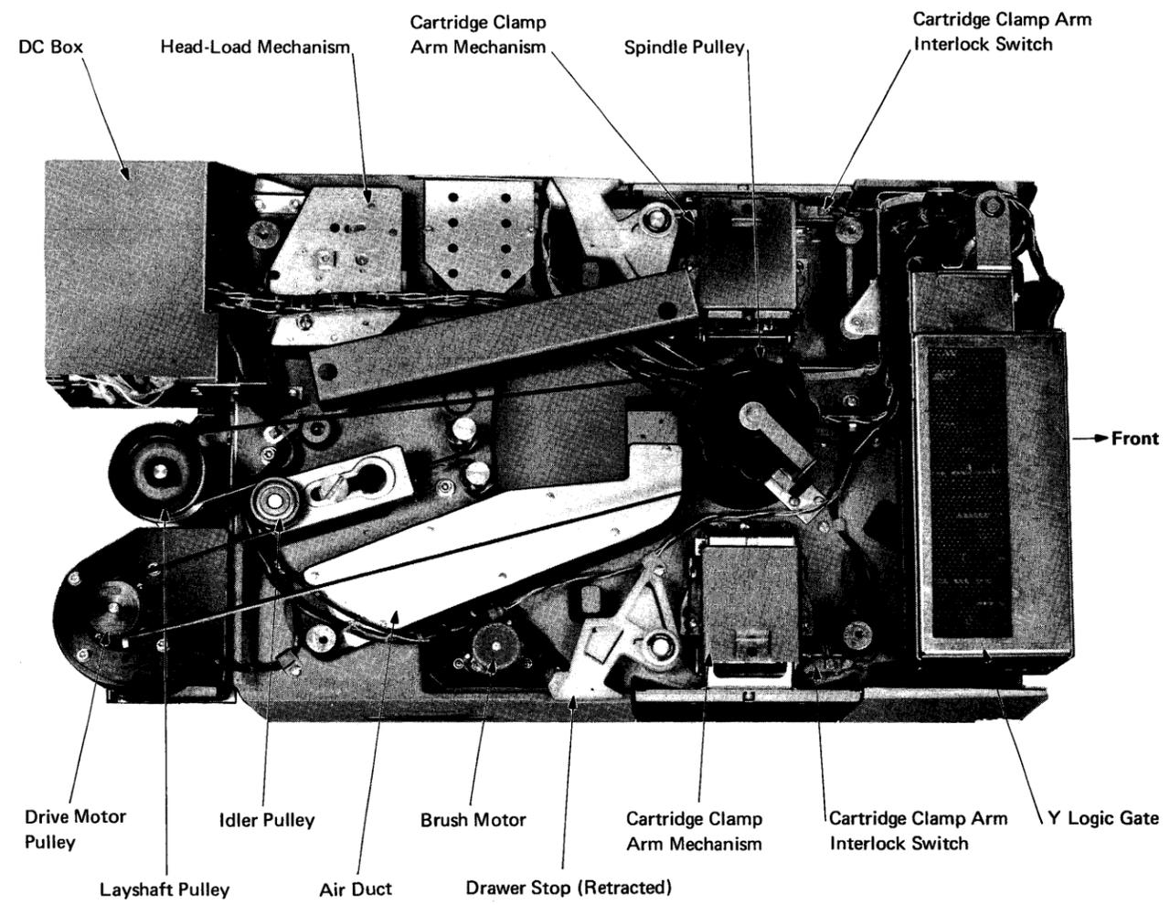
Figure 2-48. Underside View of 5444 - Locations [07568]
