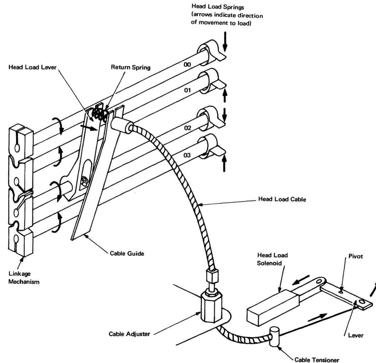
Figure 1-24. Head Load Linkage [07484]
