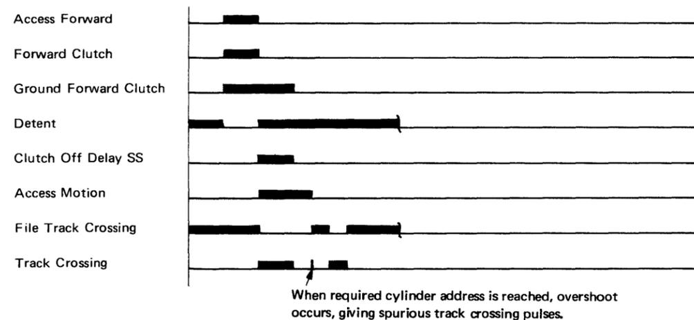
Figure 1-43. Head Forward Operation – Timing [07504]
