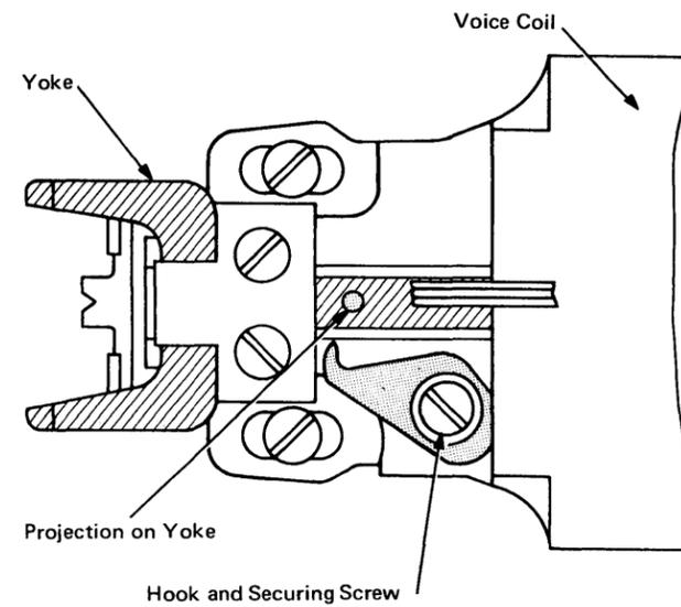
Figure 2-6. Yoke Holdout Hook [07531]
