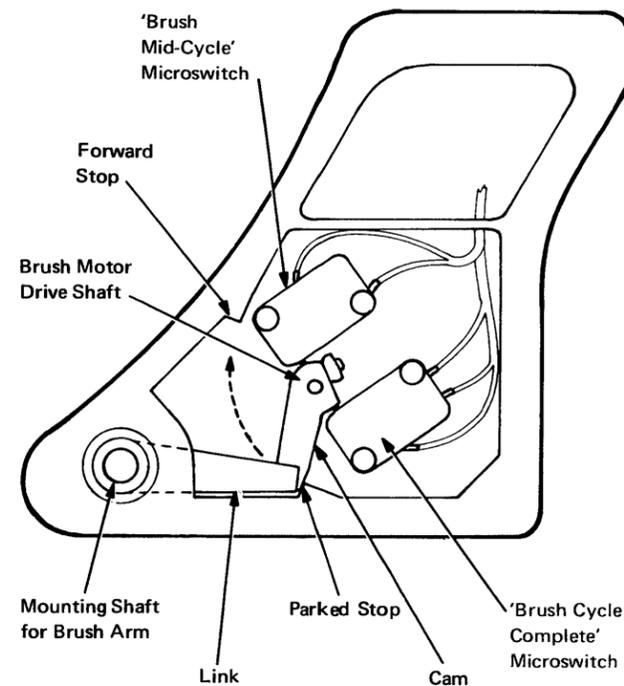
Figure 1-15. Disk Cleaning Brushes Linkage Mechanism [07475]
