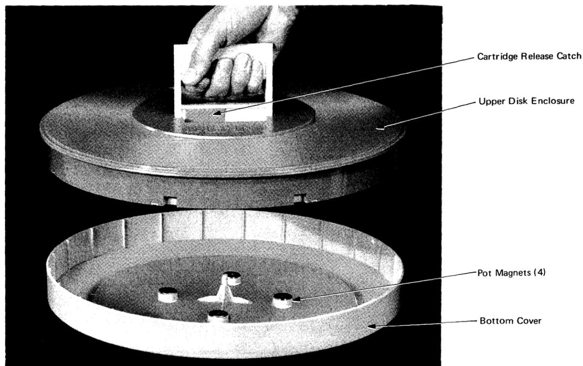
Figure 1-13. Cartridge Handle and Release Catch [07473]
