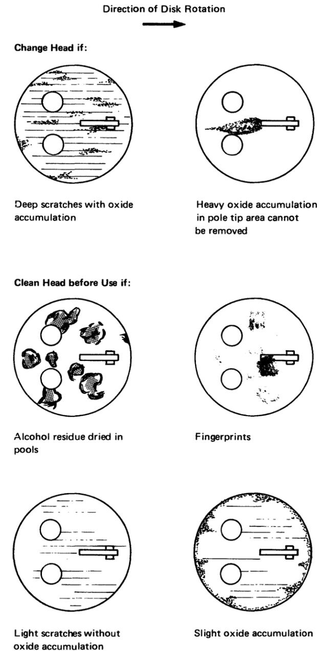
Figure 2-11. Conditions of Read/Write Heads [07536]
