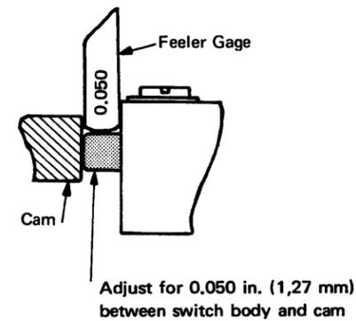
**Figure 2-24. Disk Cleaning Brush Drive – Switch Adjustment [07548]**
