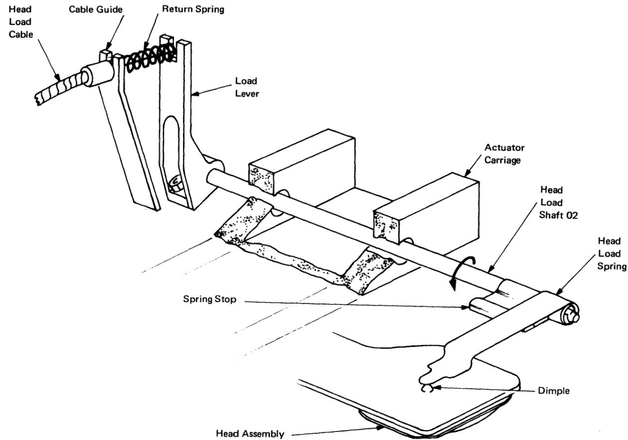
Figure 1-25. Head Load Shaft Operation [07485]
