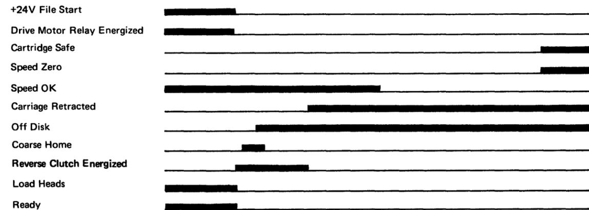
Figure 1-52. Machine Stop Timing [07513]
