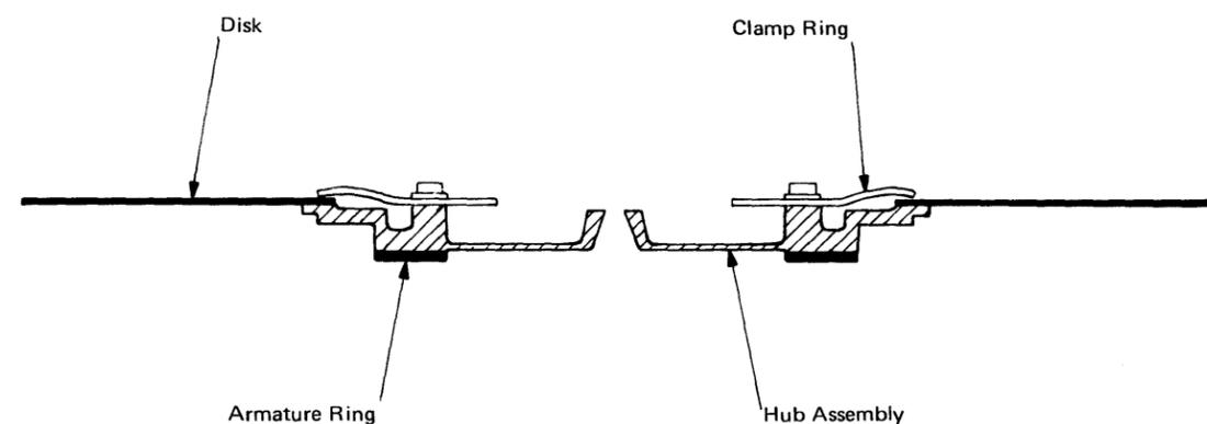
Figure 1-11. Upper Disk Hub Assembly [07471]
