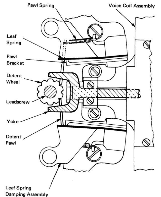
Note: Drive tire, drive disk, and clutches omitted for clarity
