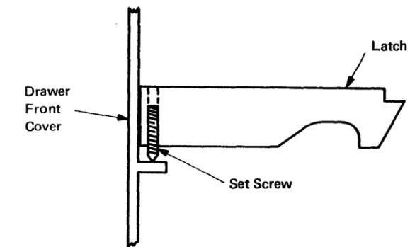
Figure C-2. Drawer Latch Adjustment [07571]
