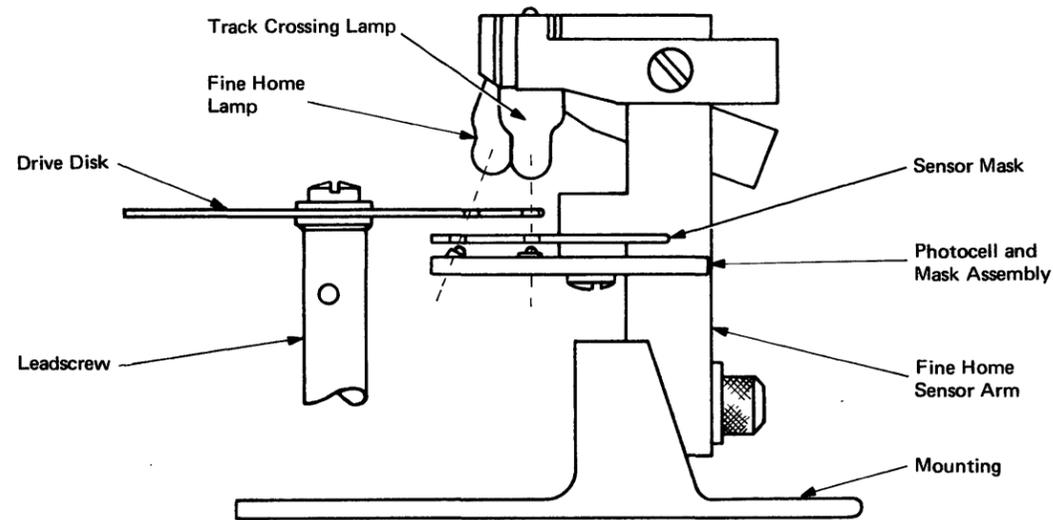
Figure 1-34. Track Crossing Sensor/Fine Home Sensor [07494]
