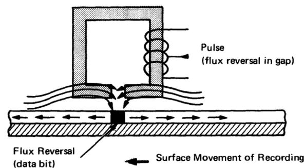
Figure 1-56. Horizontal Reading [07517]
