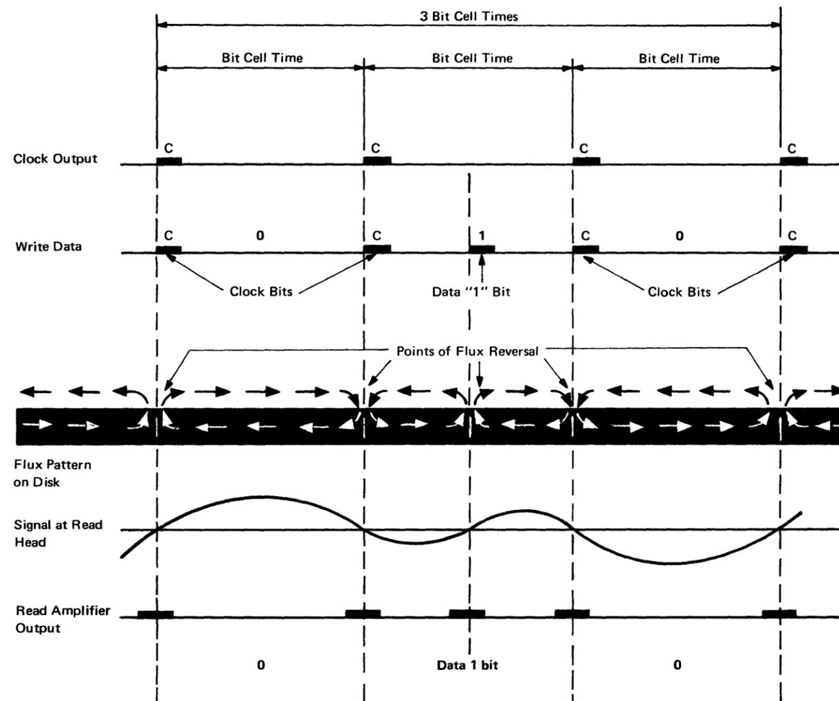
Figure 1-57. Double Frequency Recording - Flux and Pulse Relationship [07518]
