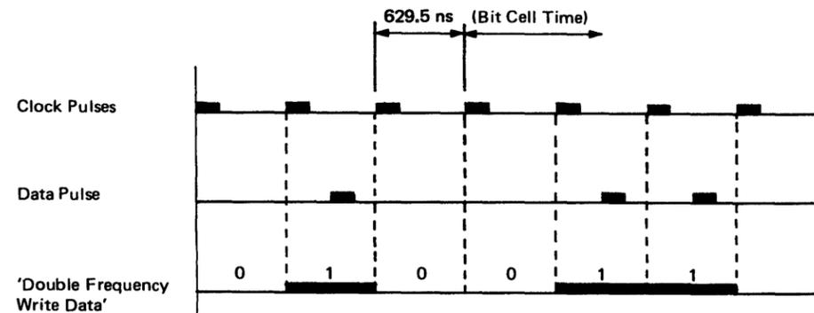
Figure 1-53. Derivation of Composite Write Signal [07514]
