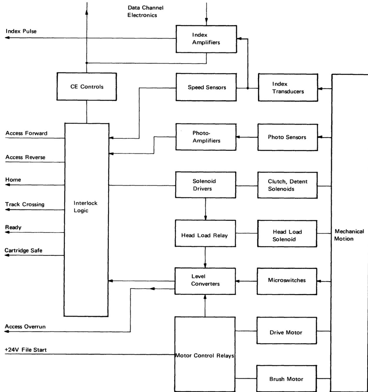
Figure 1-30. Auxiliary Electronics [07490]
