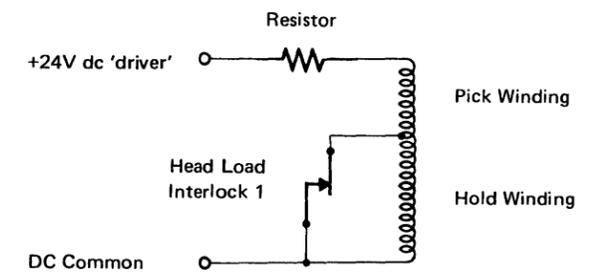
Figure 1-27. Head Load Solenoid Circuit [07487]
