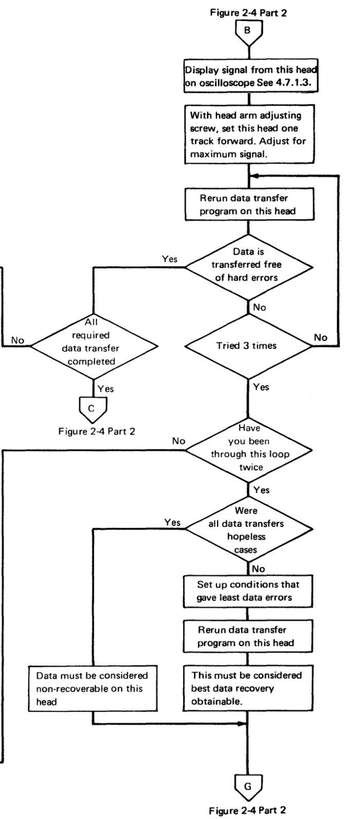
Figure 2-4. Error Recovery Procedure – R/W Head 2 or 3 Replacement (Part 1 of 2) [07501]
