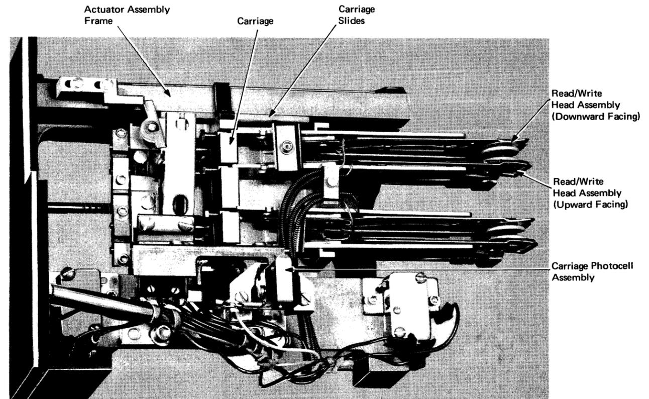
Figure 1-16. Actuator Assembly [07476]
