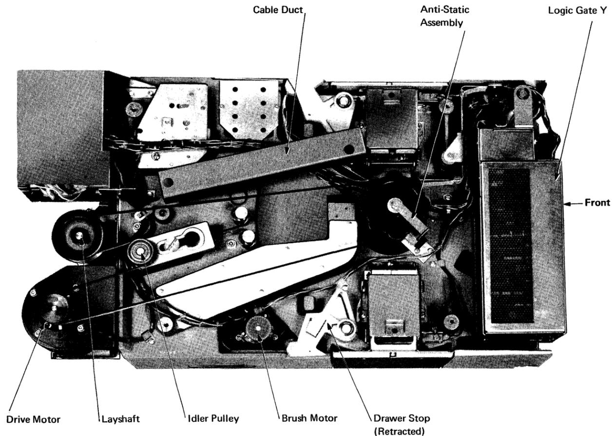
Figure 1-5. Component Layout - Underside View [07465]
