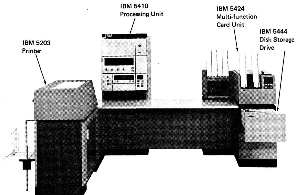
Figure 4-1. IBM System/3 Disk System
