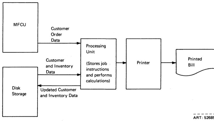
Figure 1-2. Input, Processing, and Output Functions
