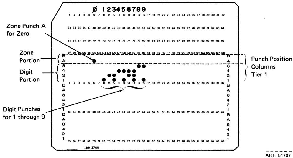
Figure B-2. Numeric Punches in a Card
