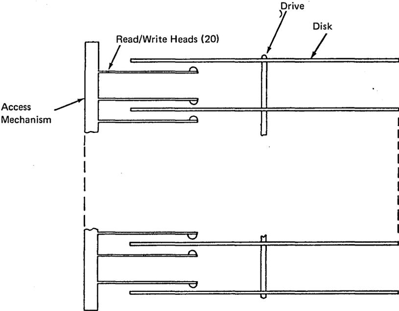
Figure 31. IBM 5445 Disk Storage Drive
