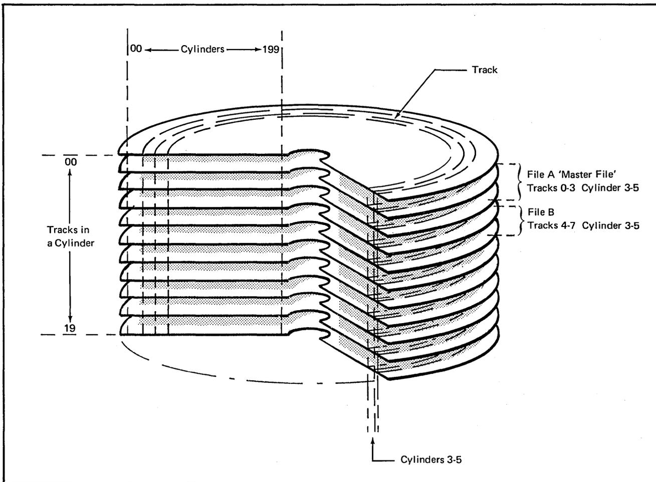
Figure 32. Cylinder Concept on the IBM 5445
