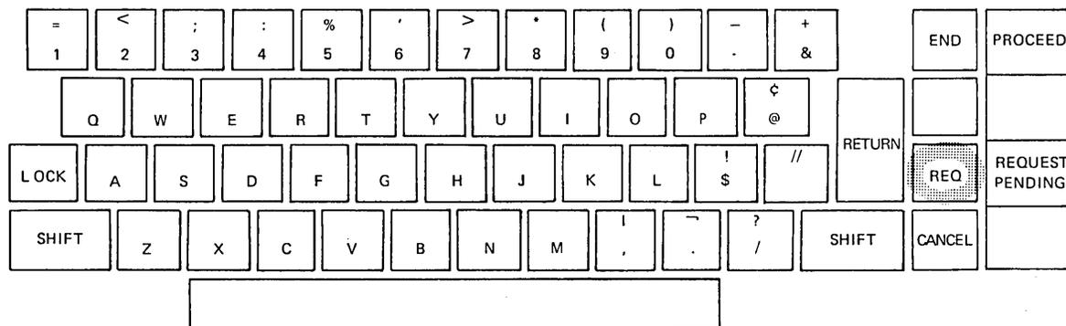
Figure 10. Keyboard Format of the 5471 Printer-KeyBoard
