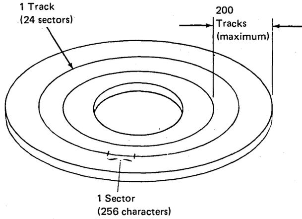
Corresponding tracks from both surfaces of one disk form a cylinder. These two corresponding tracks can be accessed in a single position of the read/write heads.
