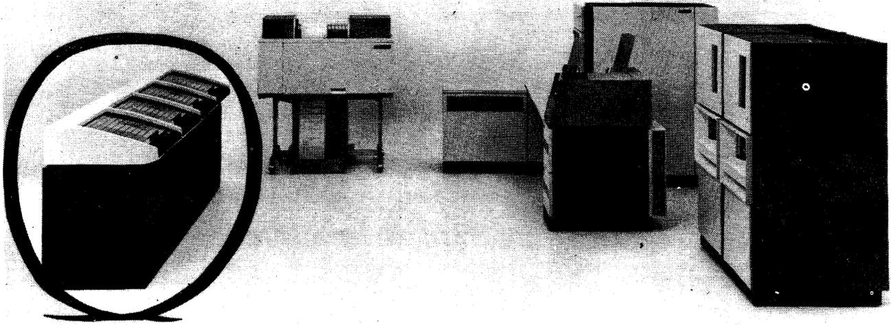
The 3410/3411 Models 1, 2, and 3 tape subsystems read and write half-inch magnetic tape. The IBM 3410 Magnetic Tape Unit is a tape unit only; the IBM 3411 Magnetic Tape Unit and Control is a tape unit and a control unit in the same frame.
