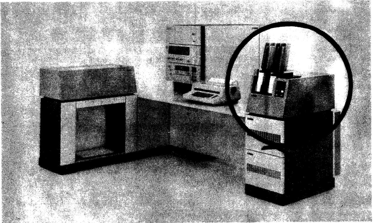
Figure 4-1. IBM 5424 Multi-Function Card Unit
