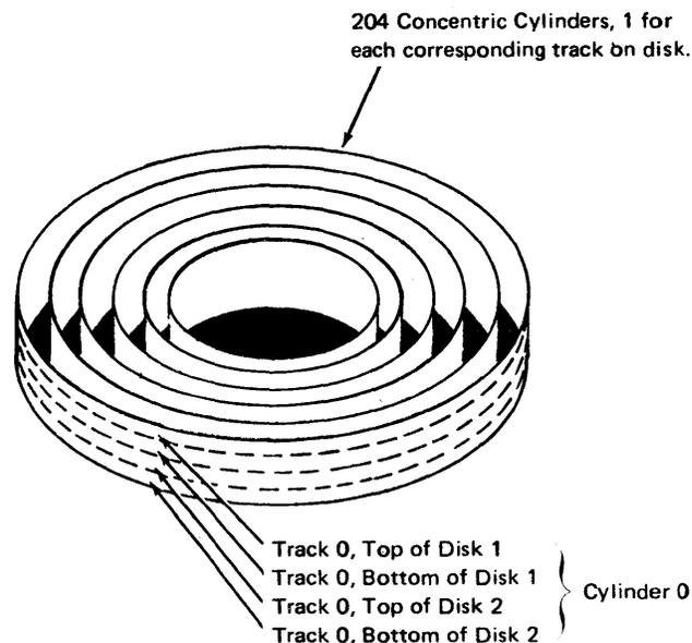
**Note:** The same cylinder address is used for all corresponding tracks on the disks. For example, track 15 on both top and bottom of disks 1 and 2 are all considered to be bands of data on one cylinder, so all four bands have the same cylinder address. On the 5444, the same track on both the upper and lower surfaces of a single disk are considered to be a cylinder, and are on either the removable disk or the non-removable disk.
