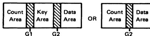
Records, consecutively numbered from record zero (R<sub>0</sub>) upward, fill the track from the home address to the end of the track (detected by encountering the index marker).
