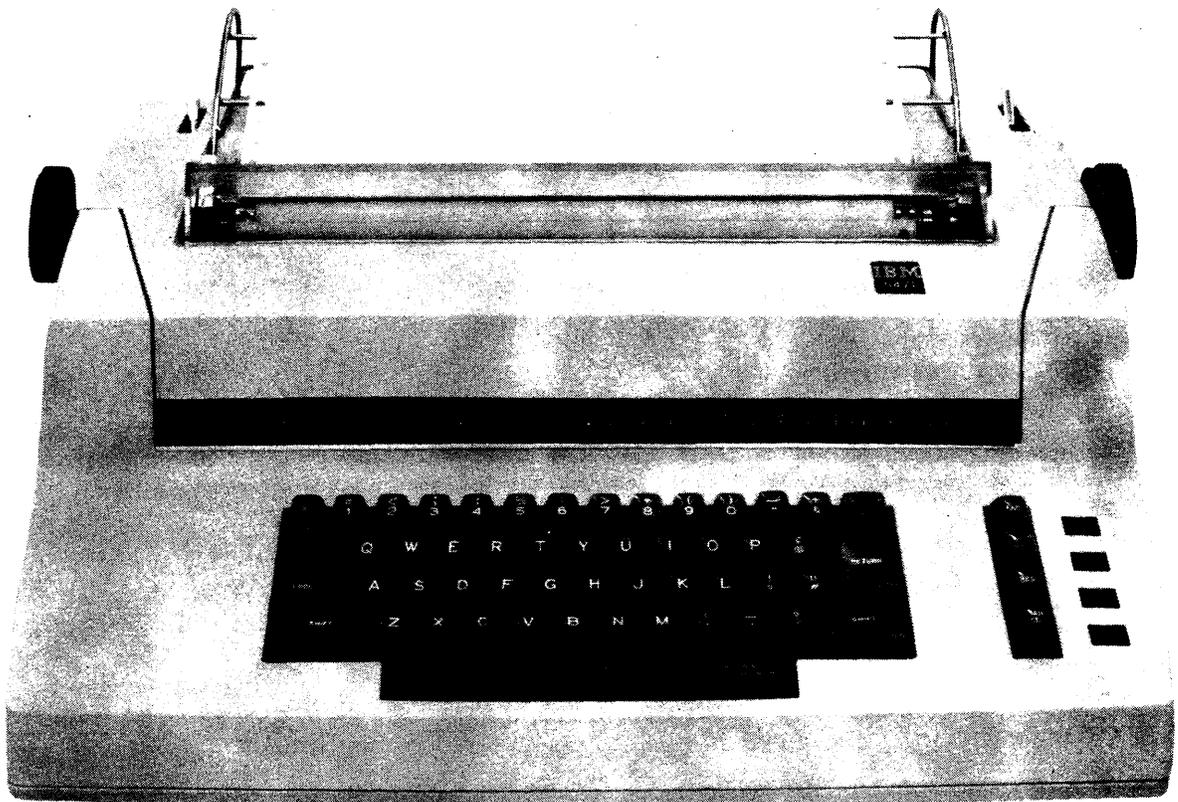
Figure 8-1. IBM 5471 Printer-Keyboard
