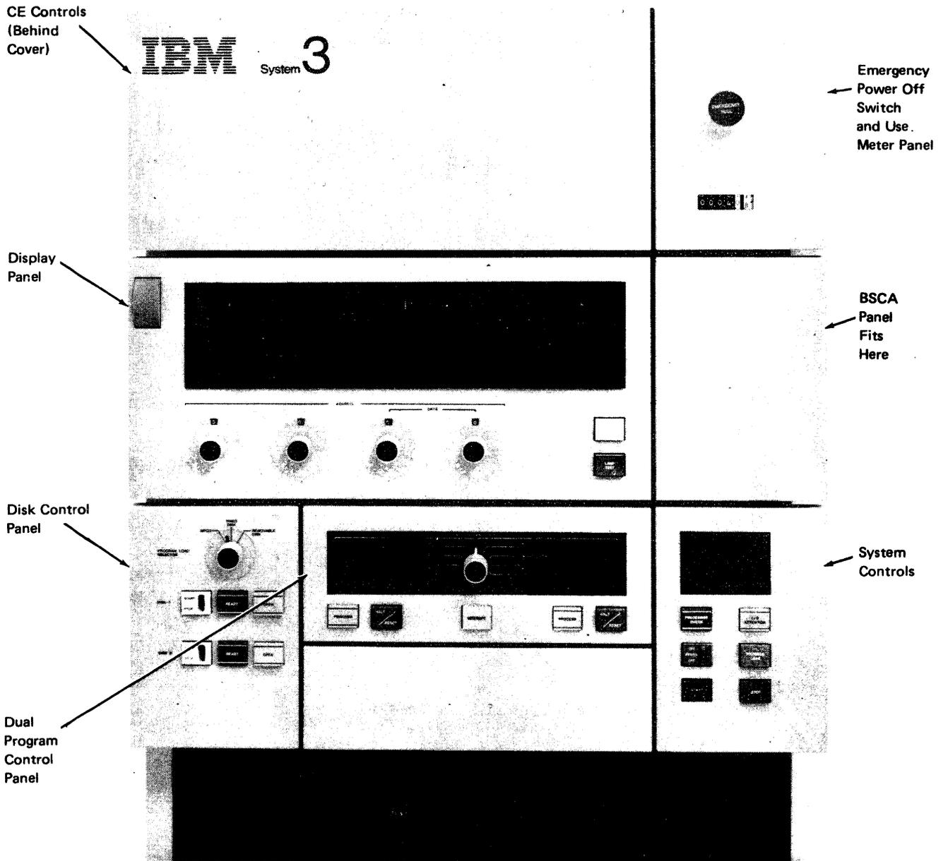
Figure 3-1. System Control Panel
