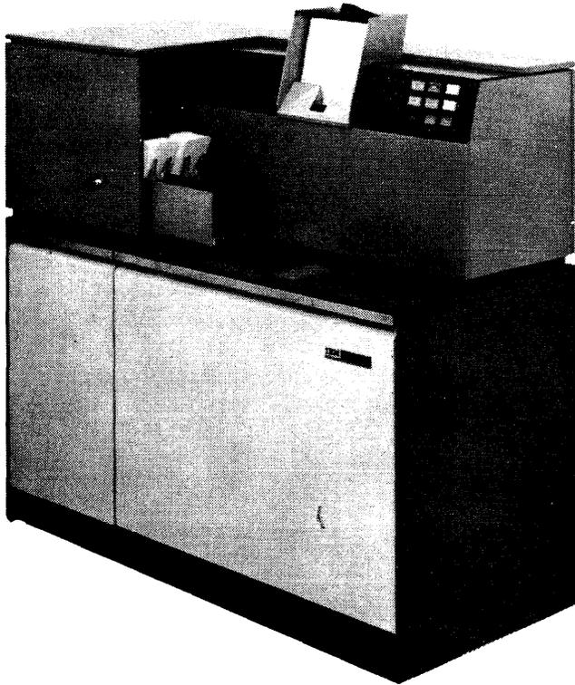
Figure 14-1. IBM 1442 Card Read Punch
