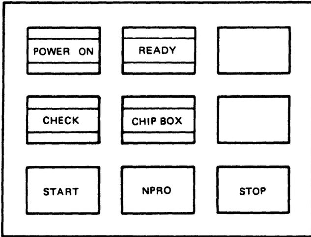
Figure 14-3. 1442 Operator's Panel
