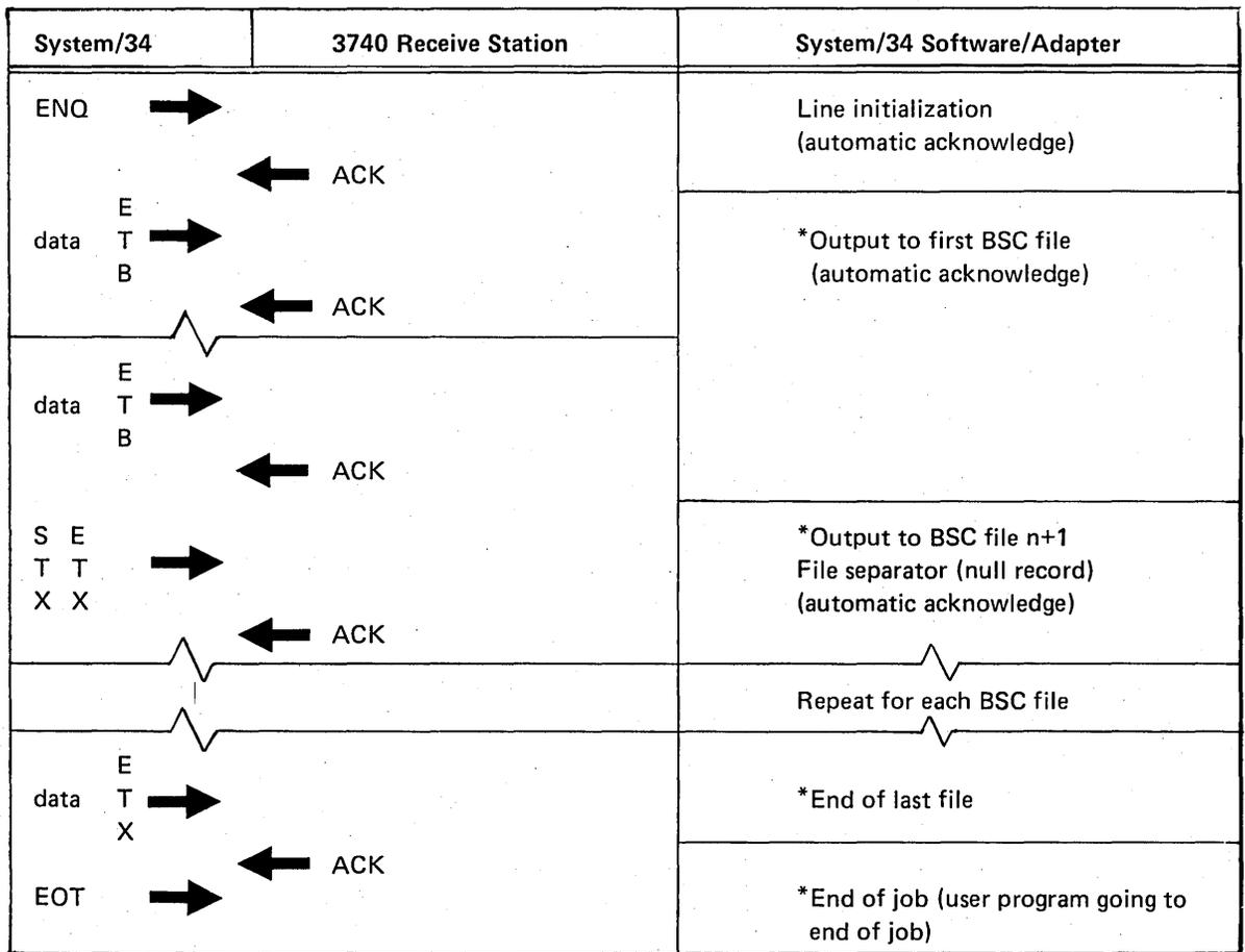
**System/34 Receives Multiple Files from and Transmits Multiple Files to 3740**
