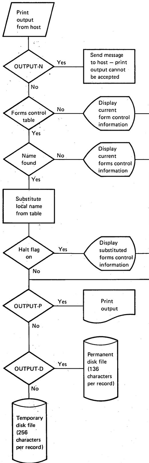
Figure 7-3. Print Output Processing by SRJE
