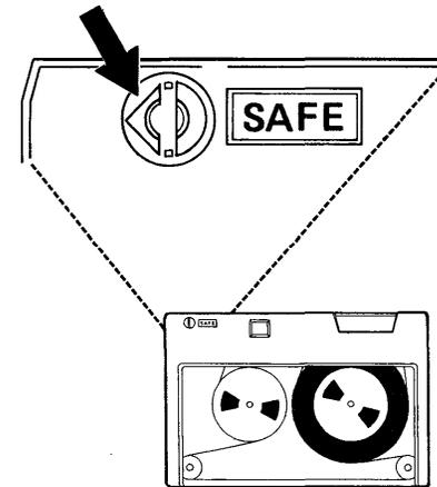
The notch on the write-protect plug should be turned away from the SAFE position.
