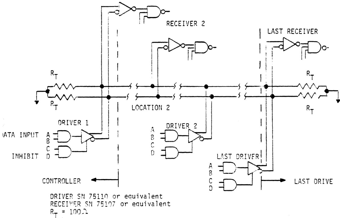
Note: Decoupling capacitors (0.1  $\mu$ f typical) are required on +5V and -5V power supply pins for each driver or receiver chip.
