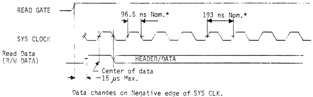
\* Based on Spindle Speed of 3600 RPM
