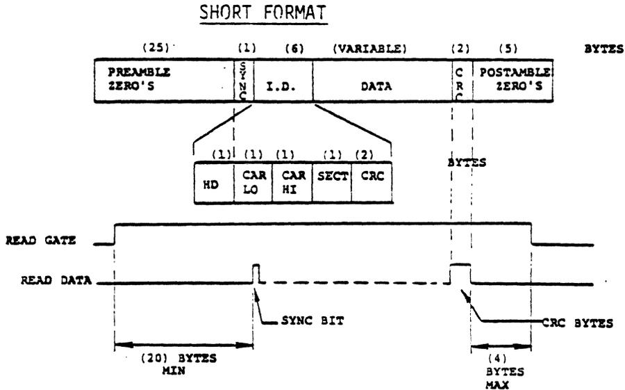
Note: I.D. may be expanded by any number of bytes to suit the user. It may include flag bits to indicate write protect and/or defective sector. Sync Byte is 01 Hex. Read Gate must drop 1 byte before end of Postamble.
