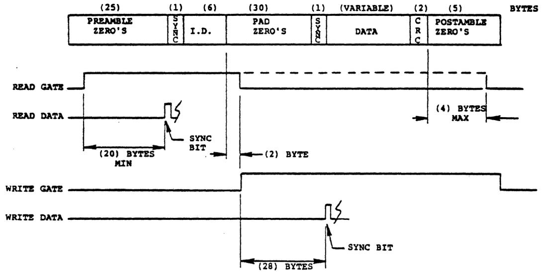
Note: I.D. may be expanded by any number of bytes to suit the user. It may include flag bits to indicate write protect and/or defective sector. Sync Bytes are 01 Hex. Read Gate must drop 1 byte before end of Postamble.
