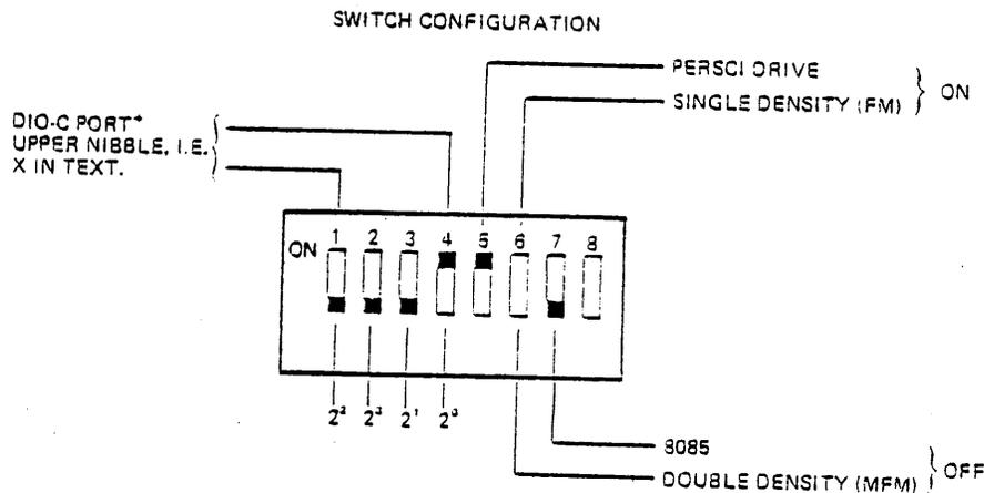
\*NOTE: Binary values of this switch do not follow normal 3, 2, 1, 0 weighting. Weighting is actually 2, 3, 1, 0 as shown in the above example. Also the ON position is a binary 0 and the OFF position is a binary 1. Thus for port set to D in the above example, switch 3 on the DIP switch would be set on and switch 4 would be off. In the example above the switch is set to E.
