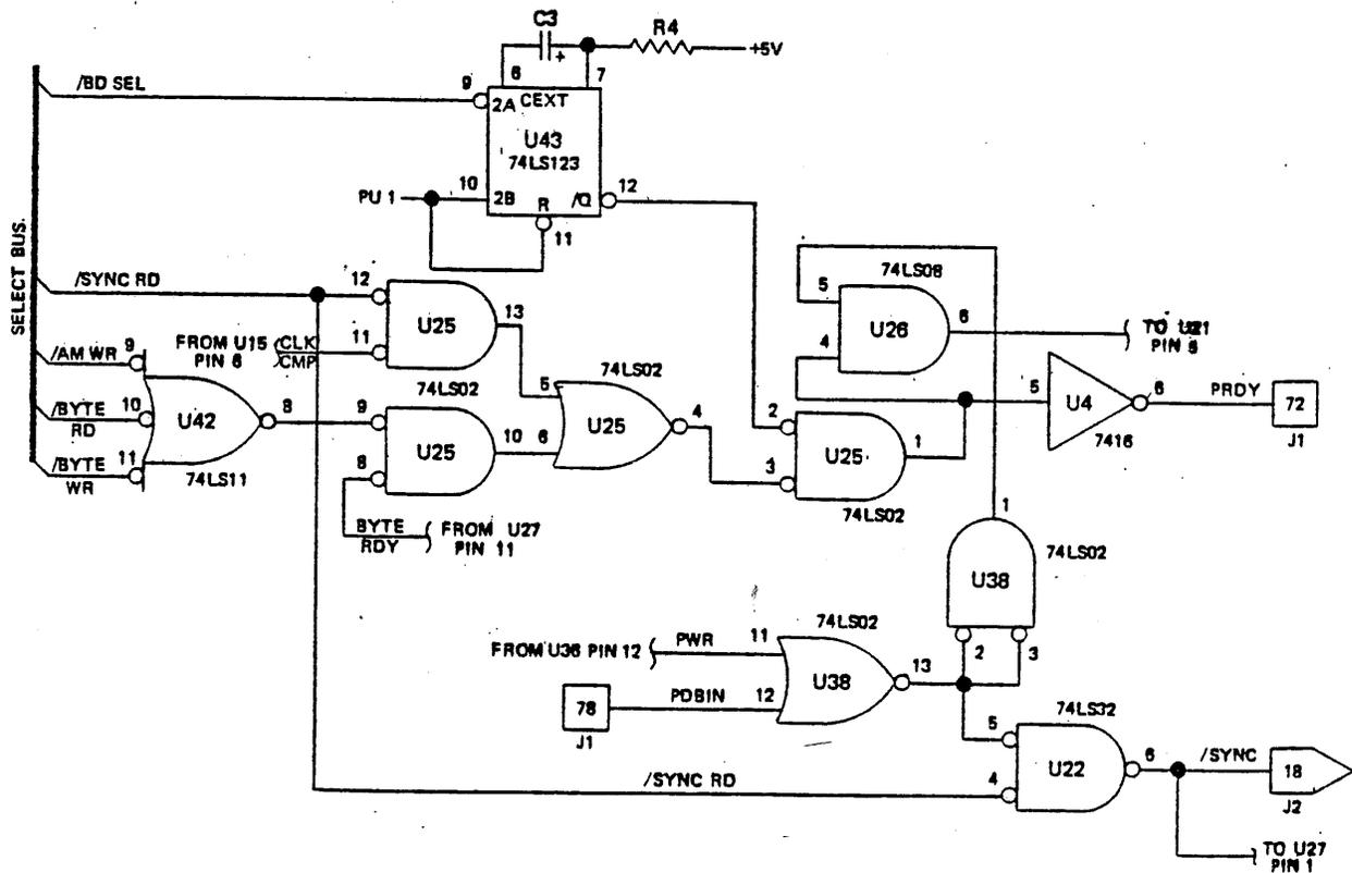
FIGURE 8 Ready Synchronization Logic
