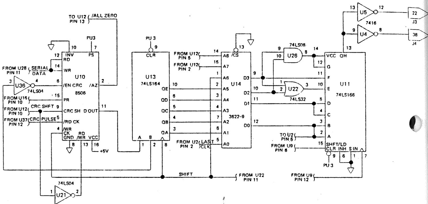
FIGURE 9 CRC and Write Pulse Generation (DIO-C)
