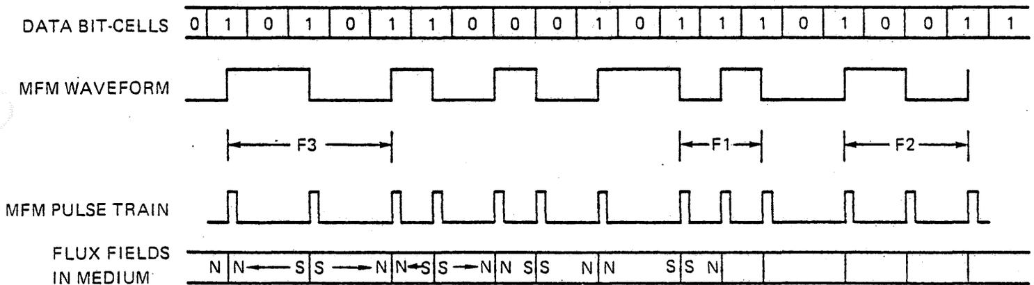
FIGURE 8 MFM Data Encodation
