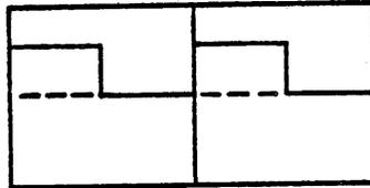
Next monitor U17-5 with the probe. Readjust R36 [R35] CW or CCW until the following waveform appears. Note that the adjustment should continue until the falling edge of the waveform coincides with vertical center of the scope screen.
