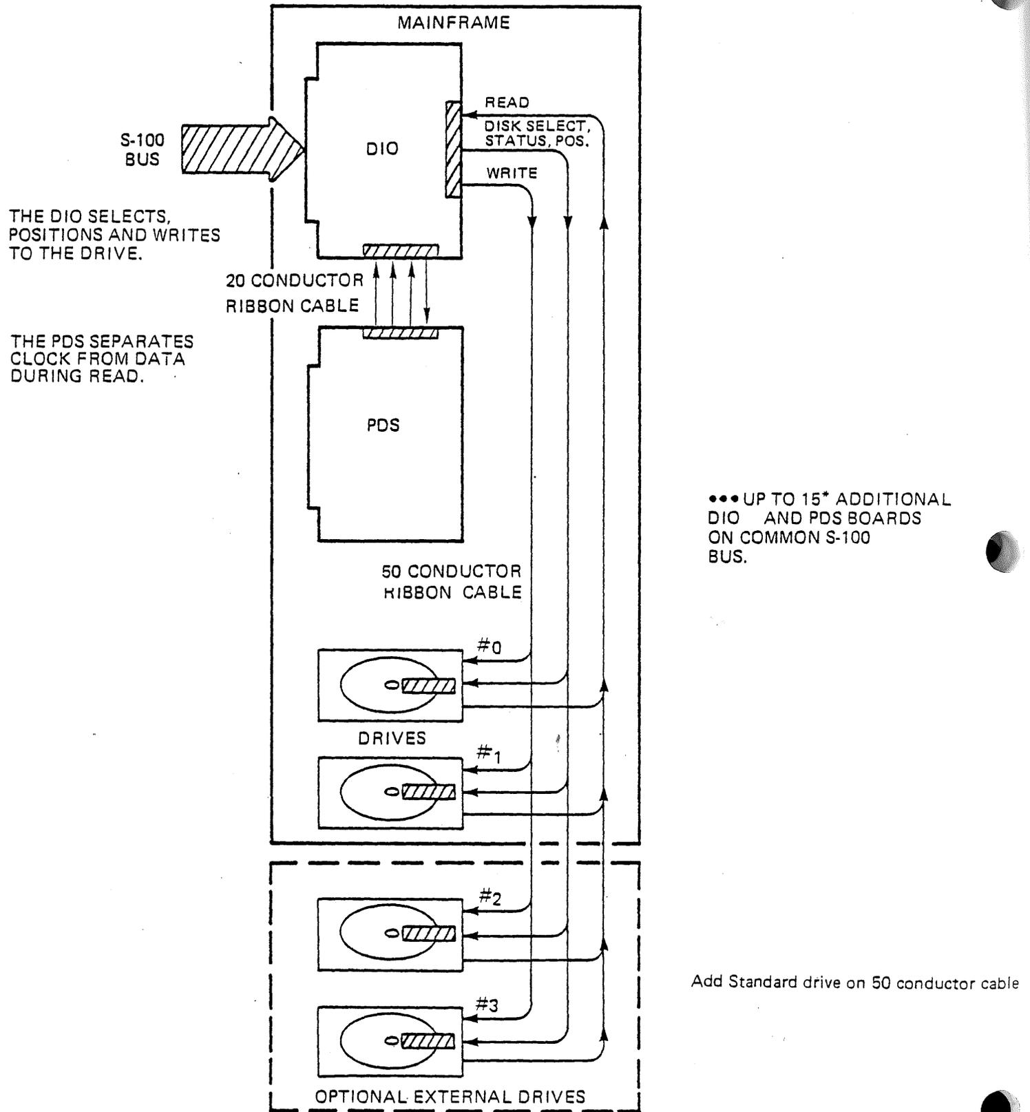
FIGURE 2 DIO/PDS Block Diagram
