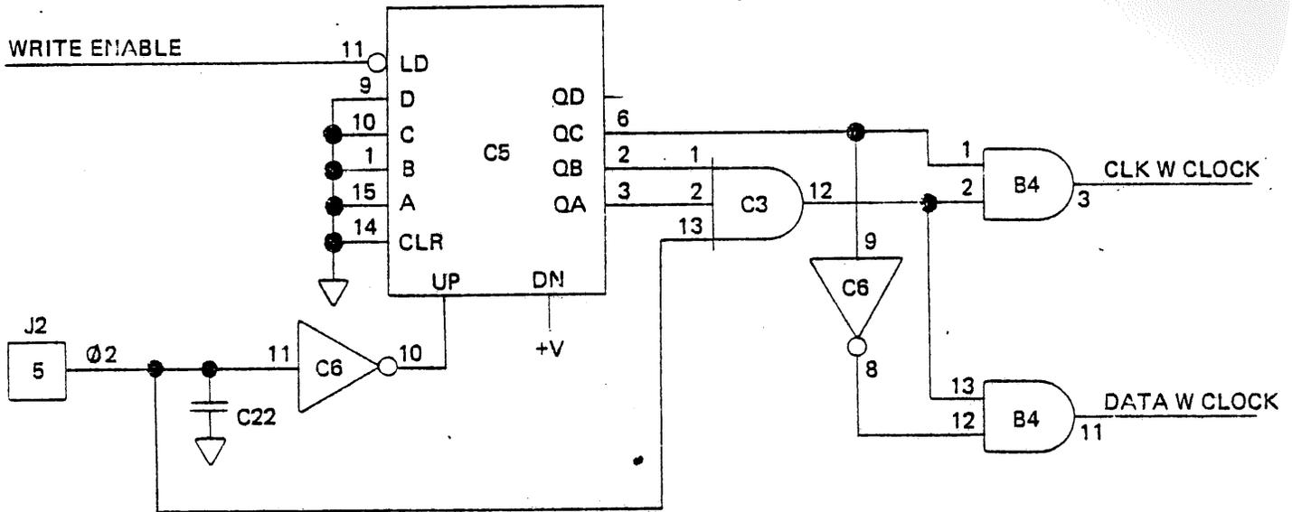
FIGURE 10 Clock W Clock/Data W Clock Generation
