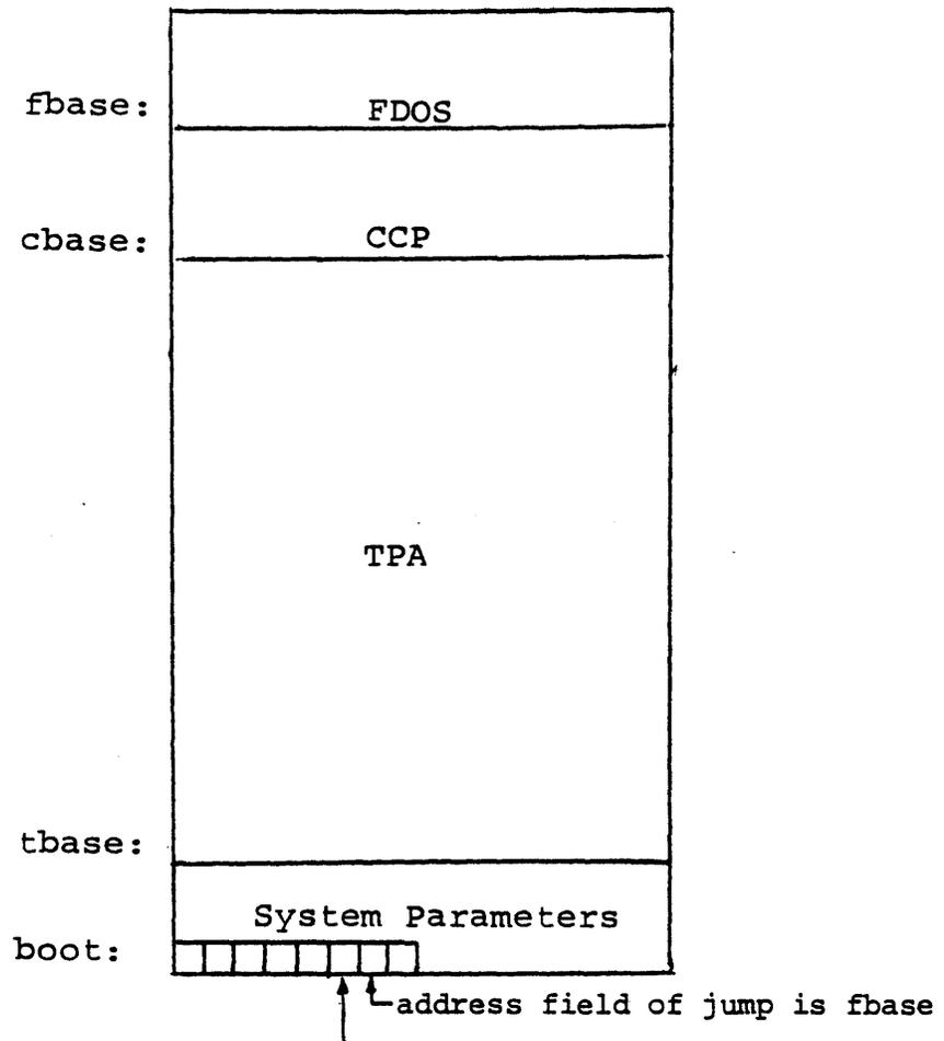
entry: the principal entry point to FDOS is at location 0005 which contains a JMP to fbase. The address field at location 0006 can be used to determine the size of available memory, assuming the CCP is being overlaid.
