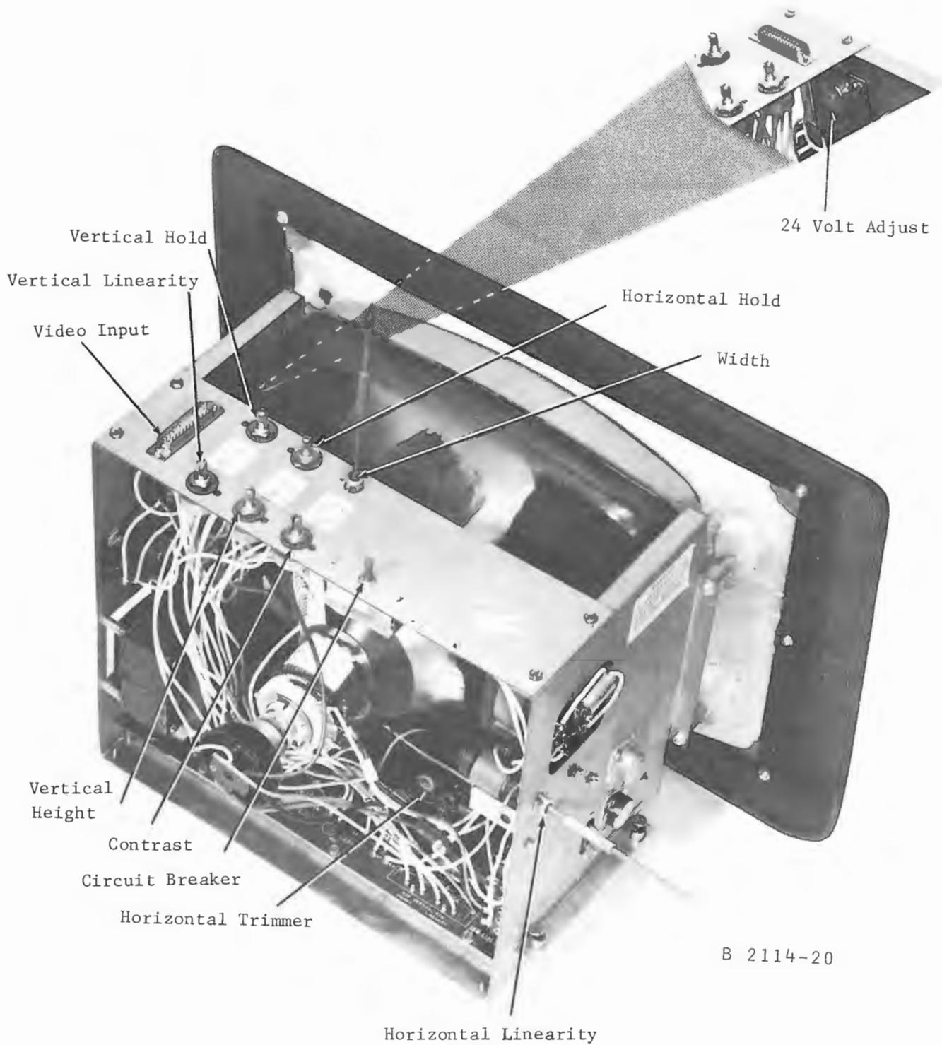
Figure 7-6. T. V. Monitor Adjustments
