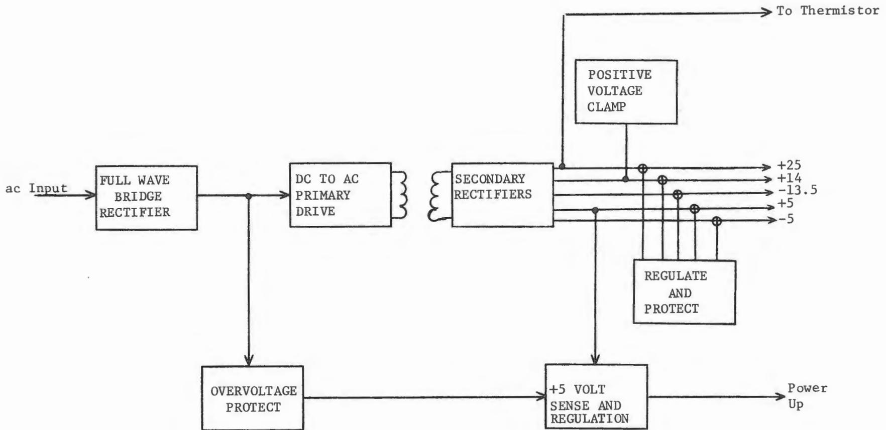
Figure 5-15. Simplified Block Diagram Power Supply
