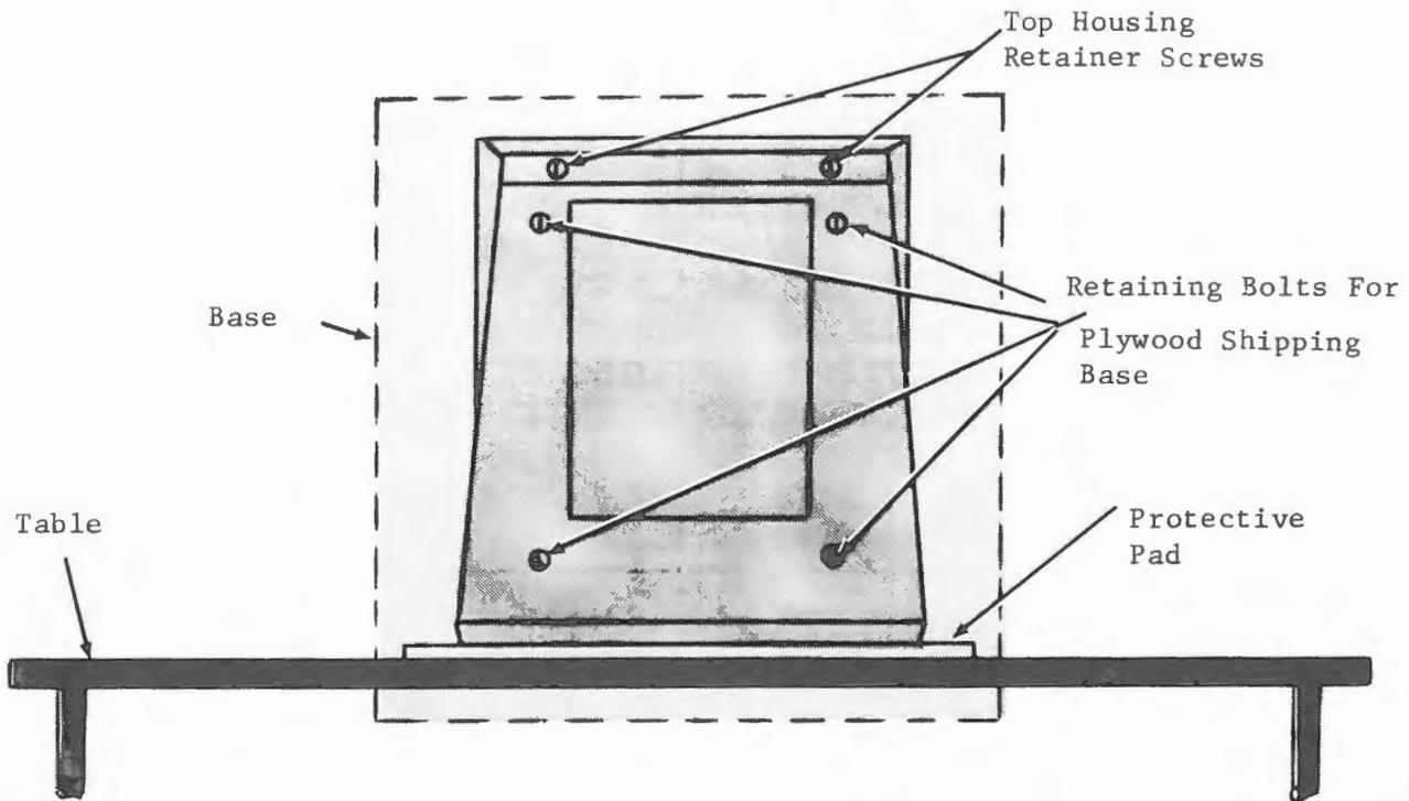
Figure 2-2. Removal of Plywood Base
