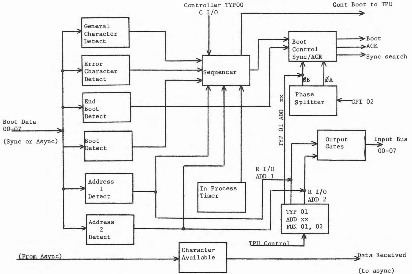
Figure 6-11. Simplified Diagram Boot Controller
