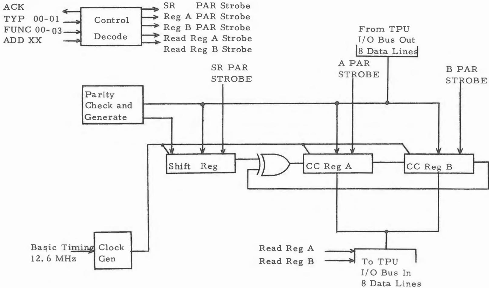
Figure 2. Block Diagram, Cyclic Check Controller
