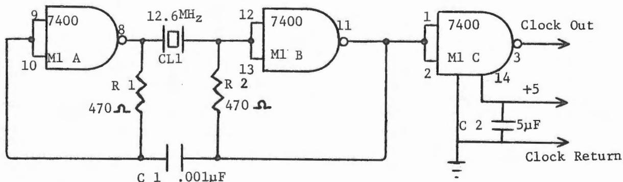
Figure 5-16. Line Lock Oscillator Schematic
