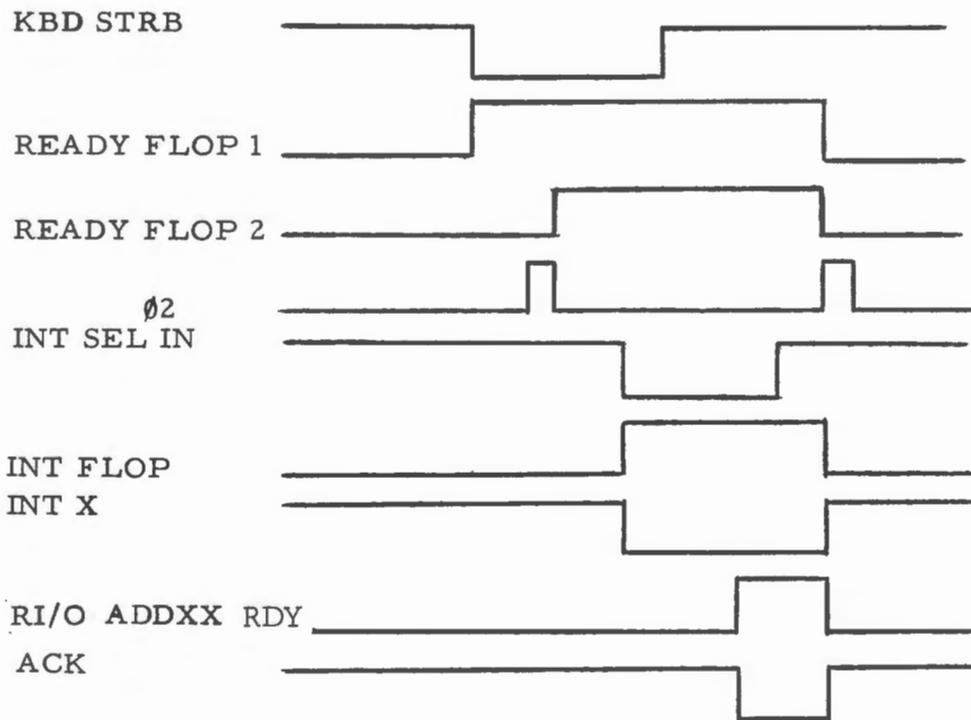
Figure 3. Keyboard Controller Timing
