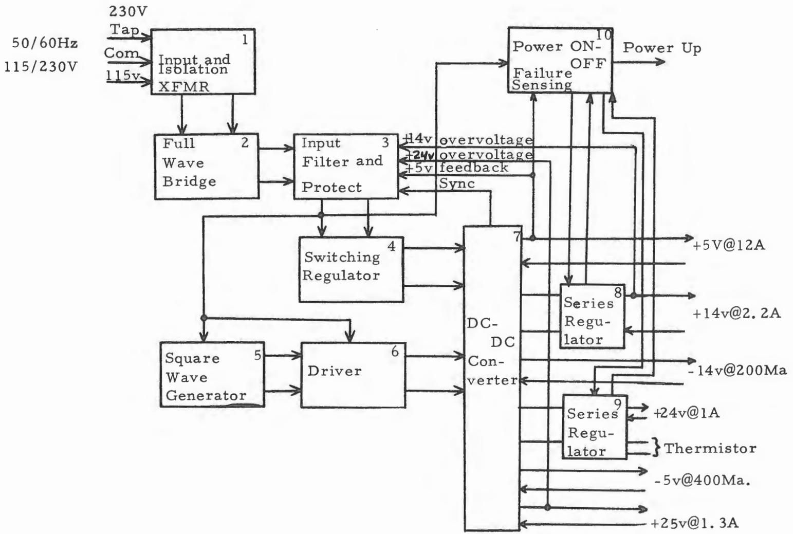
Figure 2. Power Supply Block Diagram
