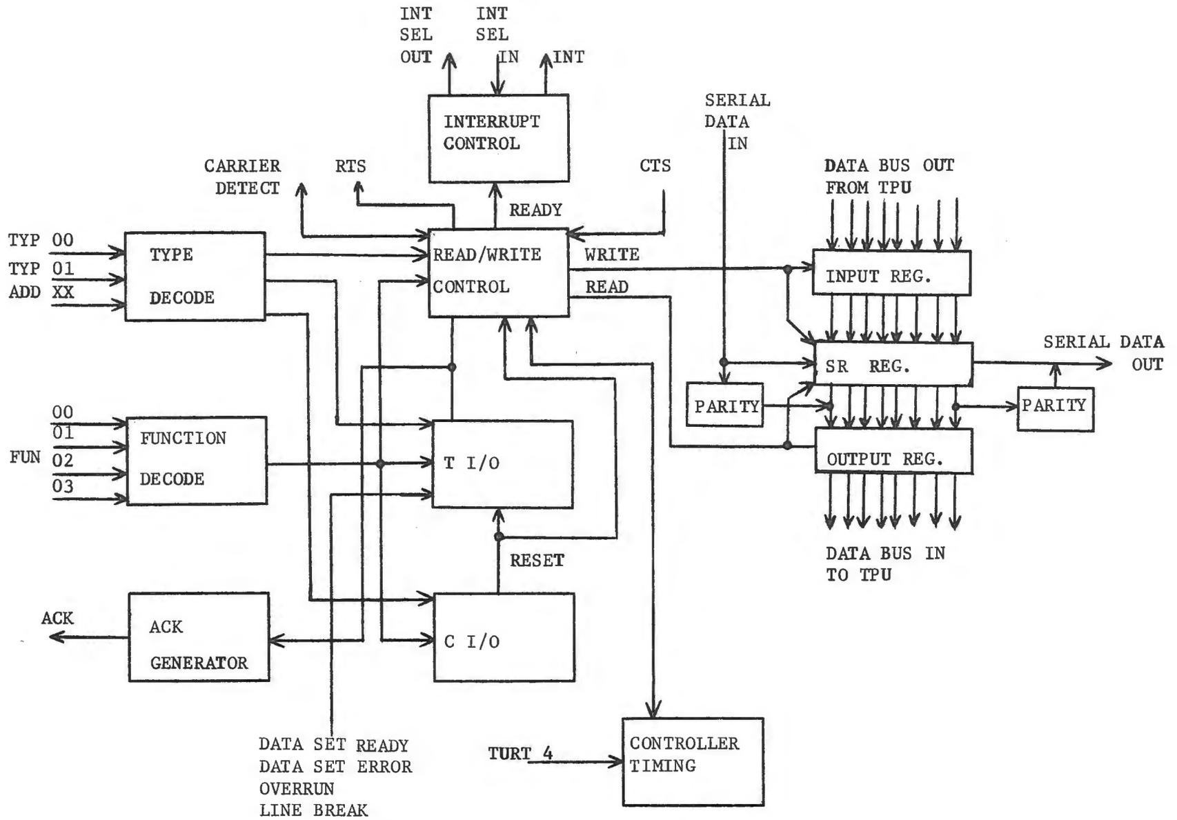
Figure 6-6. Block Diagram Asynchronous Controller
