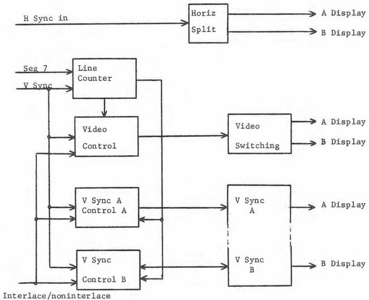
Figure 6-9. Simplified Block Diagram
