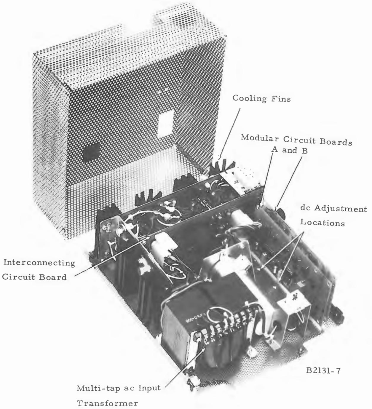
Figure 3. Internal View, Terminal System Power Supply
