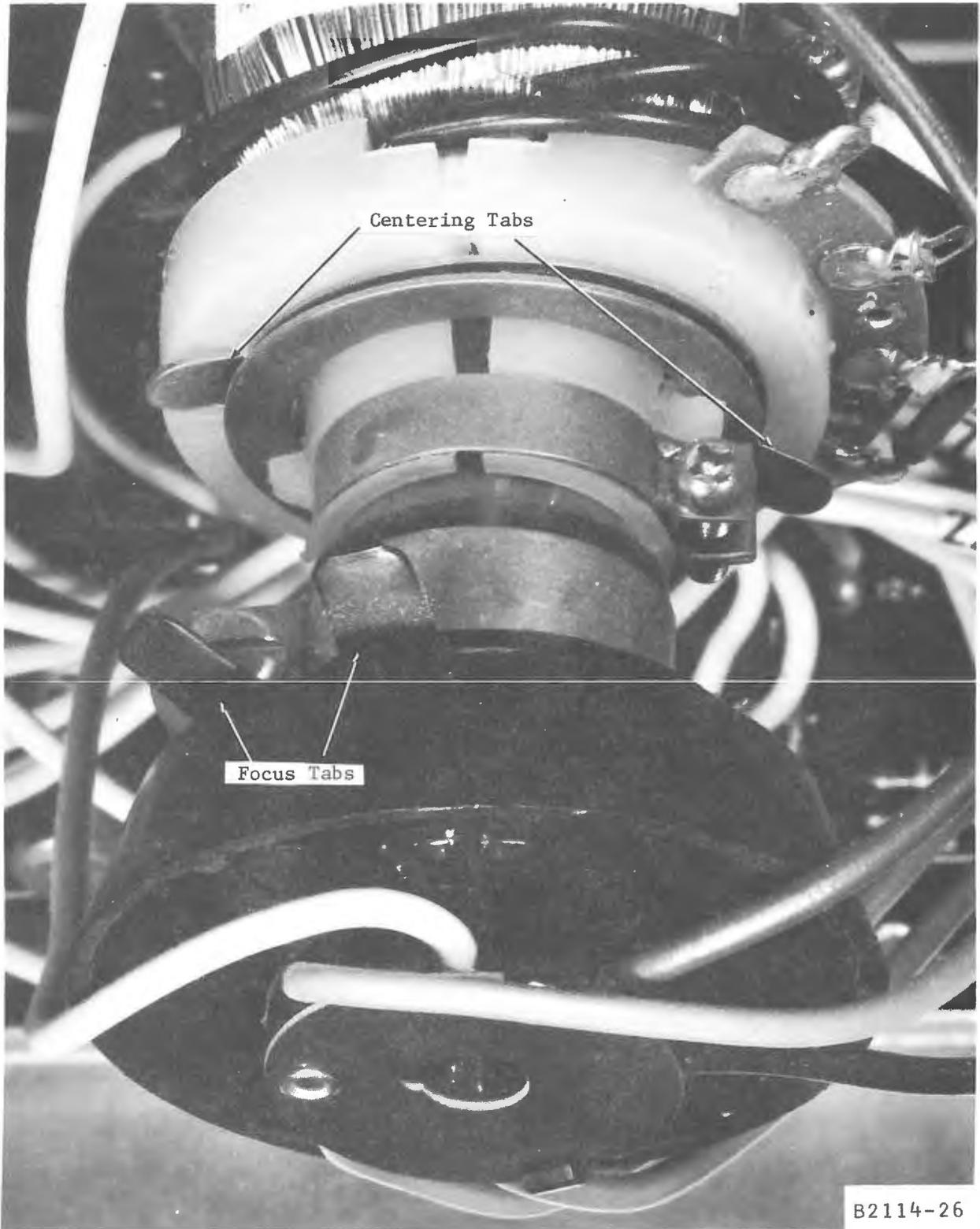
Figure 7-7. Cathode Ray Tube Adjustments
