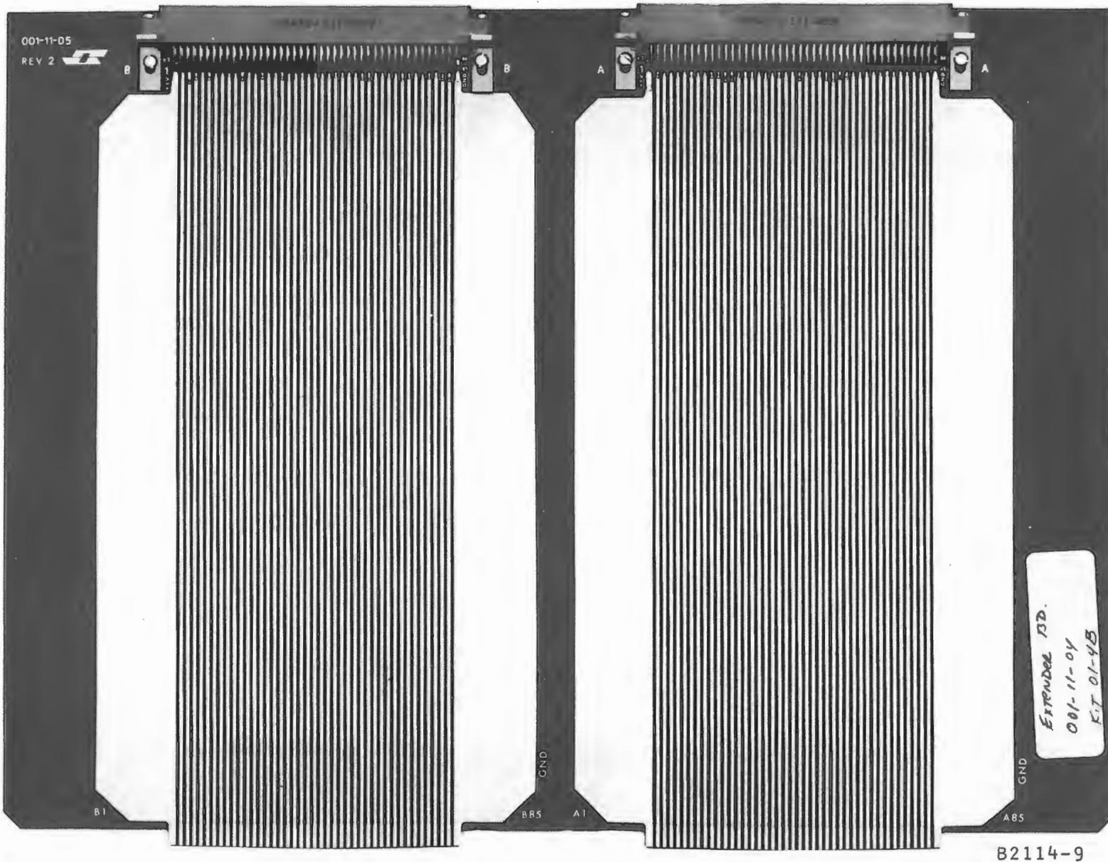
Figure 7-5. Computer Circuit Board Extender
