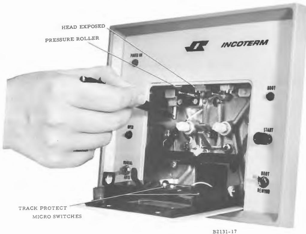
Figure 5-3. Tape Head Exposed
