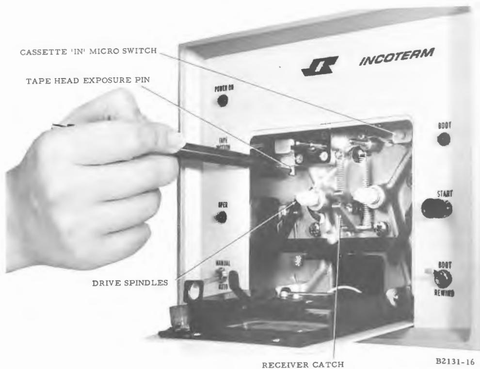
Figure 5-2. Method Used to Expose Parts for Cleaning
