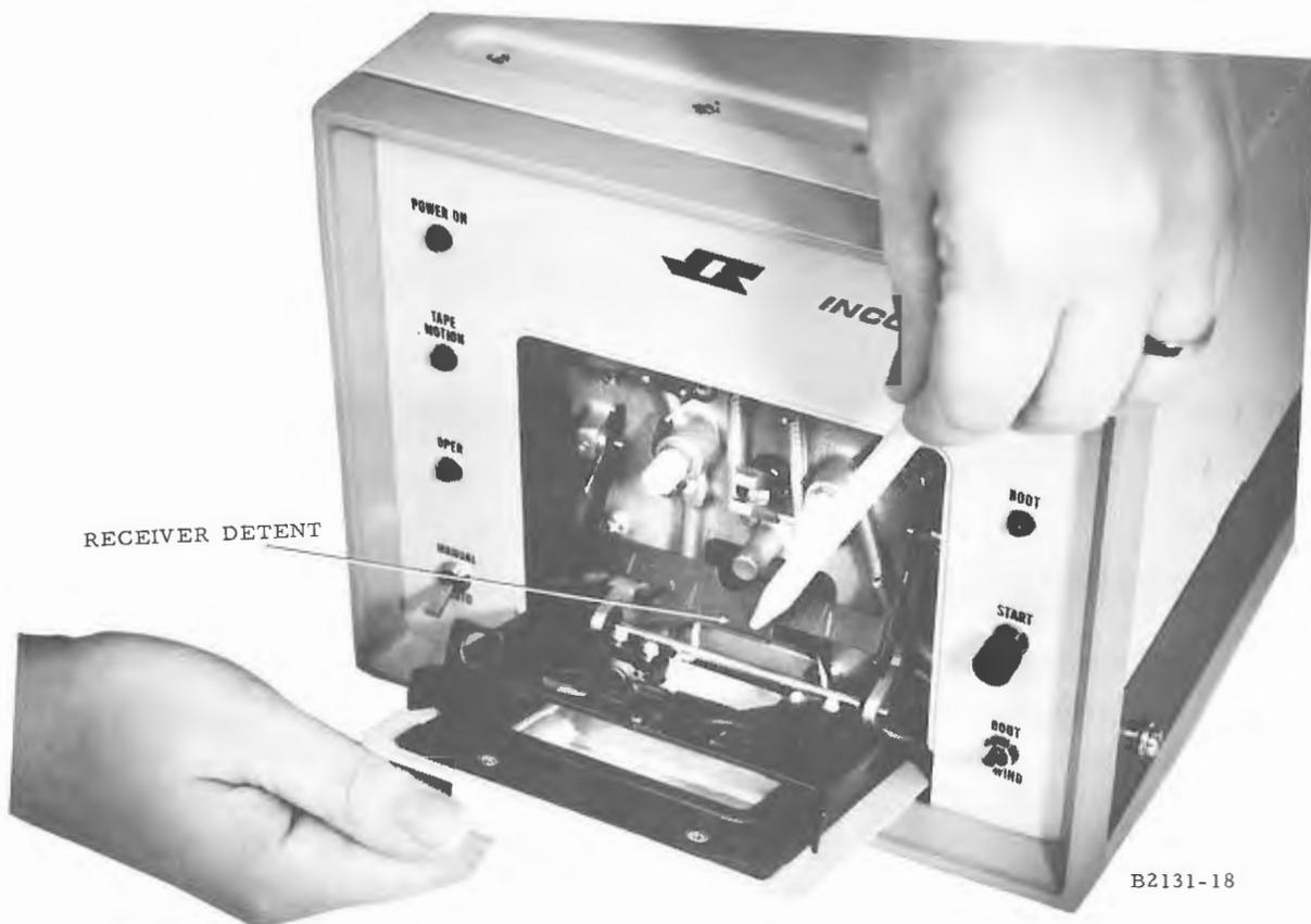
Figure 5-1. Releasing the Receiver Detent
