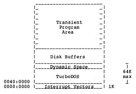
Under 8086 TurboDOS, several transient programs may be loaded into the TPA at one time (although only one may be in execution).
