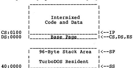
For this "8080 Model", TurboDOS initializes the CS, DS, and ES segment registers to address the single code group. The IP register is set to 0x0100 so that execution starts immediately following the Base Page. The SS and SP registers initially point to a 96-byte stack area provided within TurboDOS.
