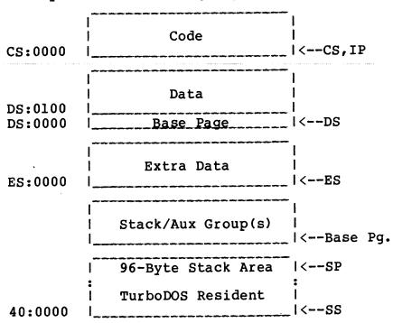
For this "Compact Model", TurboDOS initializes the CS and DS registers to the base of the code and data groups, respectively. ES is set to the base of the extra group if present, otherwise to the data group. The IP register is set to zero. The SS and SP registers initially point to a 96-byte stack area provided within TurboDOS. The stack and auxilliary groups may be located via pointers in the Base Page.
