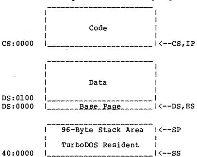
For this "Small Model", TurboDOS initializes the CS register to the base of the code group, and initializes the DS and ES registers to address the base of the data group. The IP register is set to zero. The SS and SP registers initially point to a 96-byte stack area provided within TurboDOS.
