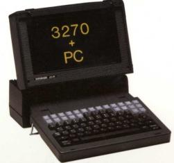
connectivity and ease-of-use in such a compact and affordable package. The dual terminal/workstation personality of the Model 213PT provides the MIS world with ideal solutions for both 3270 dial-in networking and portable application processing on an advanced 386-based PC. With the 213PT the host controls all aspects of the remote IBM computing solution.
