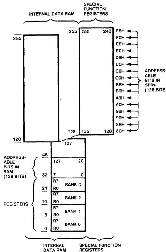
Figure 3-2. Internal Data Addressing Modes
