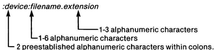
`:device:` is a two character designation for a device. The valid device designations are listed in the next section. The device designation is always enclosed in colons. `:device:` is used alone when an actual device is referenced instead of a file that resides on a device.
