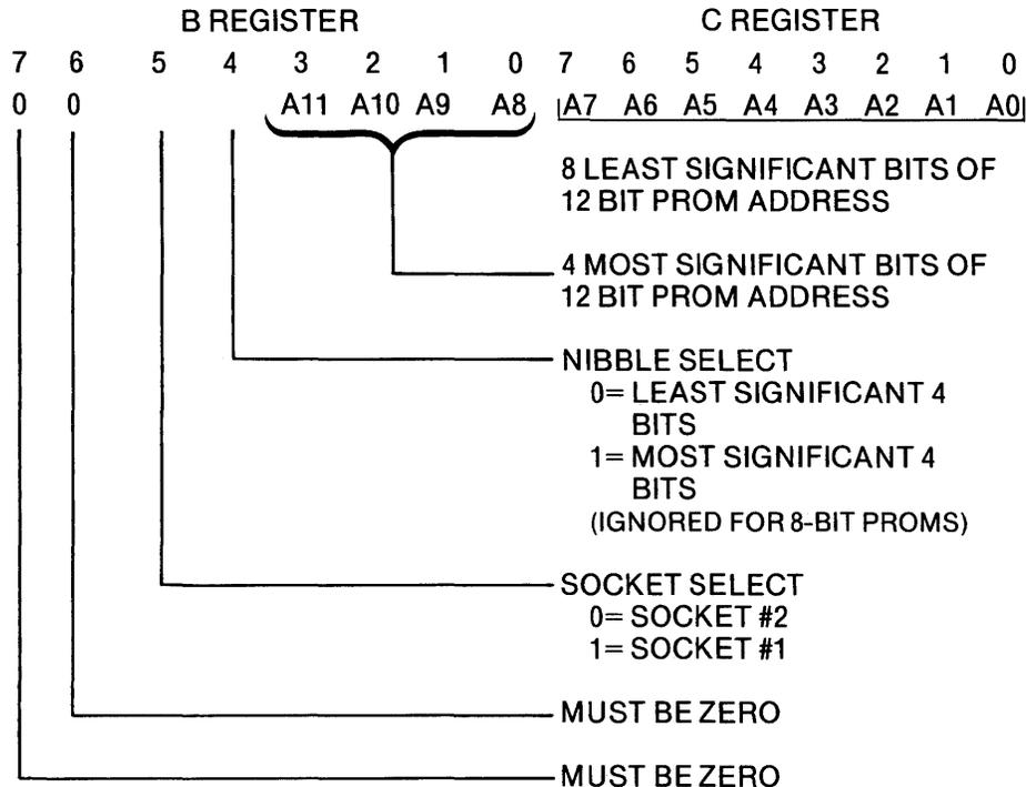
Before calling the Universal PROM Programmer Input routine, you should call the Universal PROM Programmer Status routine (described later in this chapter) to ascertain the current status of the UPP. If an error occurs in the process of reading from the UPP, the content of the A-register is meaningless. Thus, you should follow the call to the UPP input routine with another call to the UPP status routine.
