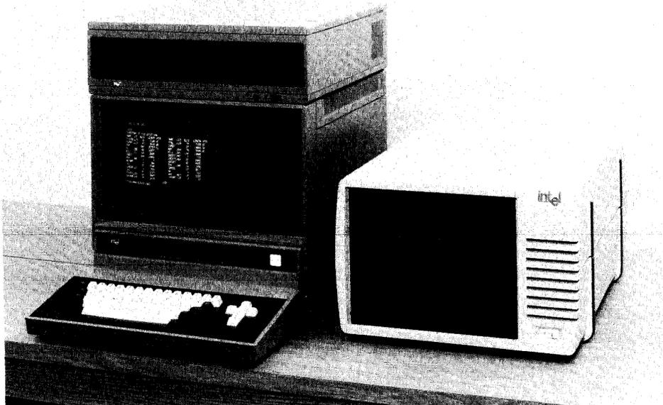
Figure 1-4. System with Winchester Disk Subsystem 121575-4
