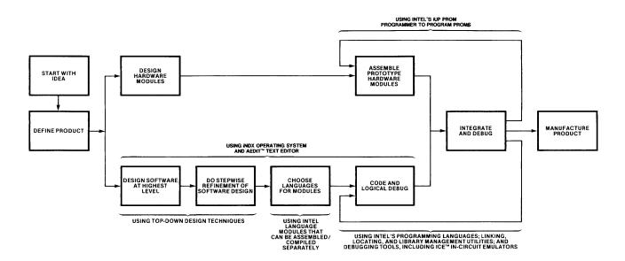
Figure 1-1. Microcomputer System Development Process
