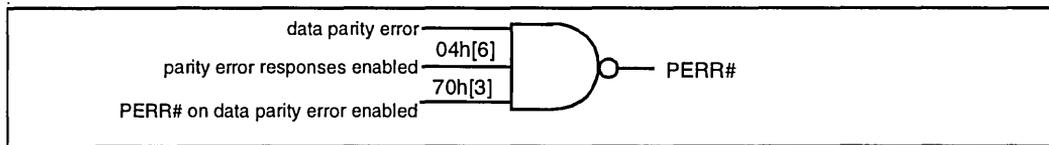
Figure 3. Logic Diagram of the Assertion of PERR#
