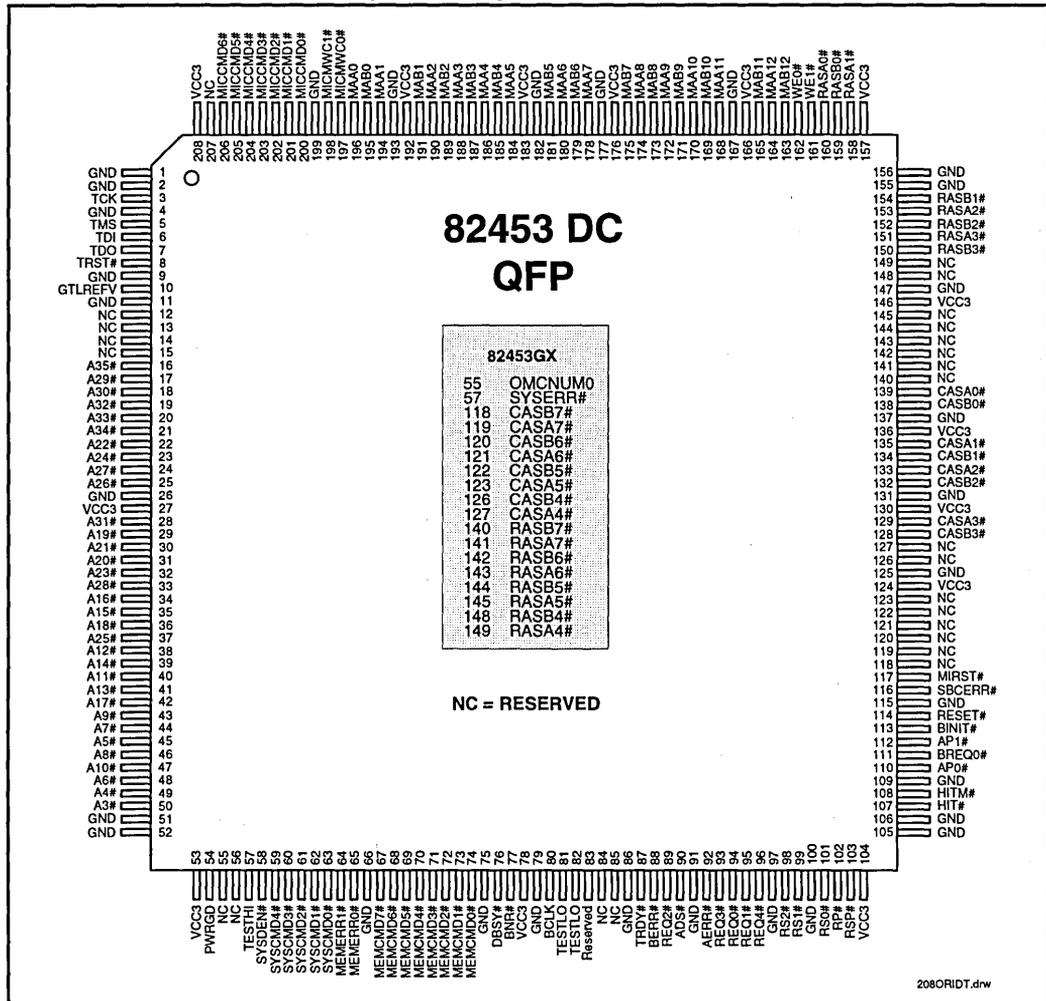
Figure 7. 82453KX/GX DC Pin Assignment (208-Pin QFP)
