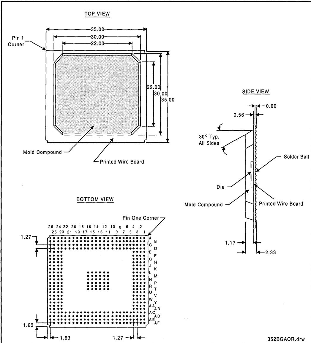
Figure 16. 82454KX/GX PB Package Physical Dimensions (352 BGA)
