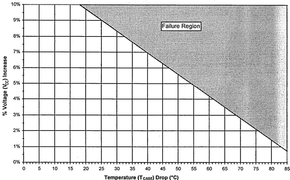
Figure 1. V<sub>CC</sub> Increase vs. T<sub>CASE</sub> Drop for DPLL Failure (Worst Case)
