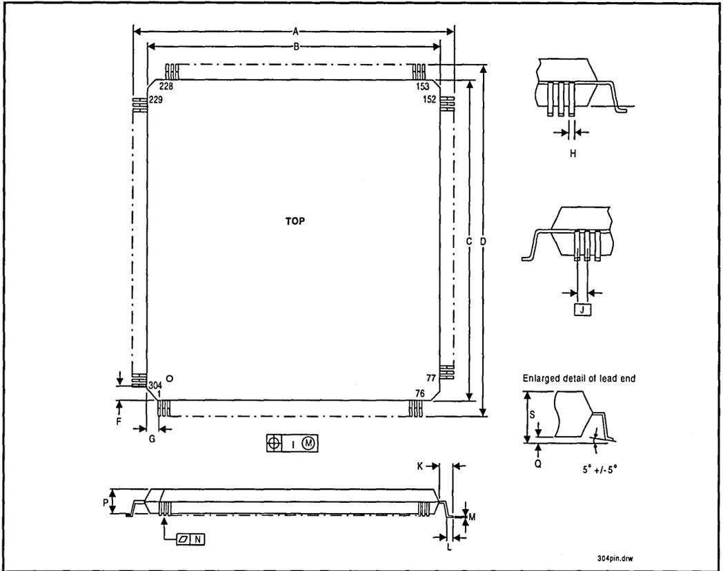
Figure 15. 82454KX/GX PB Package Physical Dimensions (304-Pin QFP)
