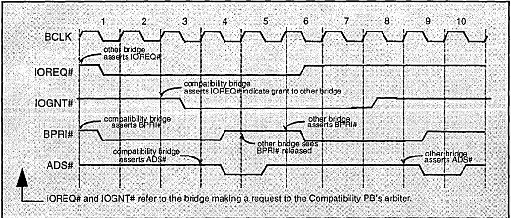
Figure 8. BPRI# Arbitration Overlapped with Bridge Transfer
