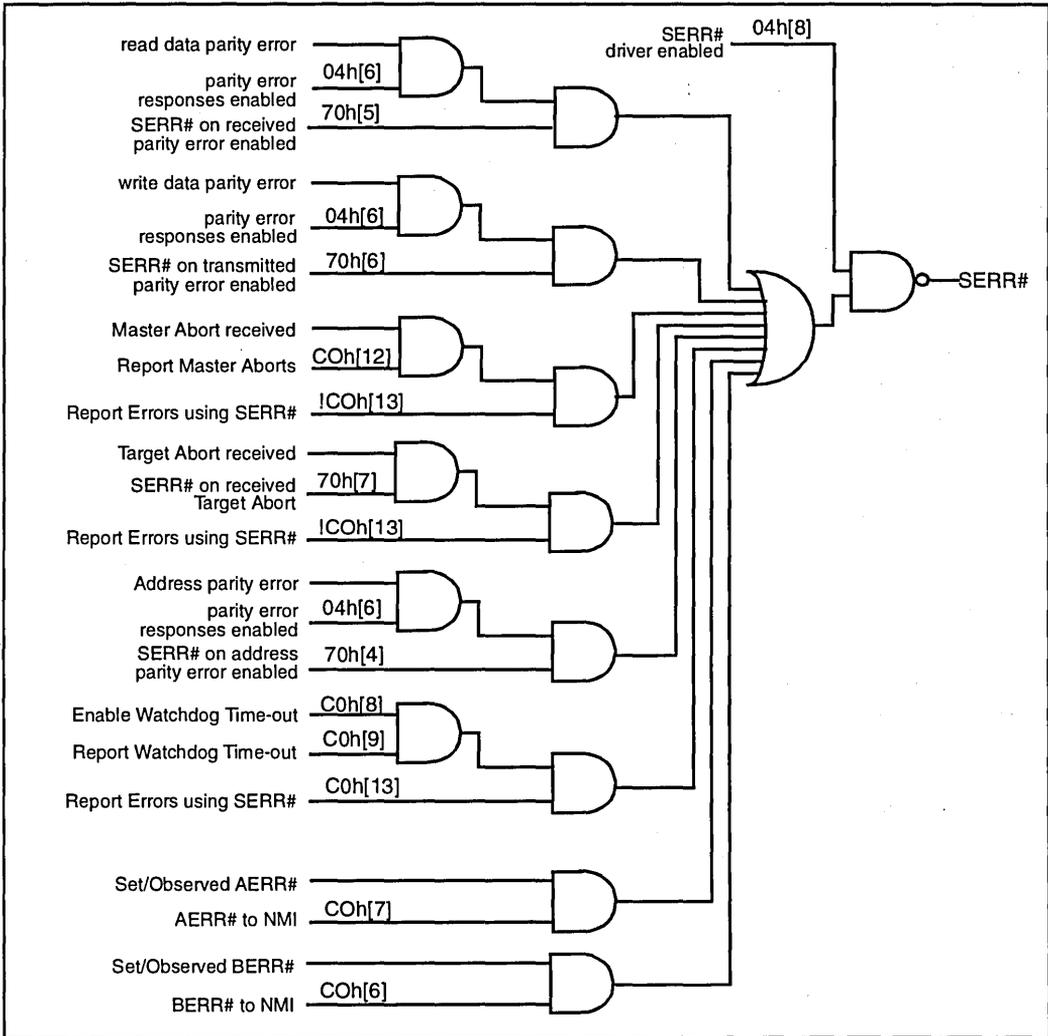
Figure 5. Logic Diagram of the Assertion of SERR#
