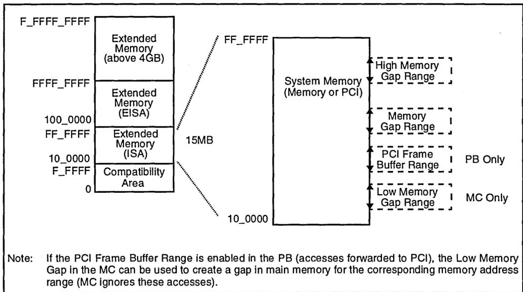
Figure 4. Expanded View of Extended Memory (ISA)
