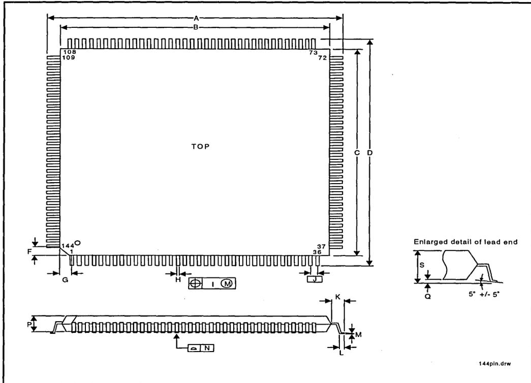
Figure 14. MIC Package Physical Dimensions (144-Pin QFP)
