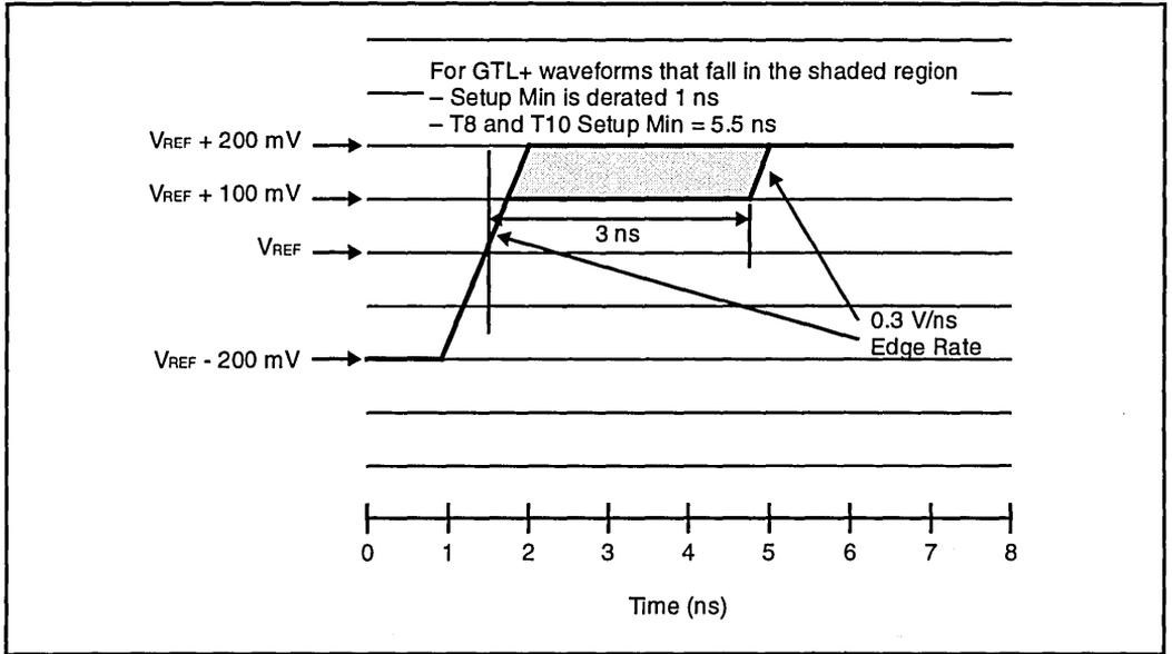
Figure 5. Exception to GTL+ Minimal Input Waveform With Setup Impact
