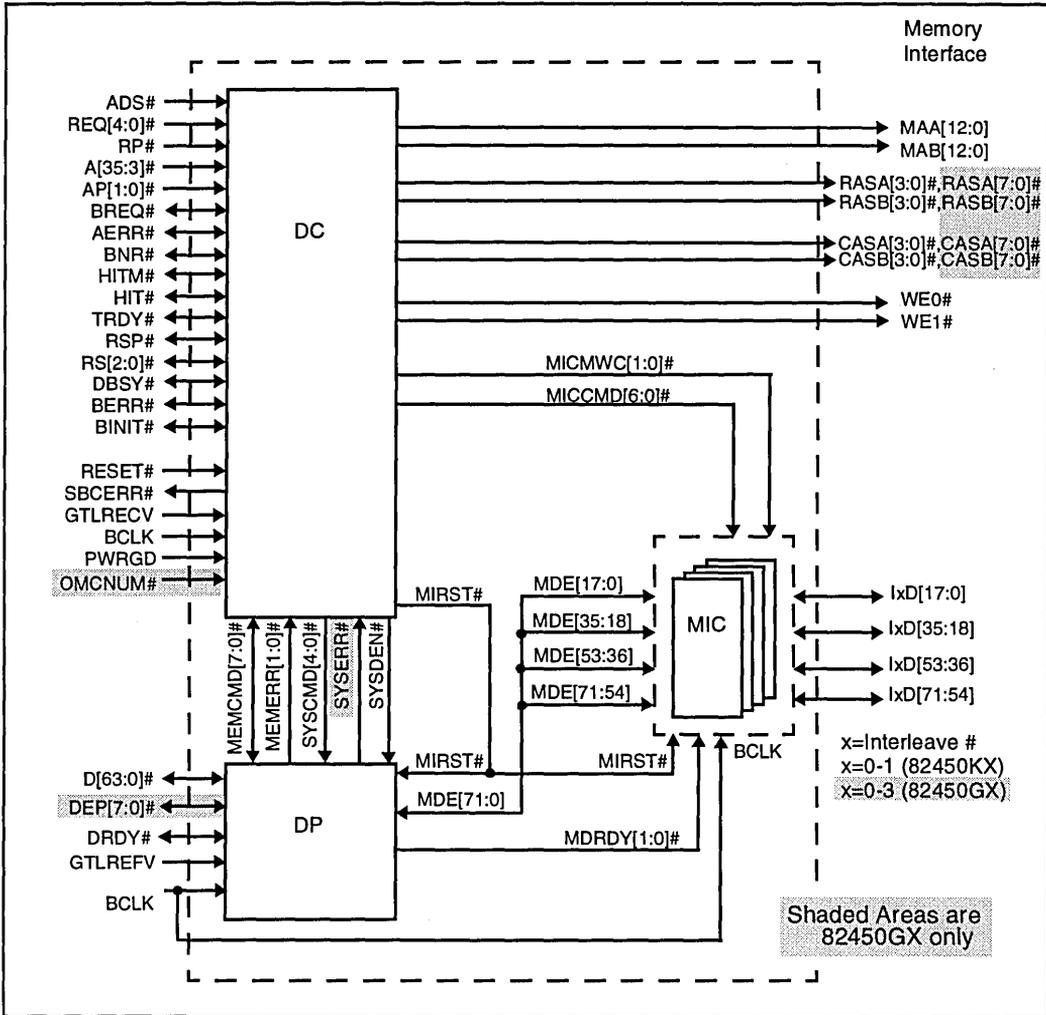
Figure 1. Memory Controller (MC) Simplified Block Diagram
