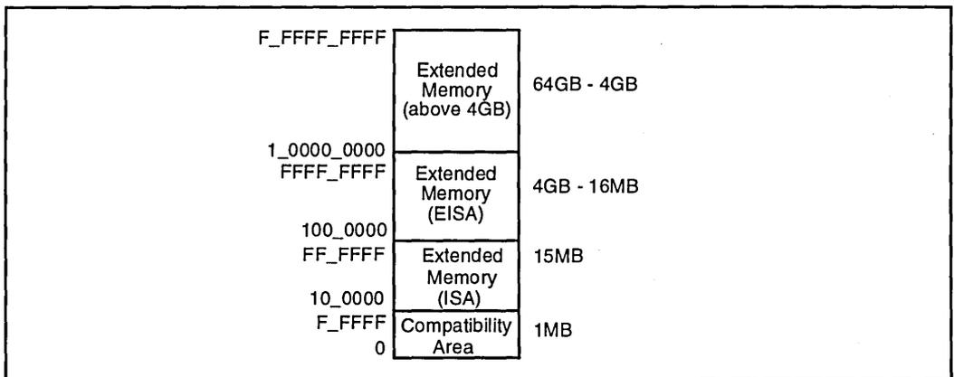
Figure 2. Pentium Pro Processor Memory Address Space.
