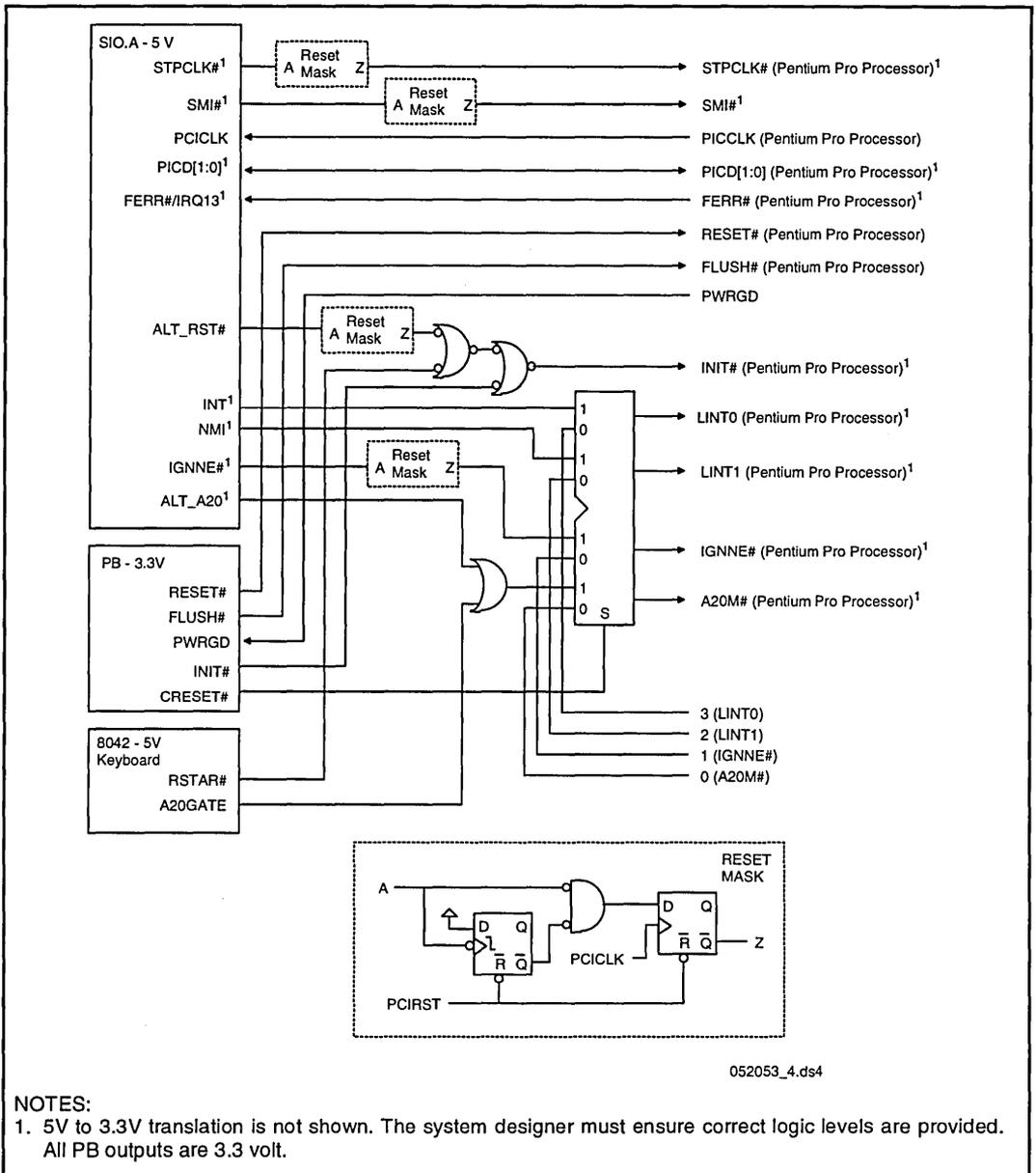
Figure 12. Blocking Logic For 82420KX/GX Designs Using the 82379AB SIO.A
