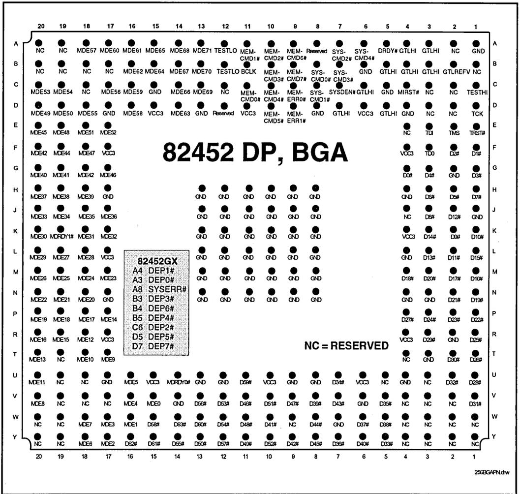
Figure 9. 82452 DP Pin Assignment (256 BGA)
