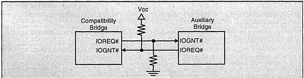
Figure 9. IOGNT# & IOREQ# Pull-Ups/Pull-Downs (Dual Bridge System)
