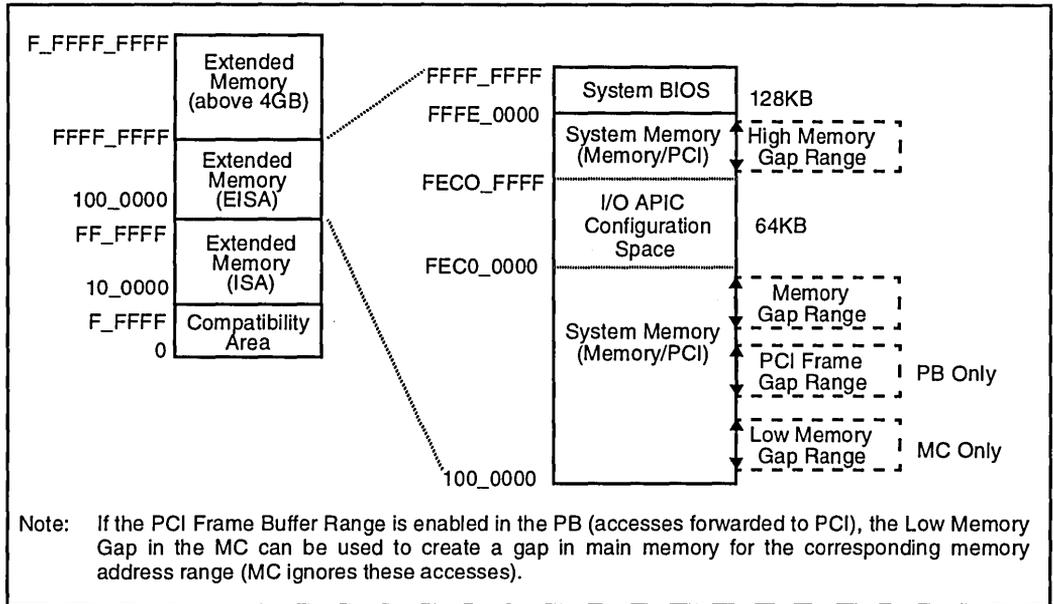
Figure 5. Expanded View of Extended Memory (EISA).
