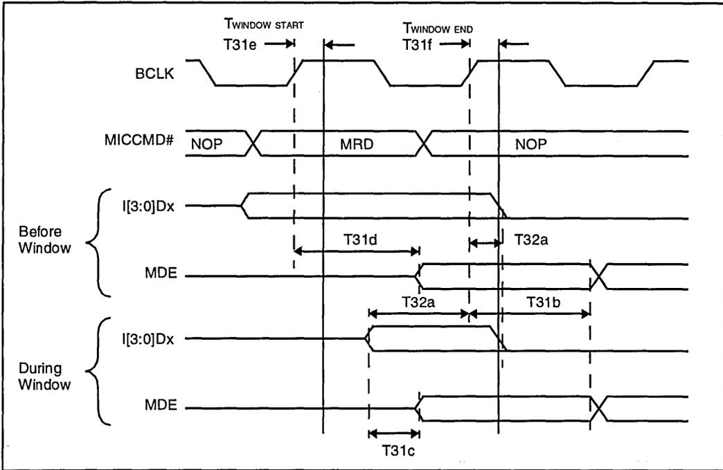
Figure 7. System Memory Signals [Memory Read (MIC)]
