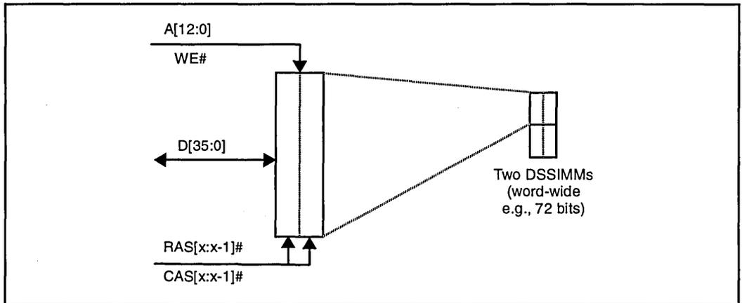
Figure 2. Signal Connections to a Double-Sided SIMM
