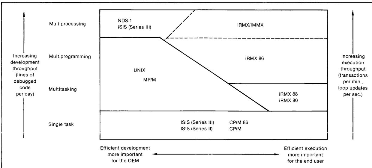
Fig. 1.  $\mu$ C operating systems are design-optimized for efficient execution for end users (right) or for efficient program development for OEMs (left). They range from single-task, single-terminal systems (bottom) to multiprocessing systems (top).
