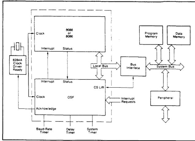
**FIGURE 2. The OSF component works with systems that use the iAPX 86, 88, 186, or 188 microprocessor. Close coupling of the CPU and the OSF allows maximum zero-wait-state performance of the OSF software.**
