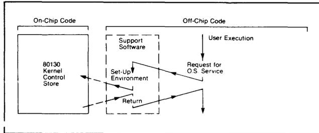
**FIGURE 3. The position-independent interface supplies data location and run-time values, and starts on-chip execution of the software.**
