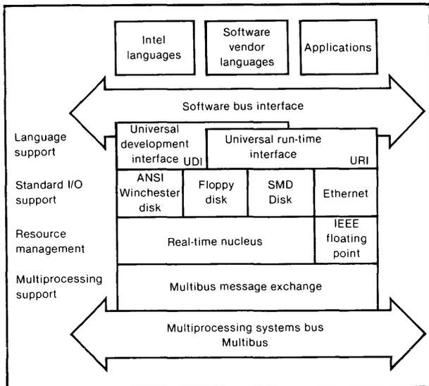
**Fig. 2. Layered operating systems with standard interfaces, standard modules and configurability are key elements in designing  $\mu$ c operating systems to take maximum advantage of lower cost, higher performance VLSI.**
