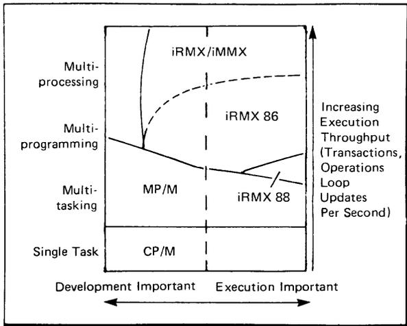
**Figure 2: These microcomputer operating systems are primarily for efficient execution.**
