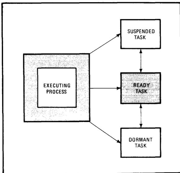
**2. Task states.** As one task (or process) runs, others may be in various states of readiness. In Hunter & Ready's VRTX, for example, tasks can be ready (able to run immediately), suspended (waiting for a resource), or dormant (deleted by a system call).
