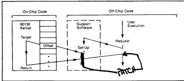
**FIGURE 4.** All on-chip accesses are routed through the on-chip stepping-independence interface, which provides compatibility between on-chip and off-chip code. Because the interface structure stays constant, the external reference also stays constant, while the on-chip OFFSET changes to point to the new location of the on-chip code.
