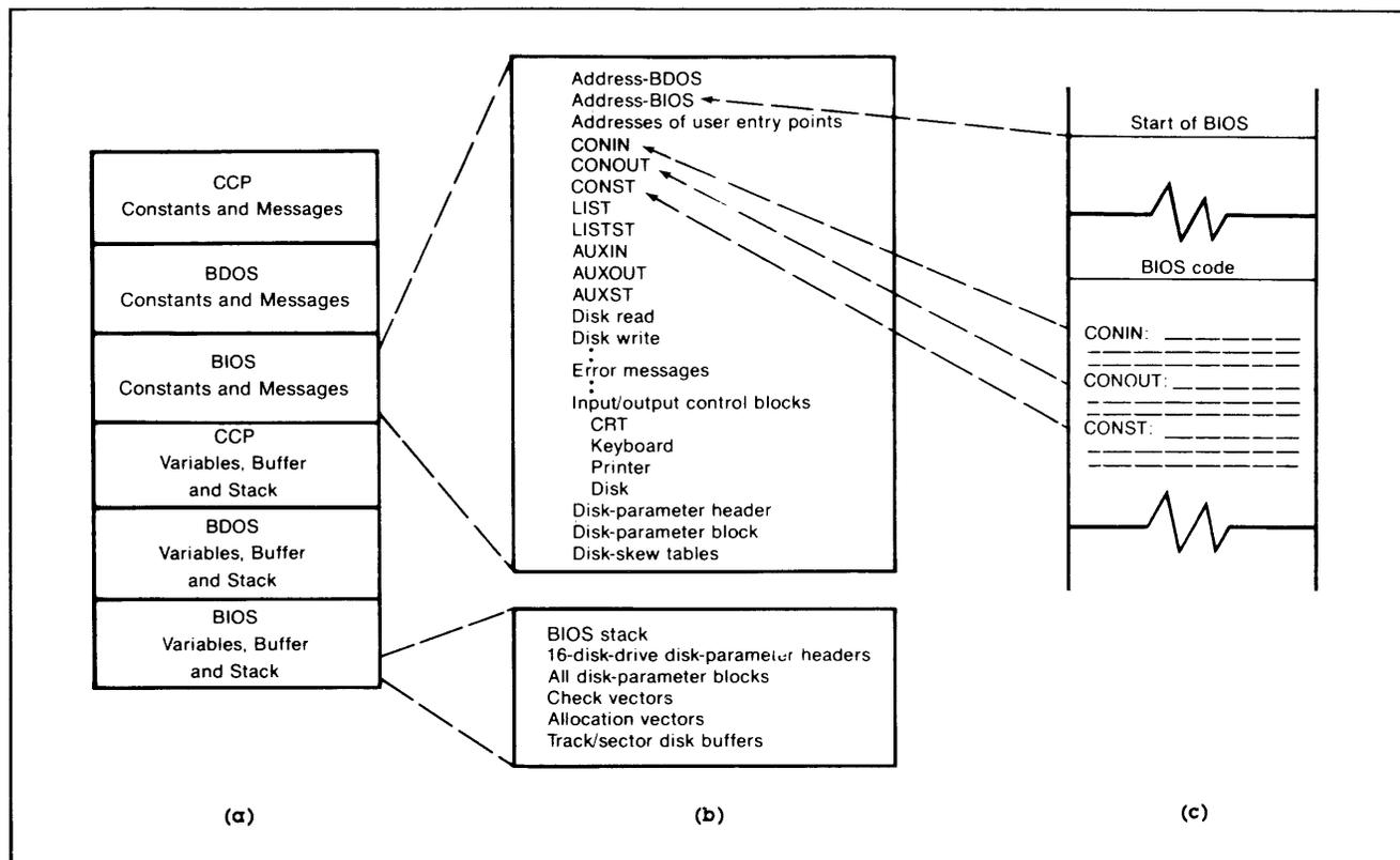
FIGURE 6. The Configuration Block (CB) reconfigures the BIOS for specific hardware systems. a) The CB contains read-down from the 80150, and variables used at run-time. b) The BIOS portion of the CB contains configuration-dependent data. c) These addresses provide access to the 80150 on-chip code, to alter execution paths for different configurations and steppings.
