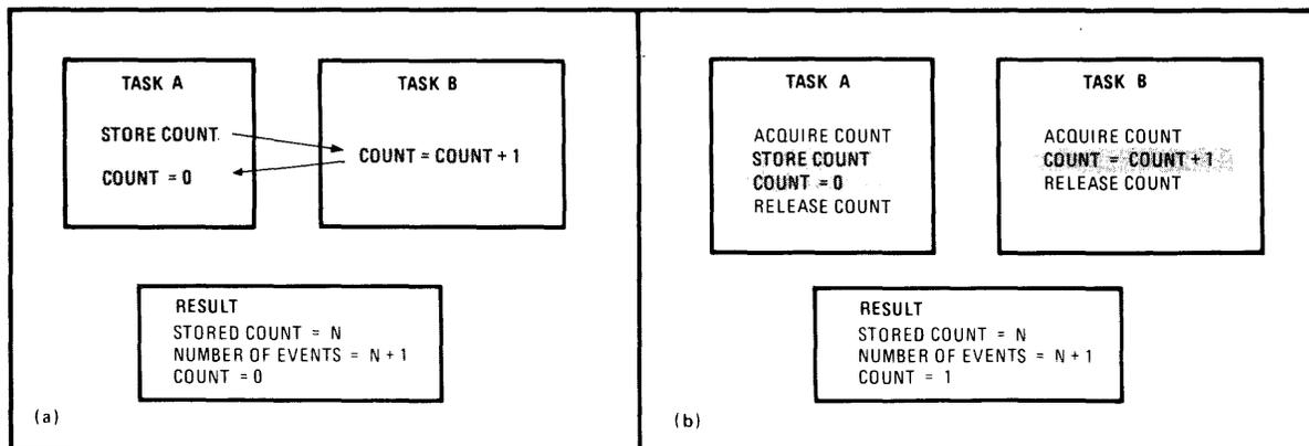
**3. Critical regions.** If two asynchronous tasks use a counter, events can be miscounted if task B interrupts task A before the counter is reset (a). Forcing the tasks to acquire a counter before using it (b) ensures synchronization through the critical regions (tinted).
