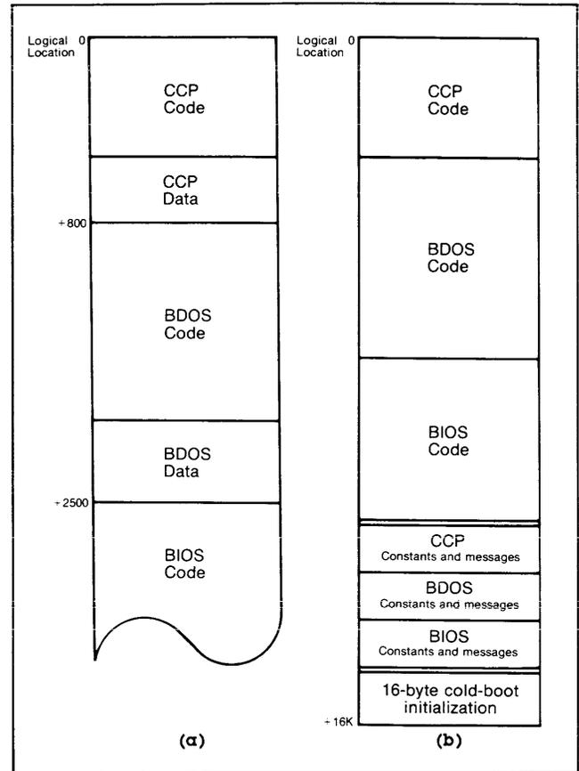
**FIGURE 5.** (a) The standard disk-based CP/M-86 module is one long structure containing both code and data. (b) Intel reorganized the basic CP/M-86 architecture to fit the operating system into the 80150 OS firmware component.
