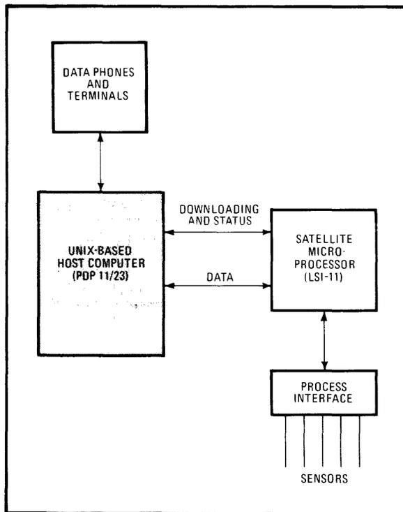
**1. Satellite processing.** In Bell Labs' Concepts system, separate microprocessors handle low-level details of process control. Yet another processor—a host computer that runs the Unix operating system—is in charge of coordinating these satellite machines.
