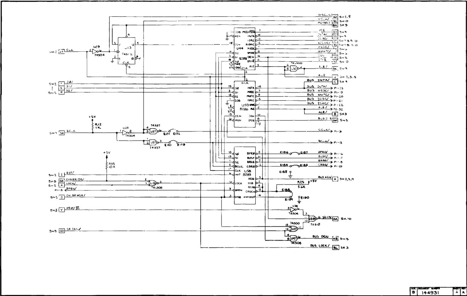
Figure 4-3. ISBC® 86/05 Board Schematic Diagram (Sheet 3 of 10)
