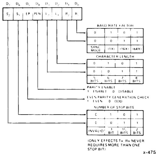
Figure 3-6. PCI Asynchronous Mode Instruction Word Format
