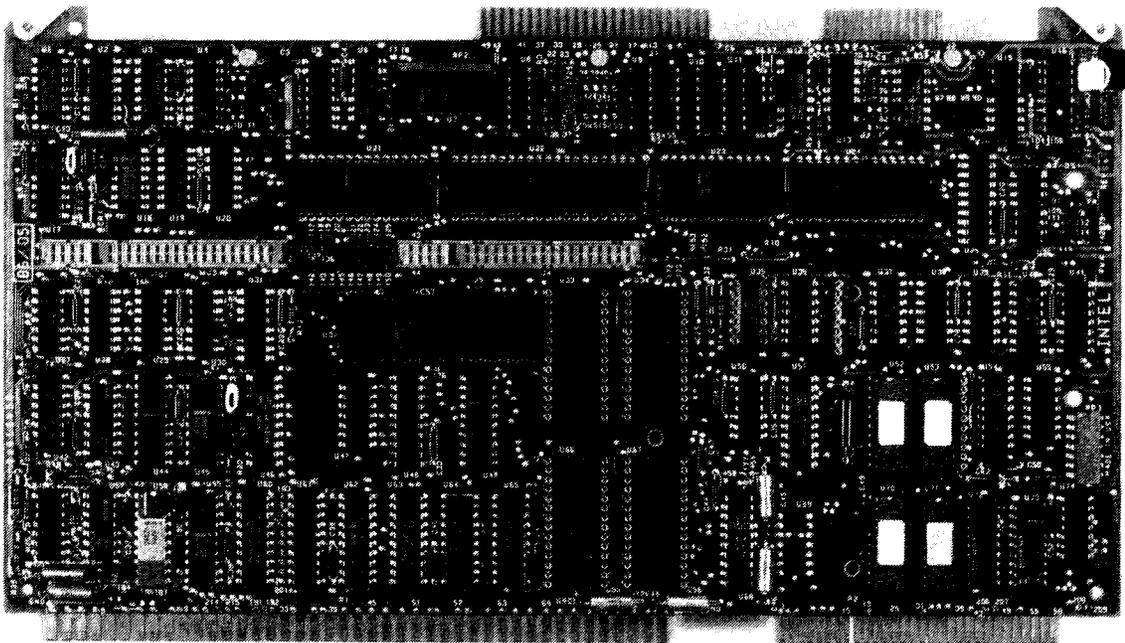
Figure 1-1. iSBC<sup>®</sup> 86/05 Single Board Computer
