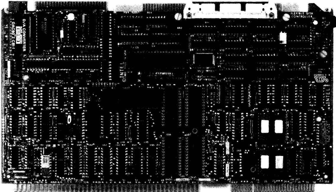
Figure 1-2. iSBC<sup>®</sup> 86/05 Board With Optional Multimodule Boards
