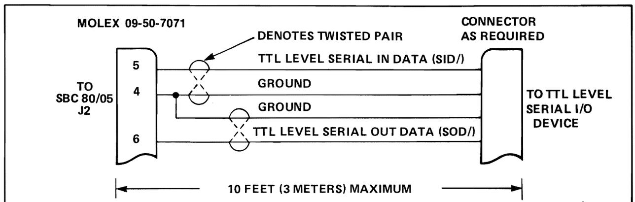
Figure 2-8. TTL Level Serial I/O Device Interface Cabling
