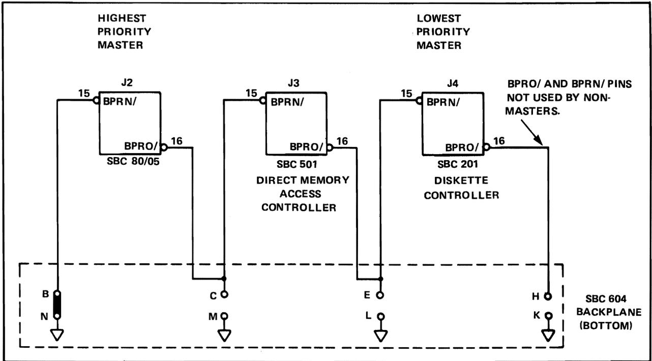
Figure 2-5. Serial Priority Resolution Scheme
