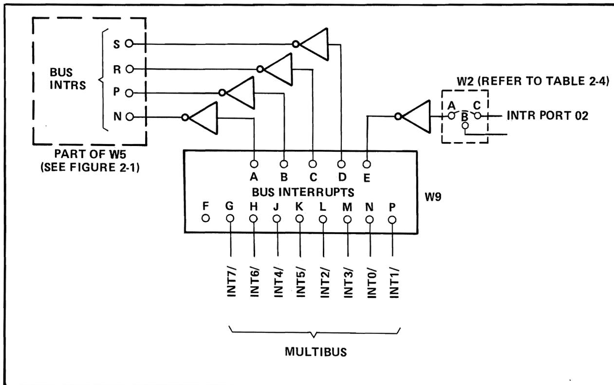
Figure 2-2. Multibus Interrupt Jumpers
