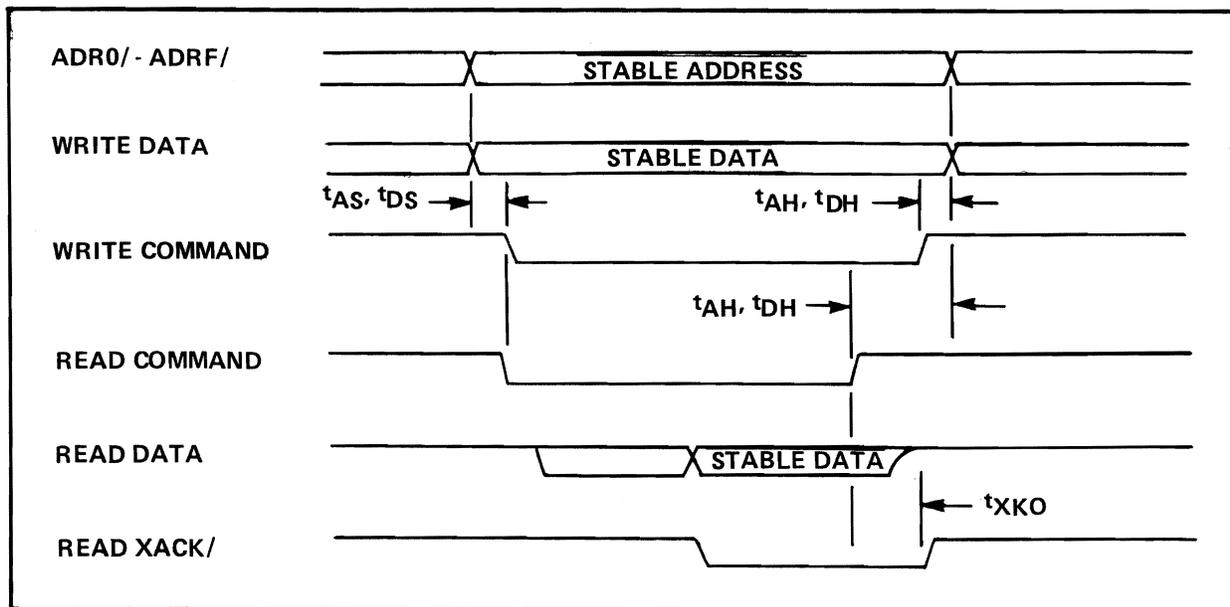
Figure 2-4. SBC 80/05 Bus Control Timing
