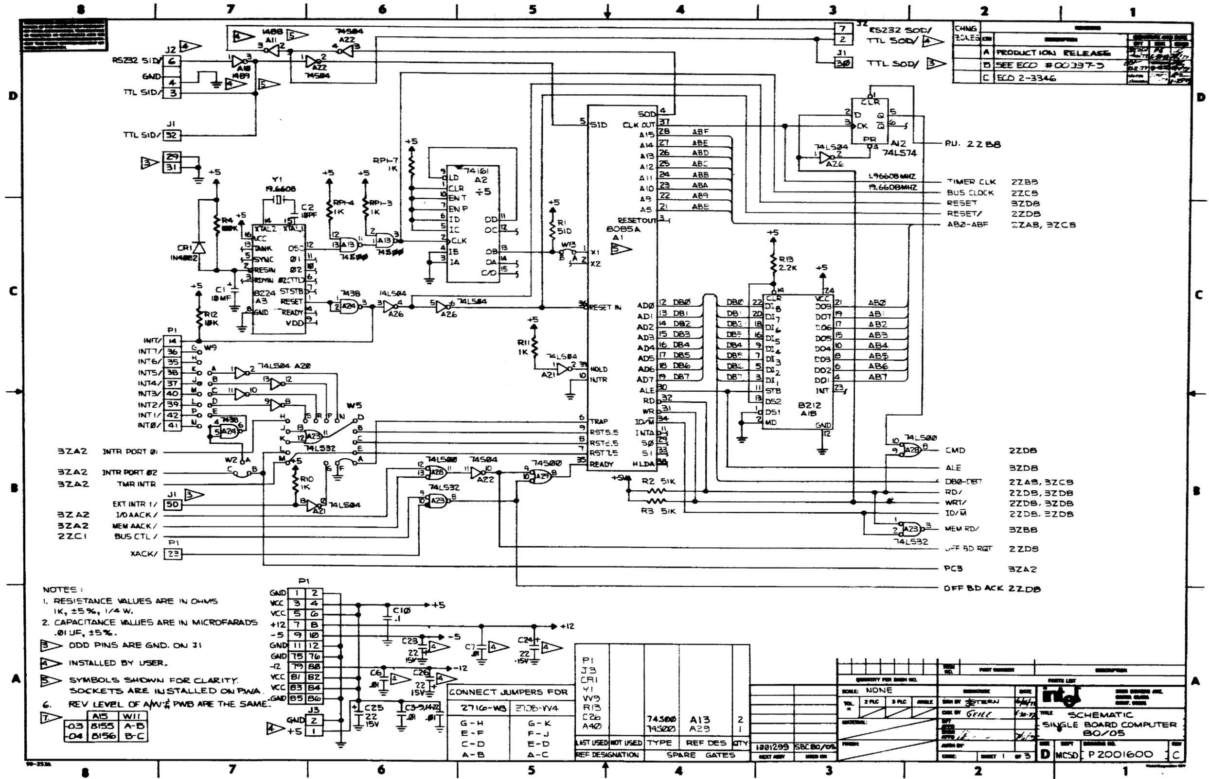
Figure 5-2. SBC 80/05 Schematic Diagram (Sheet 1 of 3)
