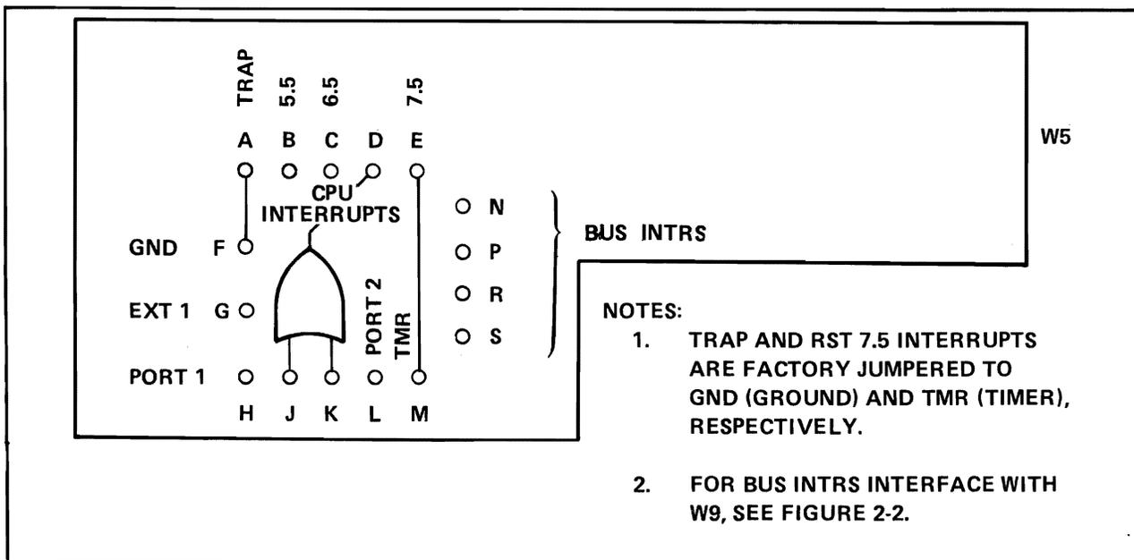
Figure 2-1. CPU Interrupt Input Jumpers
