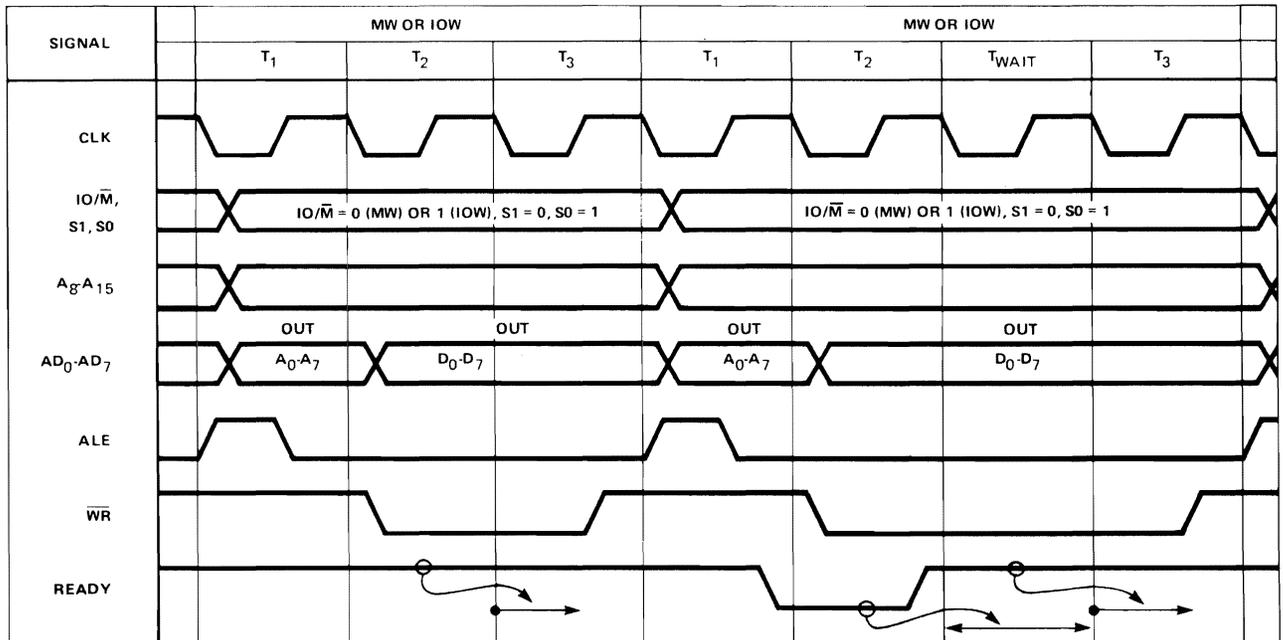
Figure 4-6. Memory Write (or I/O Write) Machine Cycles
