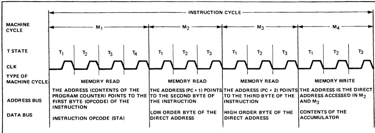
Figure 4-2. Typical CPU Instruction Cycle
