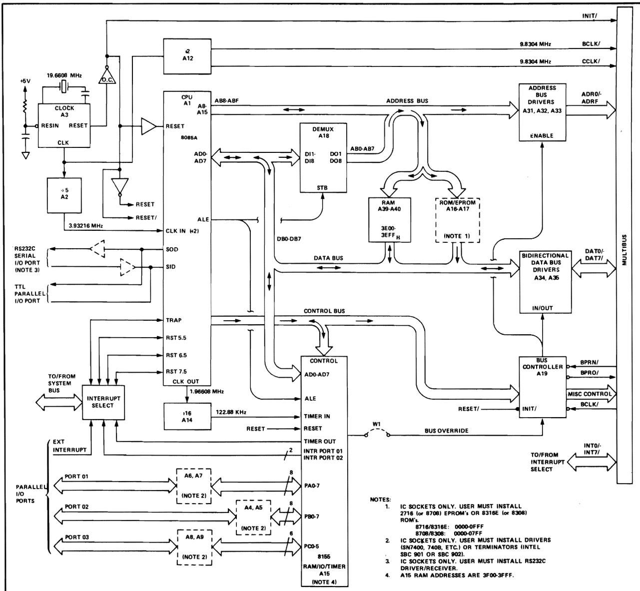
Figure 4-1. SBC 80/05 Block Diagram
