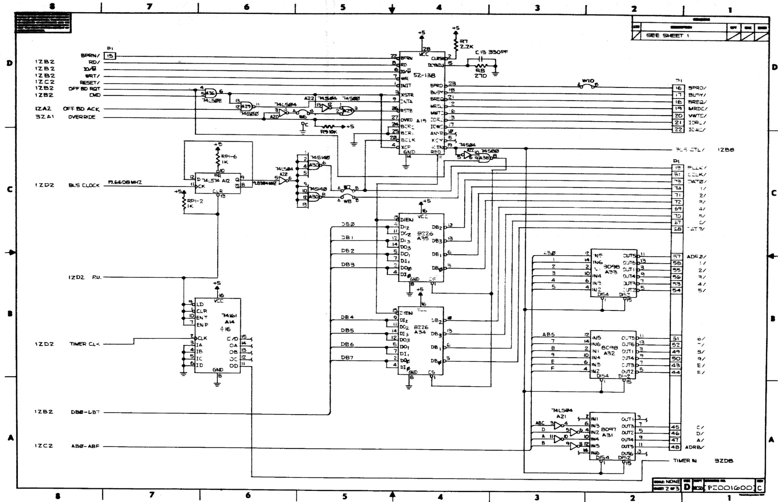
Figure 5-2. SBC 80/05 Schematic Diagram (Sheet 2 of 3)
