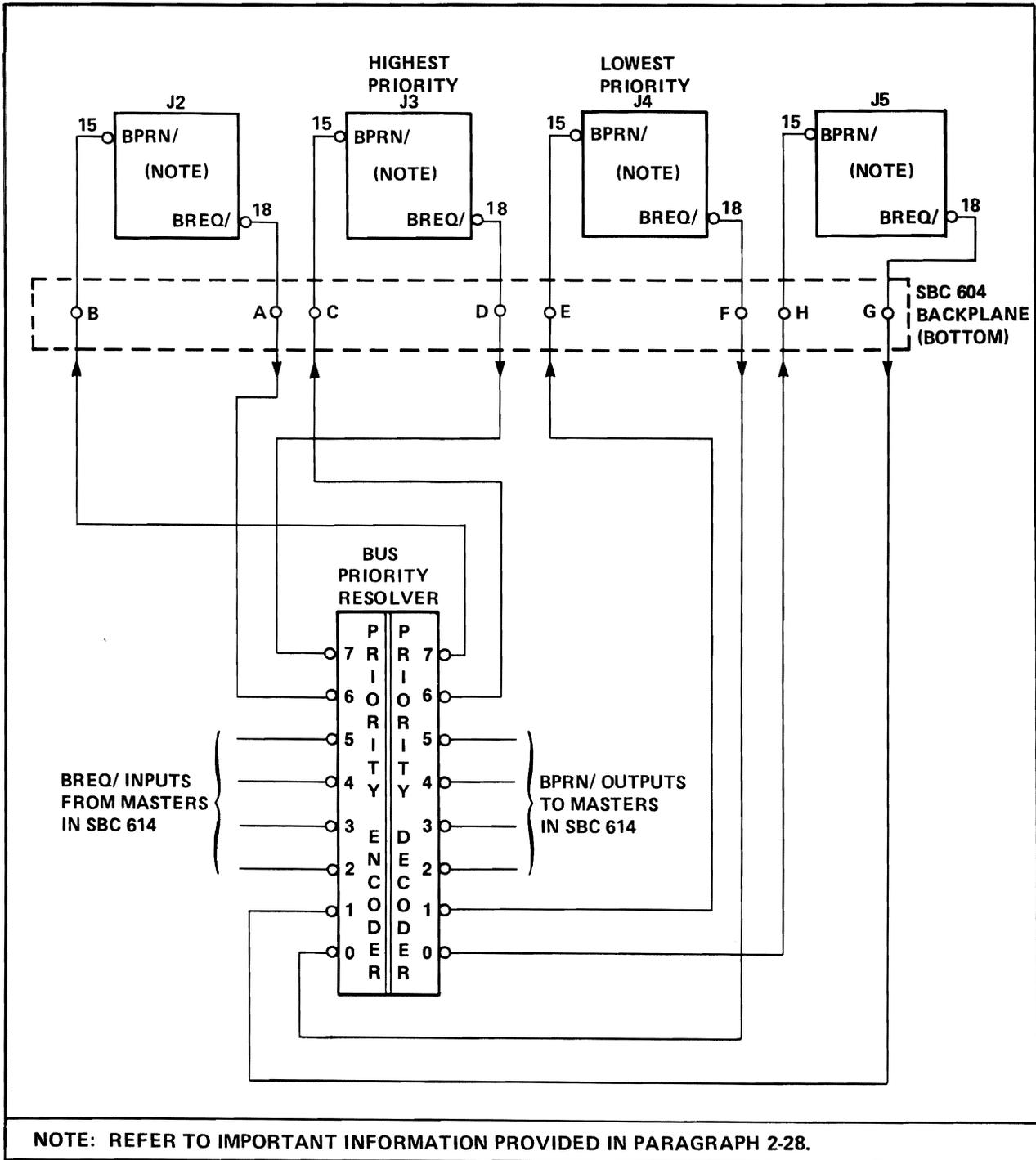
Figure 2-6. Parallel Priority Resolution Scheme
