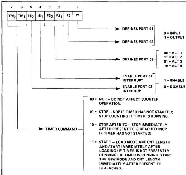
Figure 3-1. Command Register Format (Port 00)
