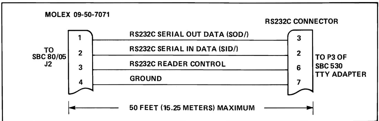
Figure 2-7. RS232C Serial I/O Device Interface Cabling
