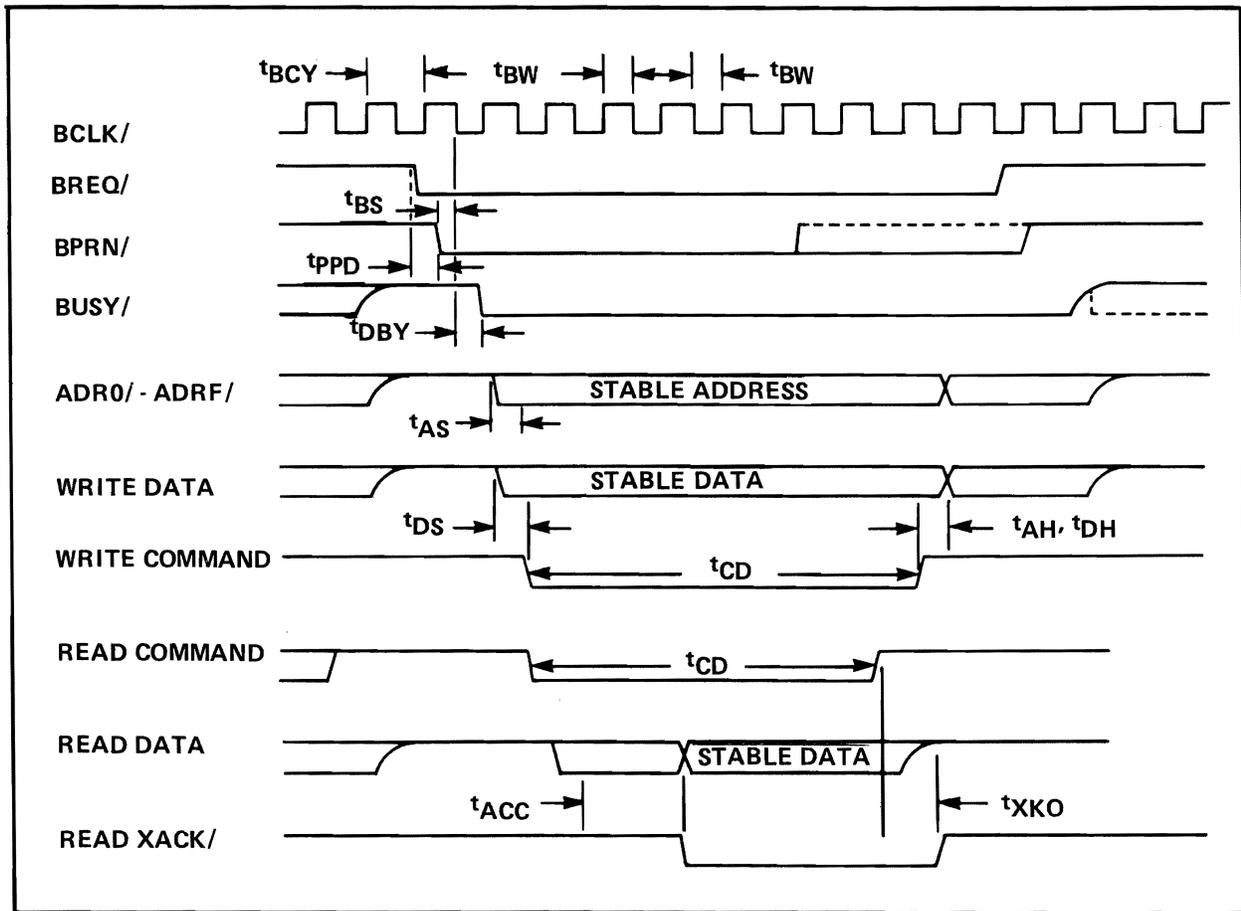
Figure 2-3. SBC 80/05 Bus Exchange Timing
