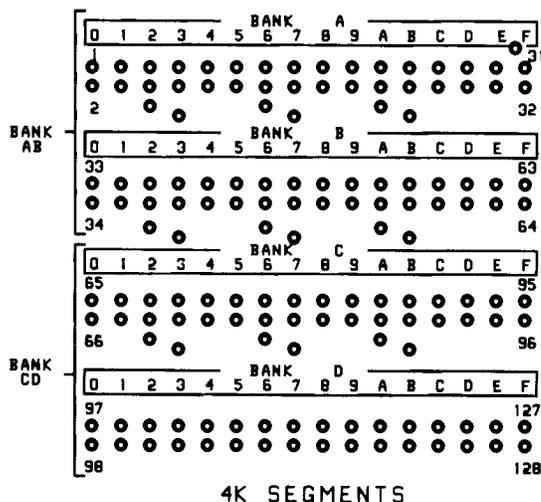
Figure 2-2. Base Address Select Jumpers
