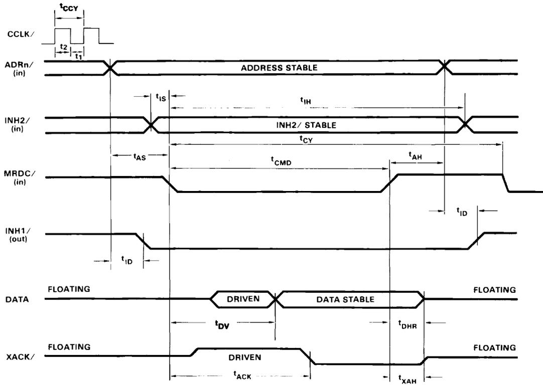
Figure 2-1. Bus Exchange Timing
