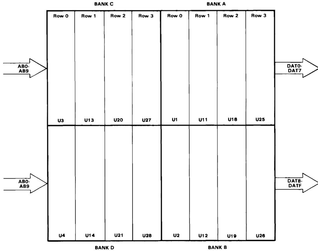
Figure 3-2. Memory Array Functional Layout
