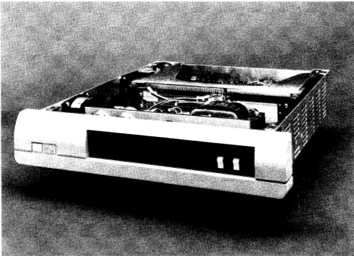
Figure 1-1. iSBC 655 System Chassis
