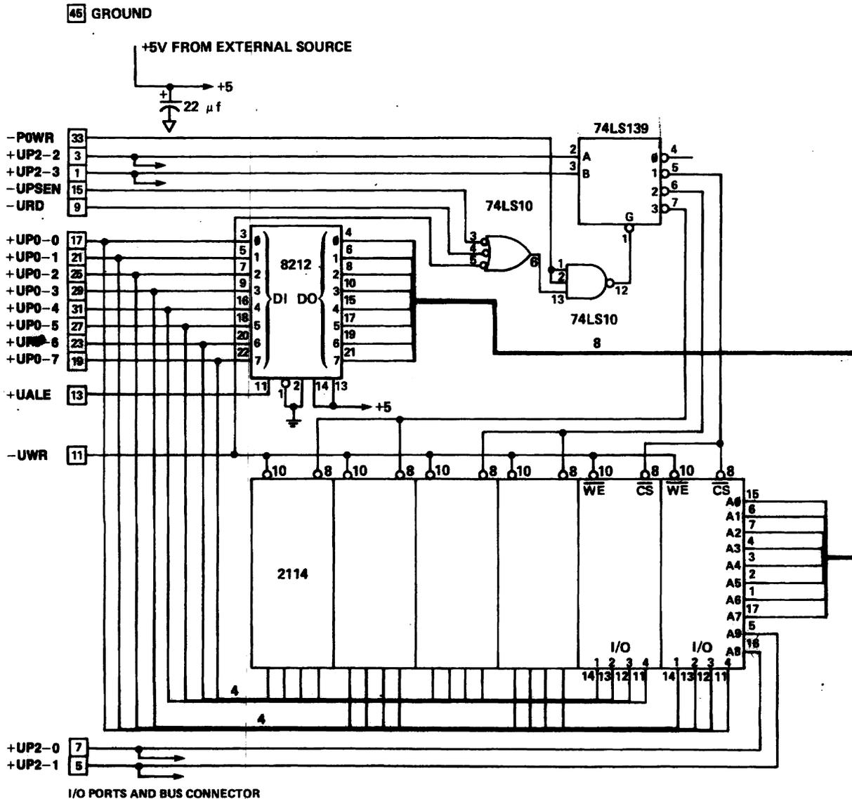
Figure 6-2. Design for "von Neumann" Expansion Memory
