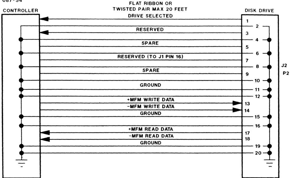
Figure 4-2 27-160 and 27-161 Disk Drive Data Signals
