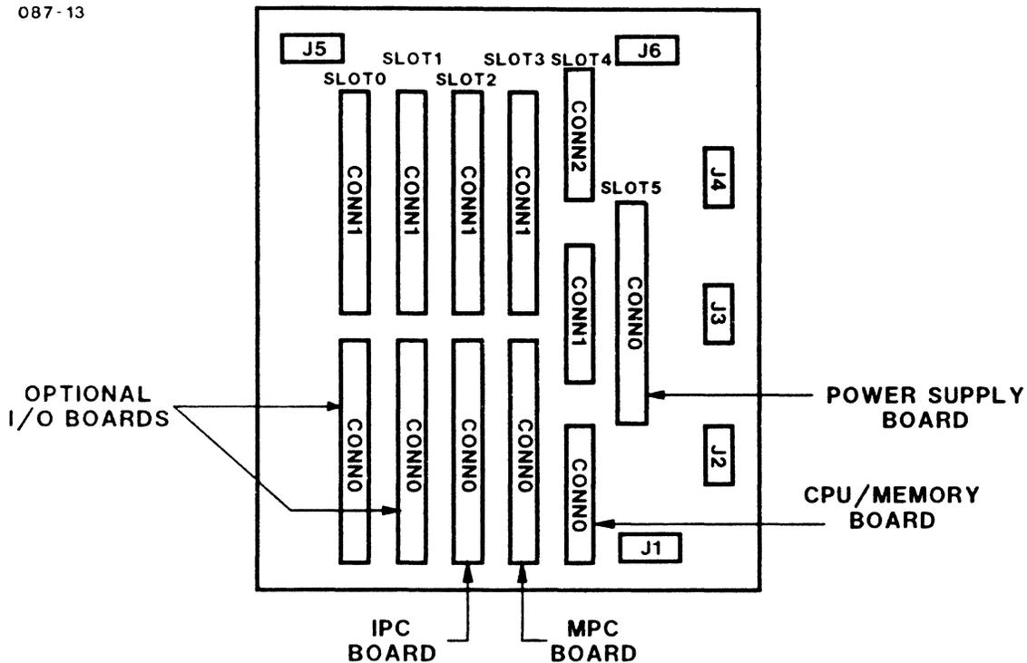
Figure 3-1 Model 3203 Backpanel Layout
