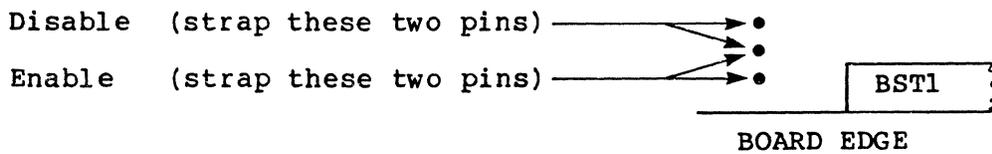
Normal Position; Enable. (May have PC in enable position.)
