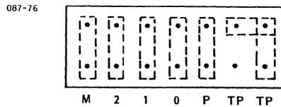
M = Motor Start Option:- Motor starts on command when M is jumpered, otherwise, the disk motor starts on power up. The start on command option is not used in Model 3203 Systems.
