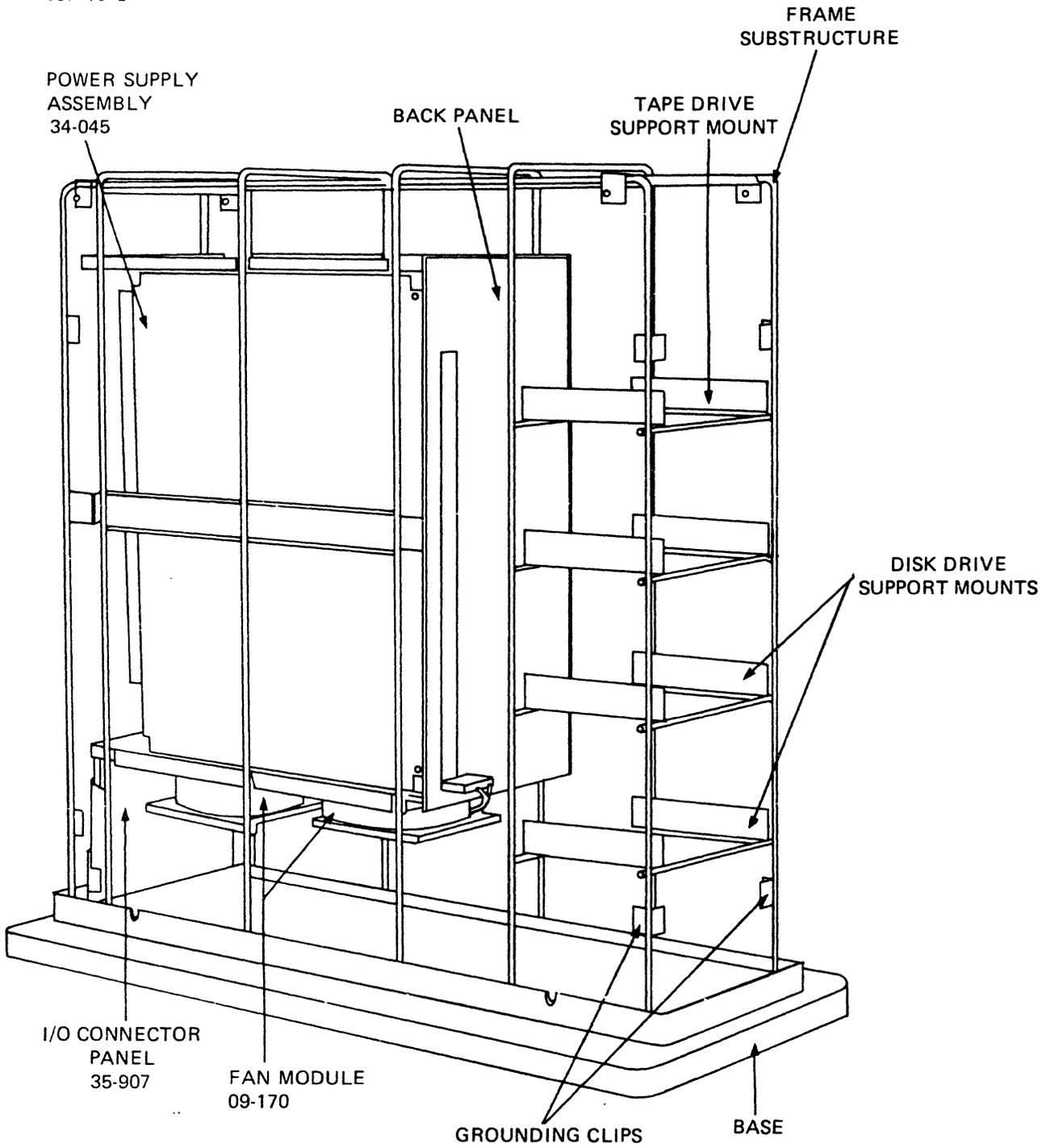
Figure 2-6 Basic System Cabinet (Front View)
