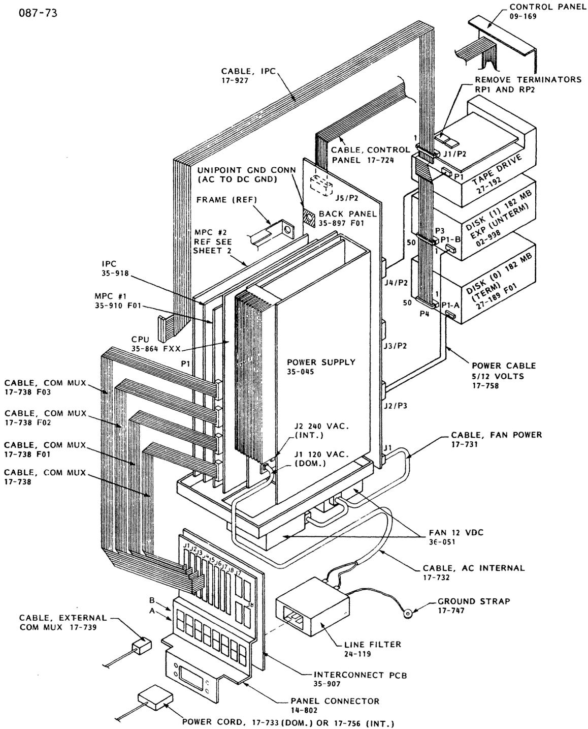
Figure 3-4 01-339 System Cabling Diagram
