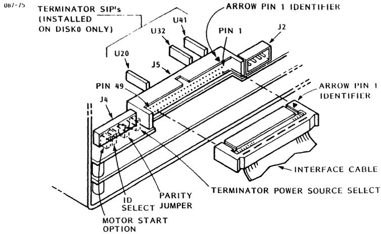
a. Jumper, Terminator and I/O Cable Location/Identification
