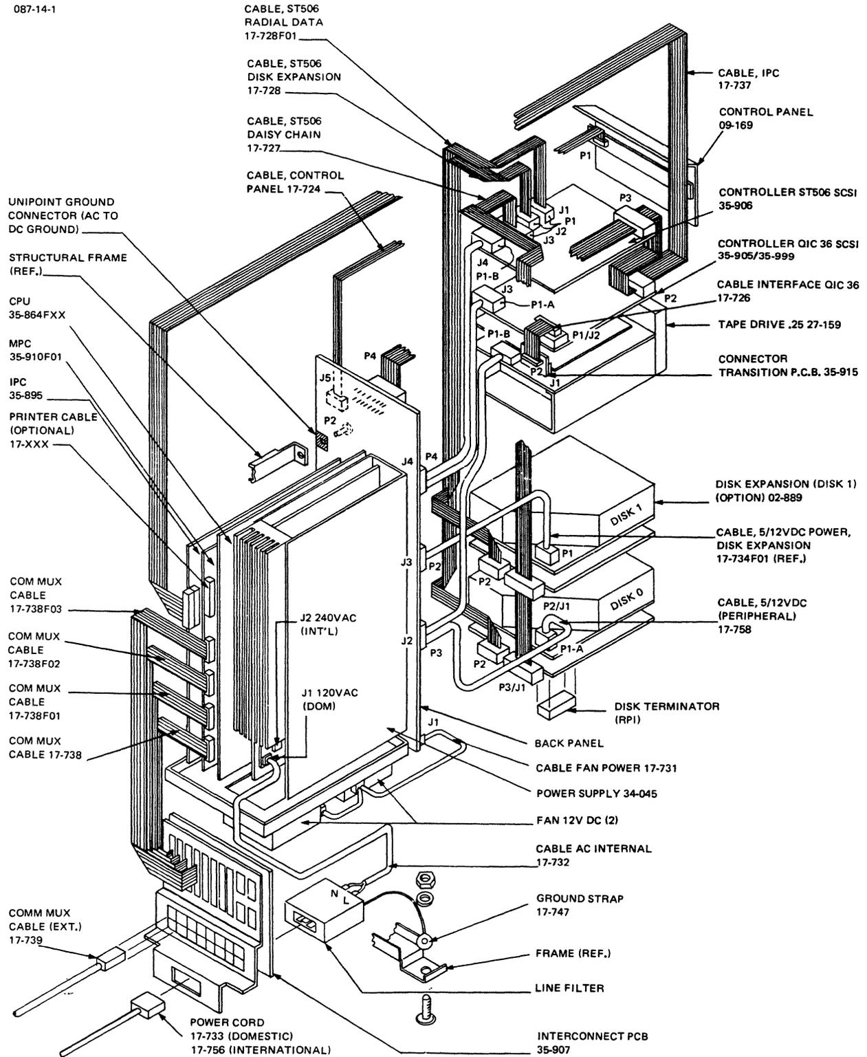
Figure 3-2 01-277 System Cabling Diagram
