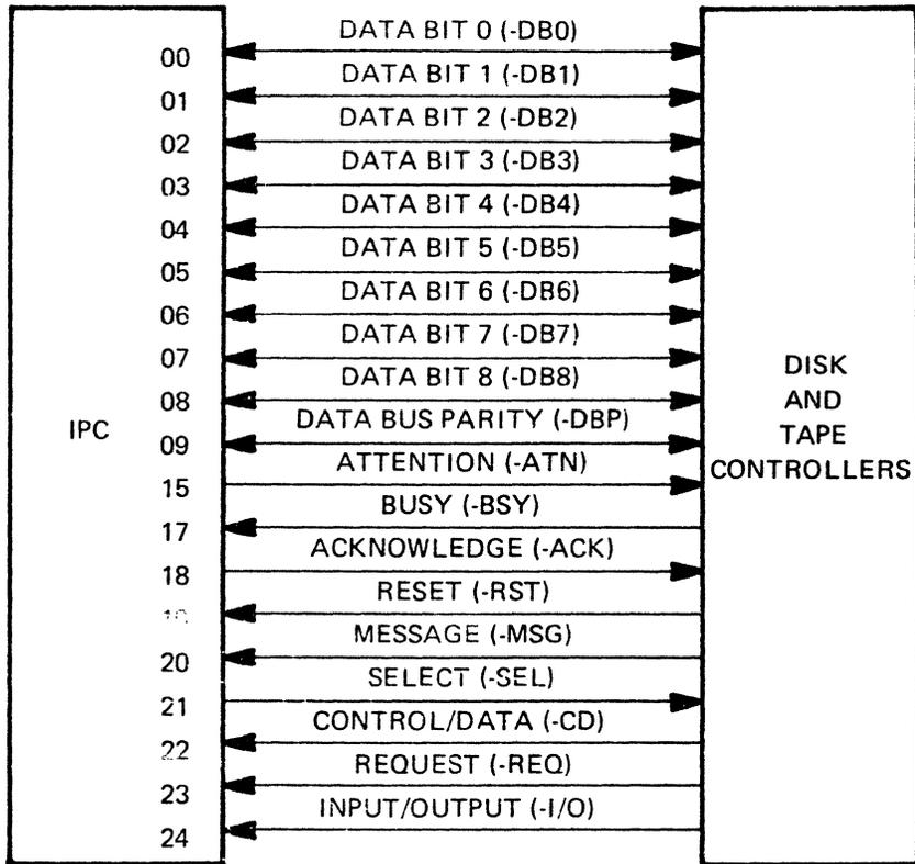
Figure 1-4 SCSI Signal Interface
