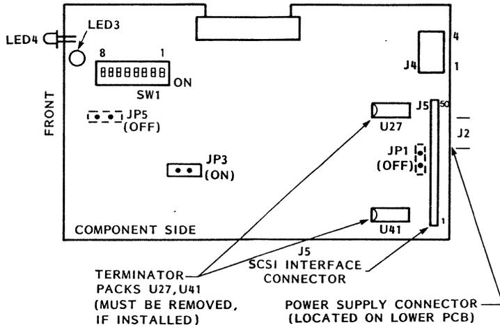
c. Address and Option Switch Setup
