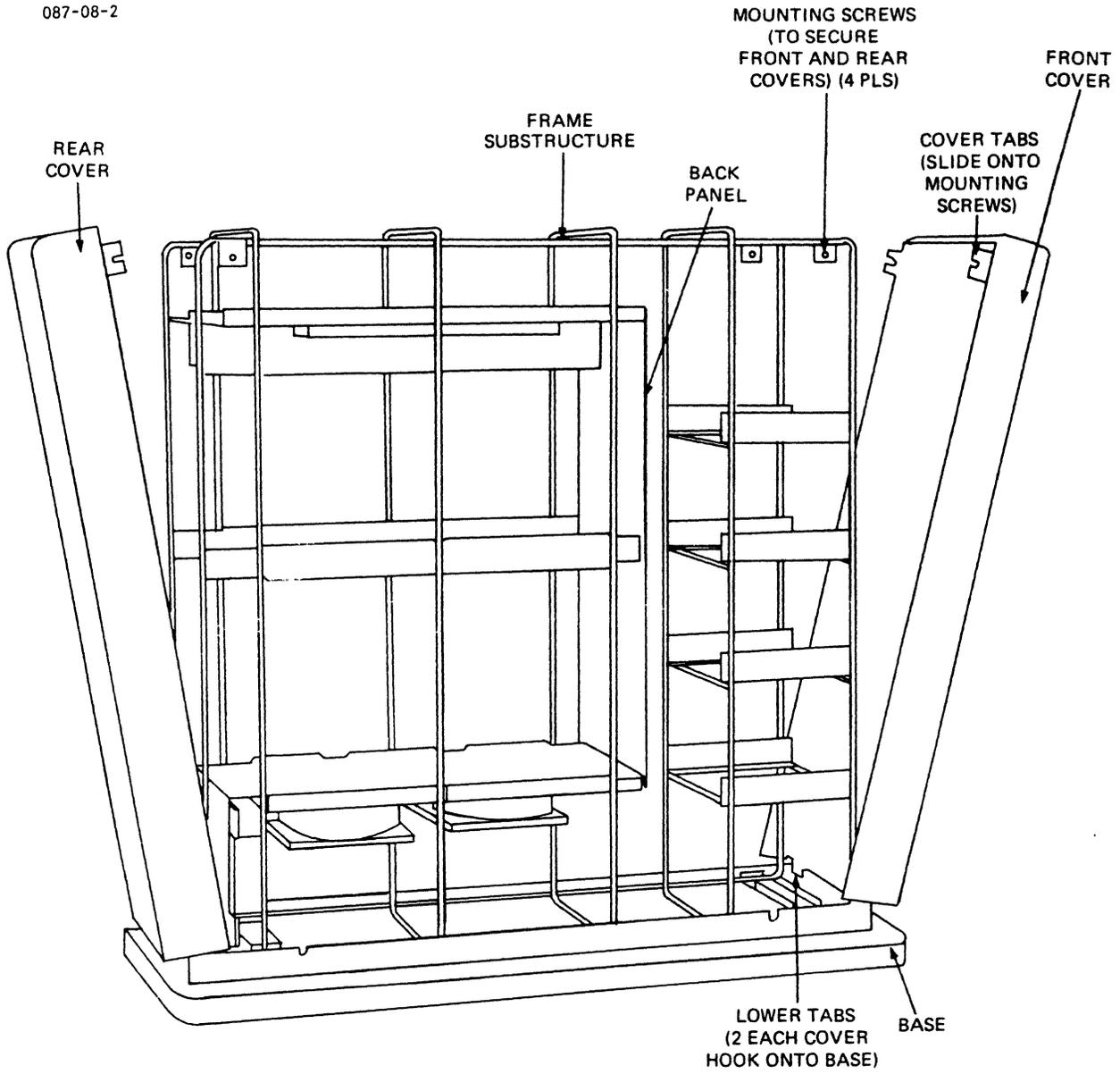
Figure 2-4 Front and Rear Cover Installation
