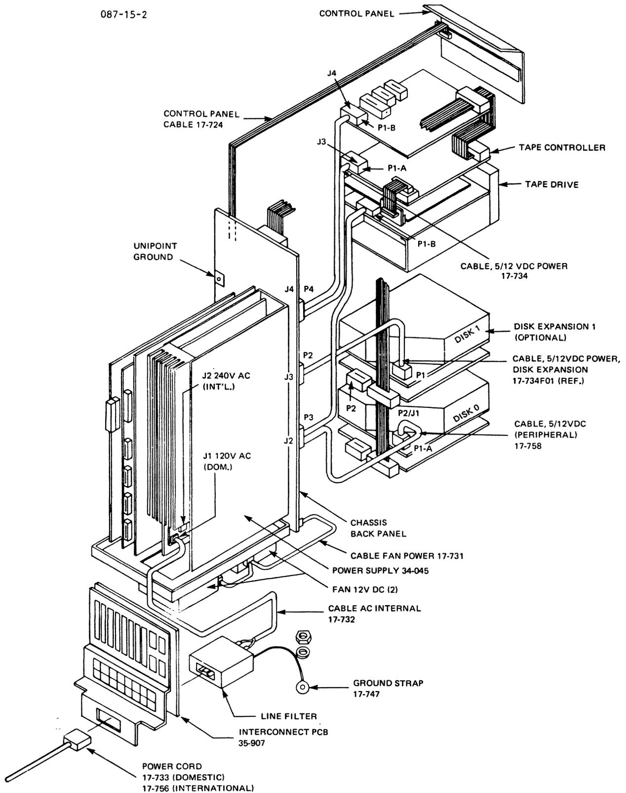
Figure 3-3 01-277 System Power Supply Cabling
