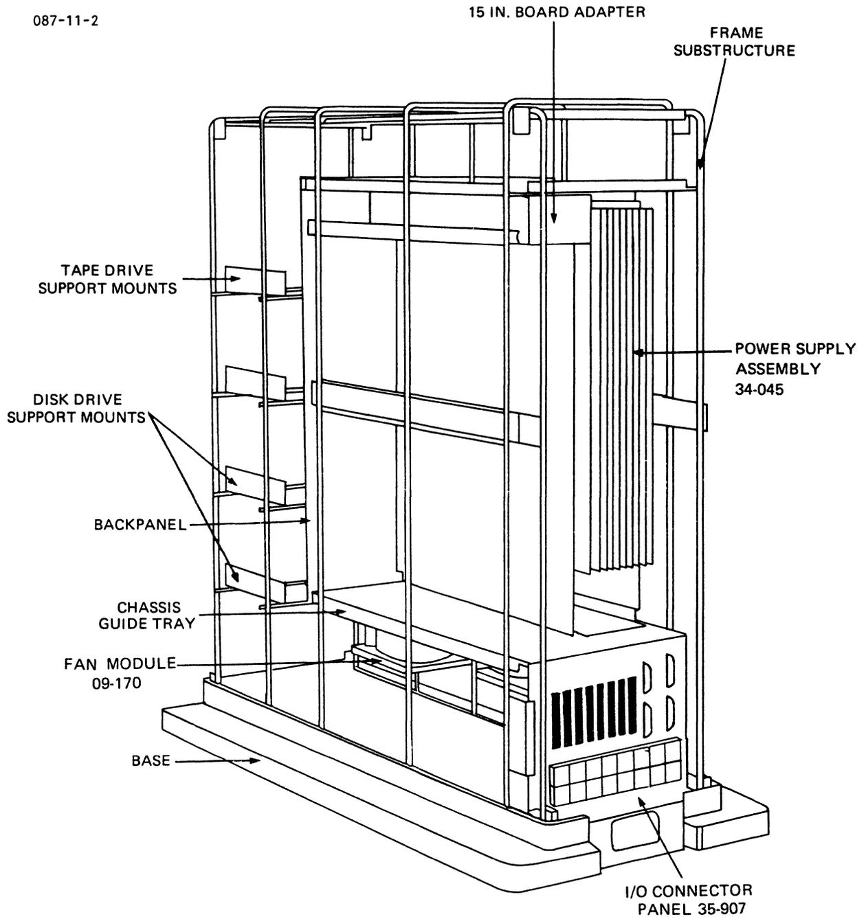
Figure 2-7 Basic System Cabinet (Rear View)
