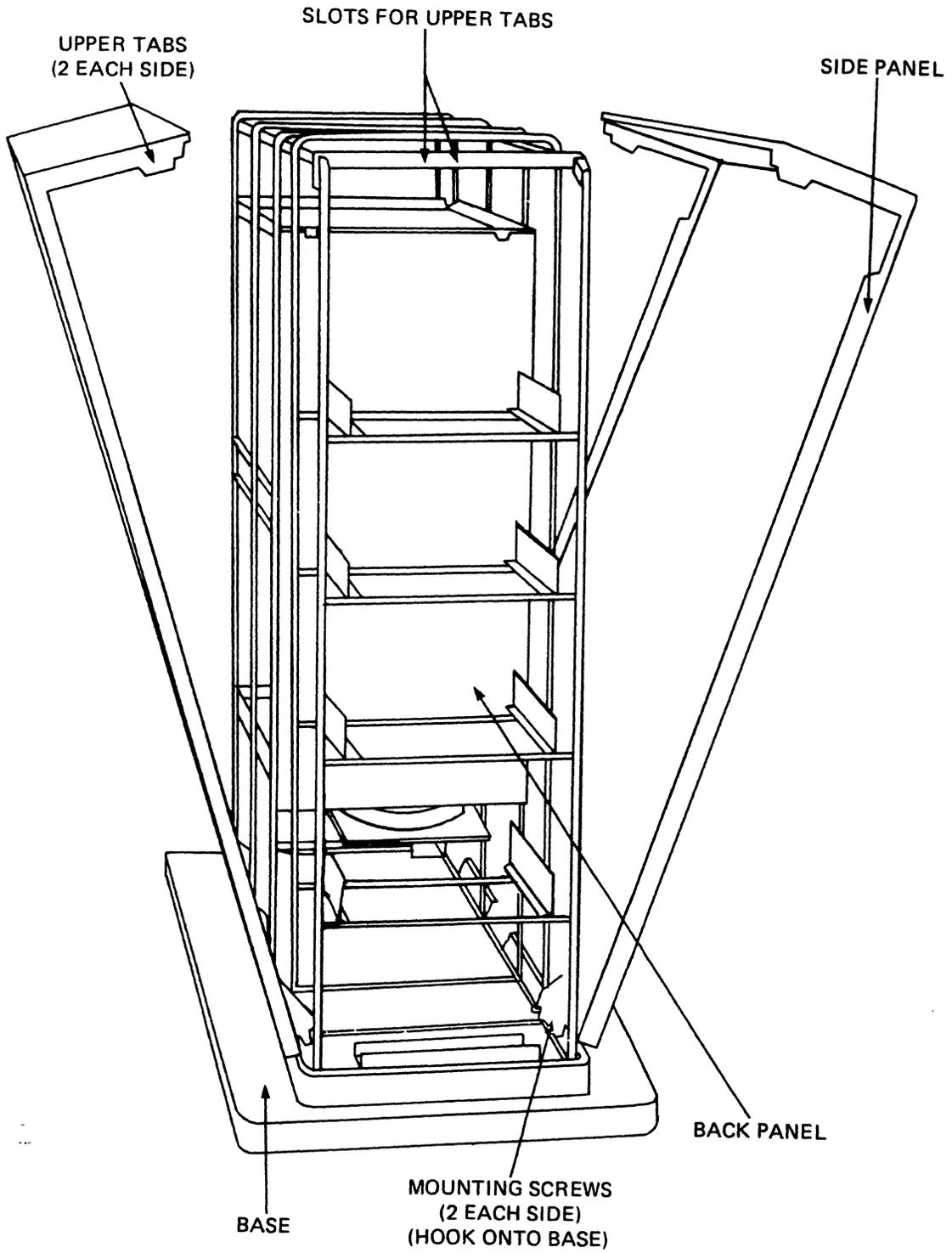
Figure 2-5 Side Panel Installation
