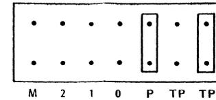
c. Jumper Configuration for Disk 0 (Terminated)
