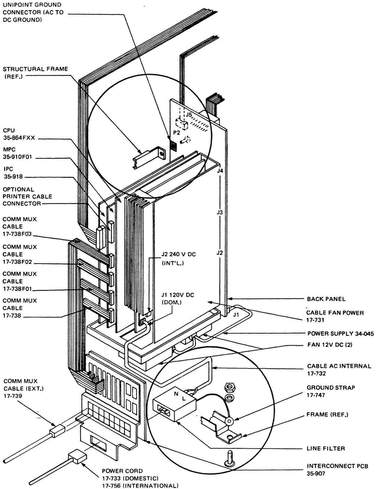
Figure 2-1 System Grounding
