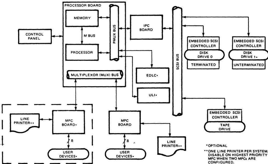
b. Type 01-339 System With Embedded Tape/Disk Controllers
