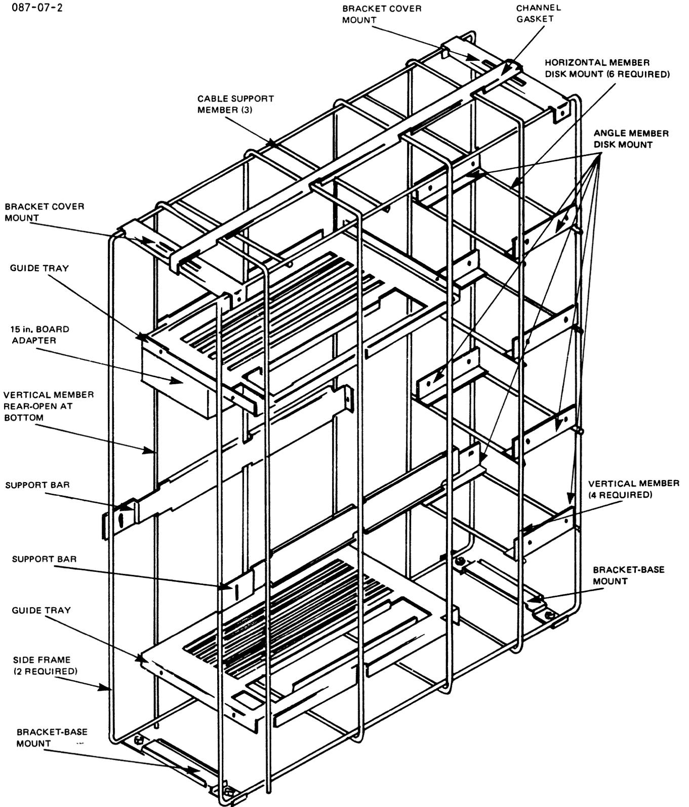
Figure 2-3 Model 3203 Frame Substructure
