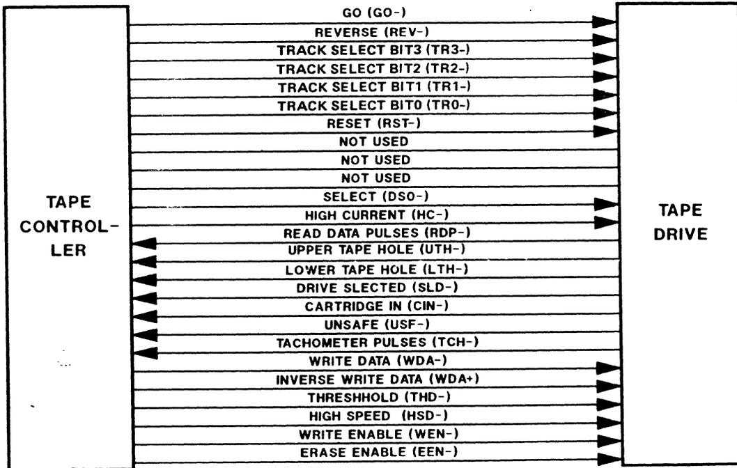
Figure 4-3 Tape Controller/Drive Handshaking Signals
