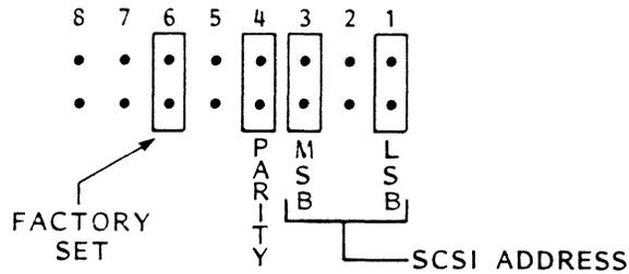
The normal address for this device is '5'. Strap pins 1 and 3 (binary) using the jumpers provided with the board or using wire wrap.
