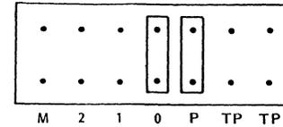
d. Jumper Configuration for Disk 1 (Unterminated)
