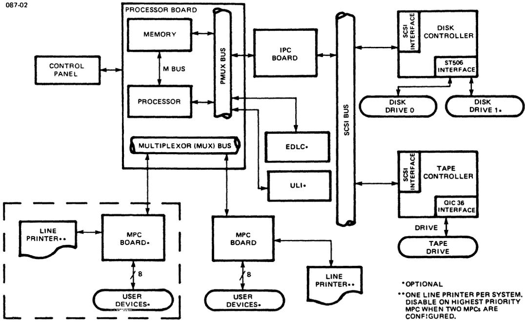
a. Type 01-277 System With Controllers External to Tape/Disk Drives
