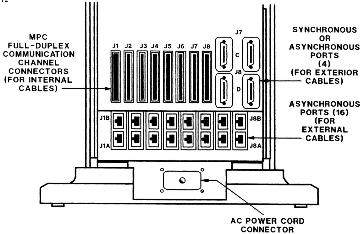
Figure 2-8 I/O Connector Panel (35-907)
