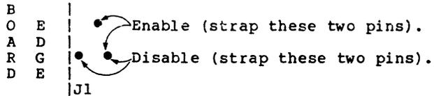
Normal Position: Enable. (May have PC in enable position.)
