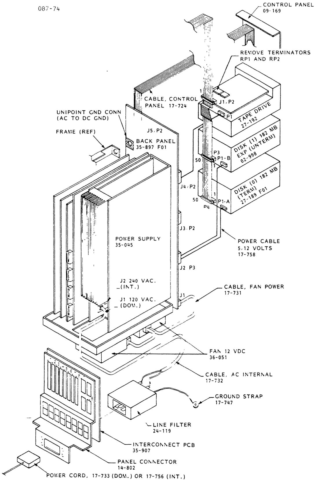
Figure 3-5 01-339 System Power Supply Cabling
