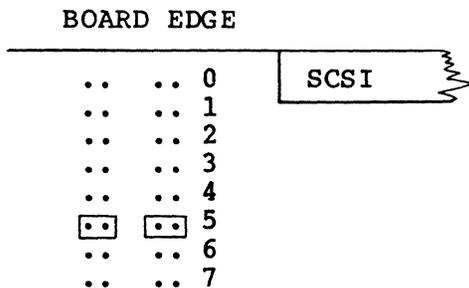
Normal Position: Strap both address '5' positions using straps provided with board, or use wire wrap.
