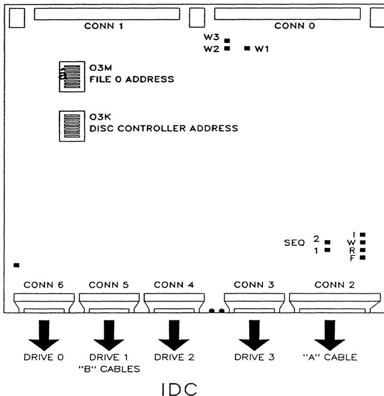
CONTROLLER ADDRESS. Open=1, Closed=0. Example: All open except switch 6 - x'FB.
