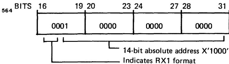
No indexing is specified; therefore, the second operand address is X'1000'.
