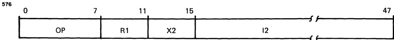
This is a 48-bit instruction format. Bits 0:7 contain the operation code; bits 8:11 contain the R1 specification; bits 12:15 contain the X2 specification; and bits 16:47 contain the 32-bit immediate value, I2.
