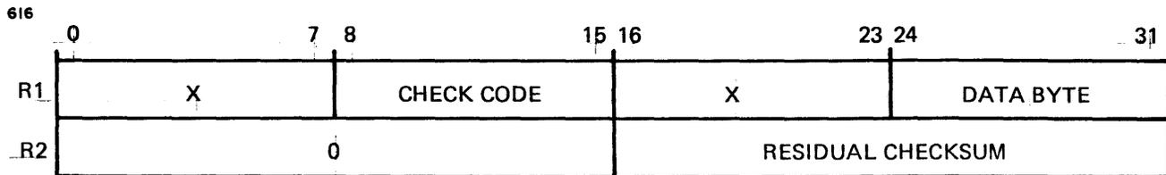
Bits 24:31 of the register specified by R1 contain the data byte to be processed. Bits 8:15 of the register specified by R1 contain a check code indicating the type of processing. This byte is interpreted as follows:
