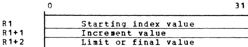
Before execution of this instruction, the register specified by R1 must contain a starting index value. The register specified by R1+1 must contain an increment value. The register specified by R1+2 must contain a comparand (limit or final value). All values may be signed.
