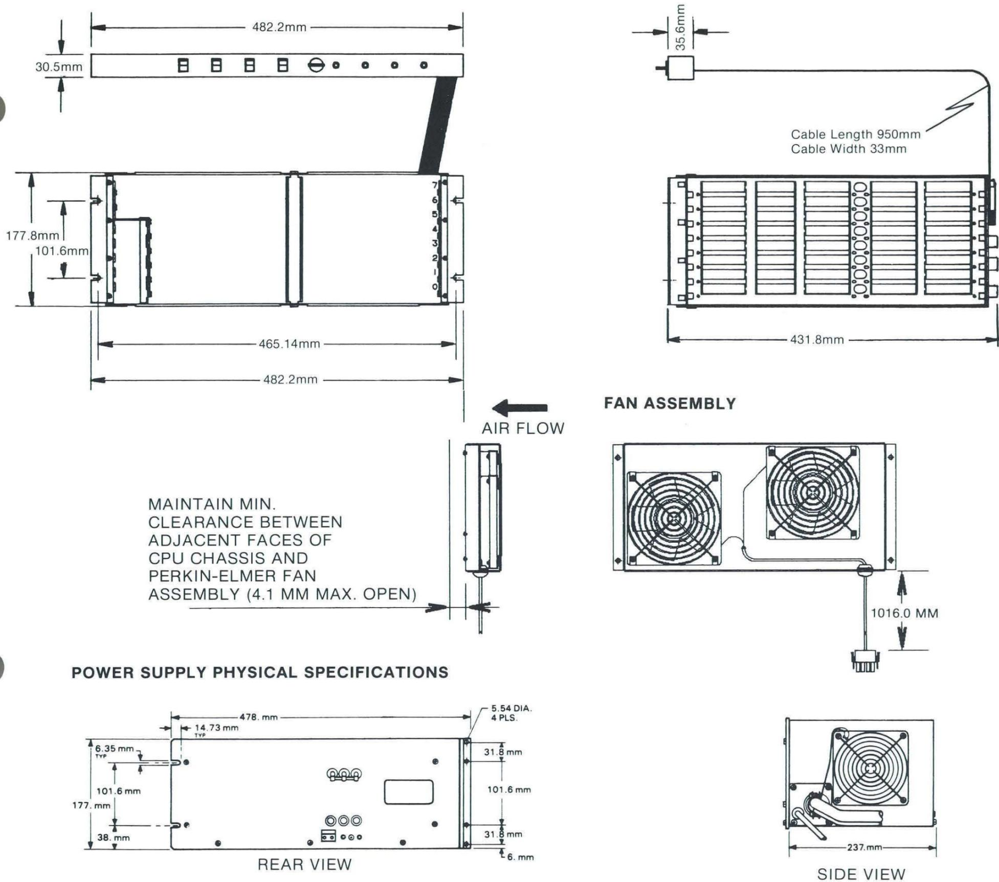
FIGURE 3 — CPU CHASSIS
