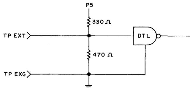
Figure 3. External Oscillator Connections, and Internal Termination
