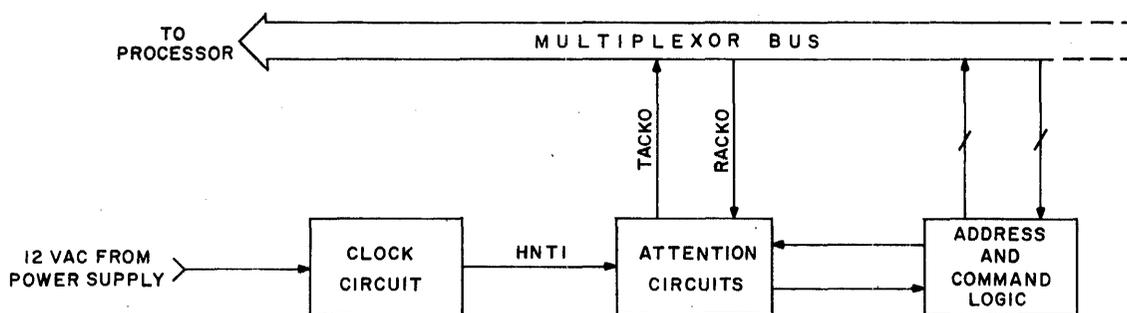
Figure 2. AC Line Derived Clock Block Diagram
