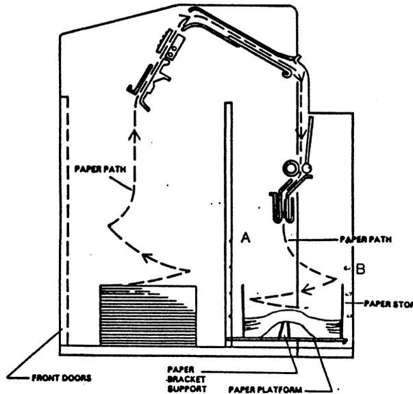
Figure 1-4 Attaching the Paper Bracket Support
