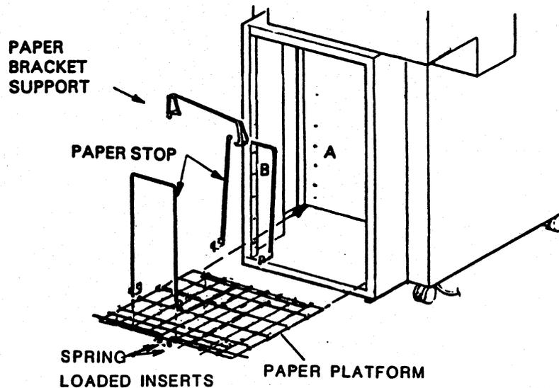
Figure 1-3 Attaching the Paper Platform
