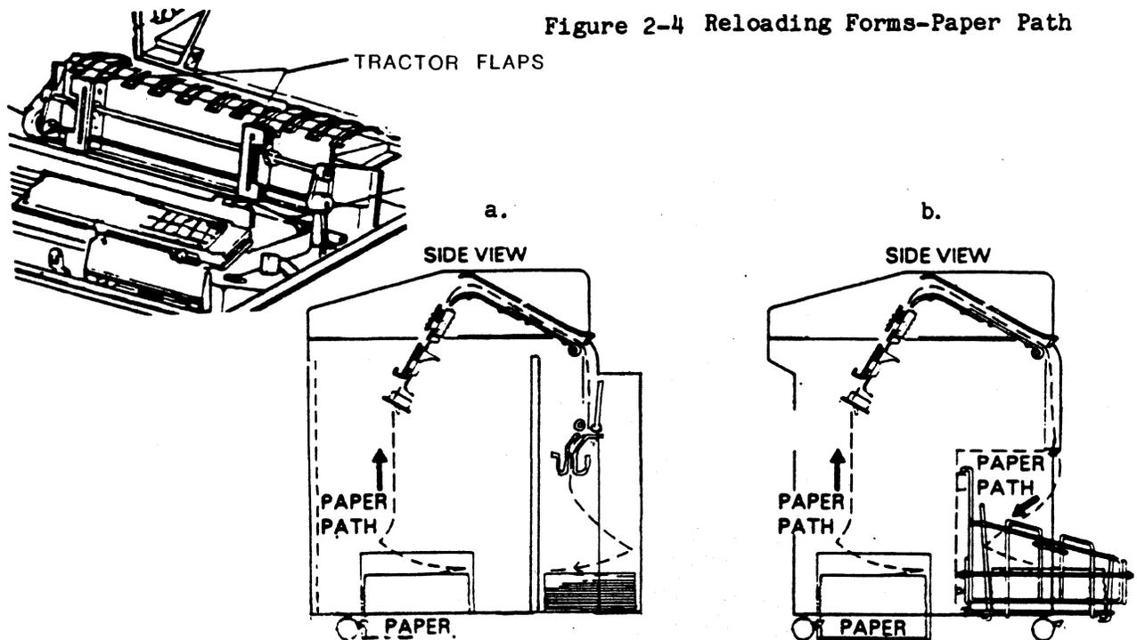
5. Feed paper up through the paper throat, behind the ribbon shield support plate, and onto the paper feed tractor pins. (See Figure 2-4B.)
