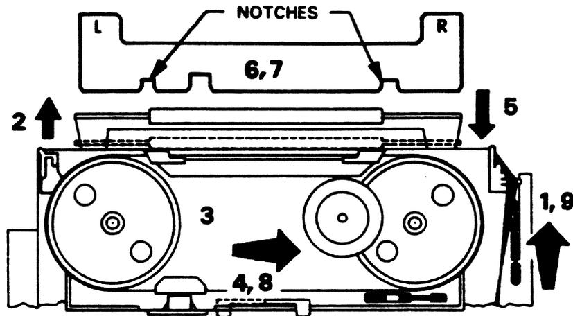
Figure 2-2 Replacing the Ribbon Shield
