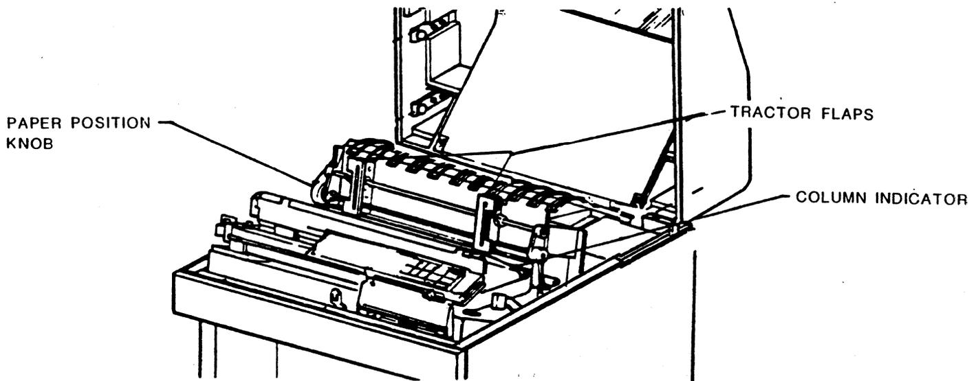
Figure 1-10 Adjusting the Tractor Flaps
