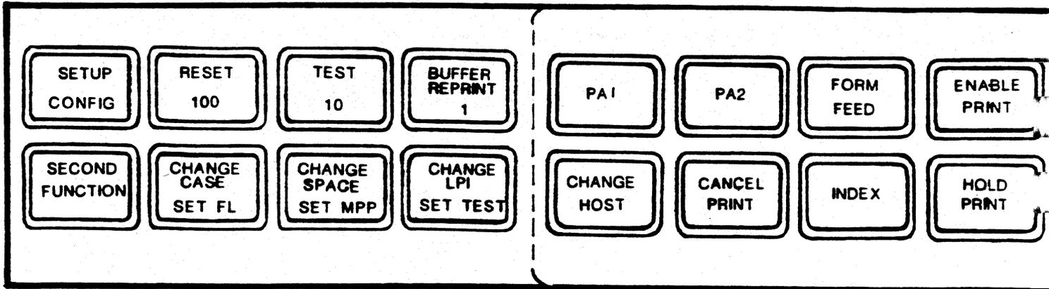
Figure 2-6 Control Panel Keys
