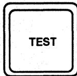
Runs the currently selected test. Some tests which need to perform repeatedly may continue until this key is pressed again. See *"Running Laser 8 Driver Self-Tests"* on page 65 for details. Tests 1-10 are available and can be accessed using the OPTION key function.
