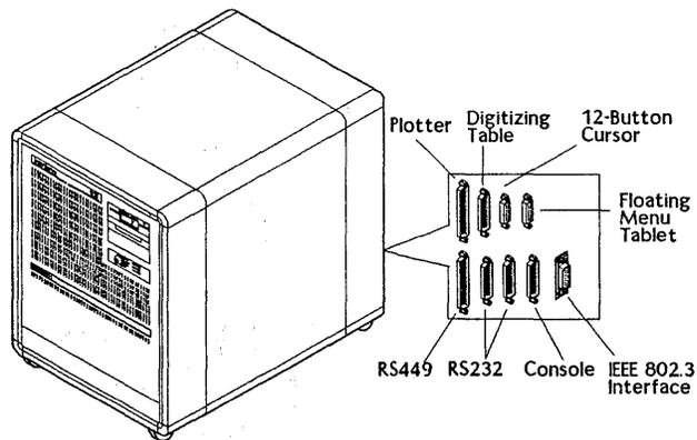
Figure 2-6. Lowboy Electronics Cabinet Ports
