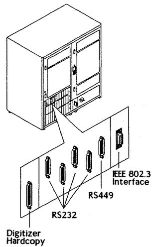
Figure 2-8. Two-Bay Electronics Cabinets Ports
