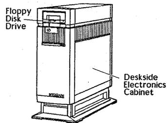
Figure 2-3. Suitcase Electronics Cabinet Main Components
