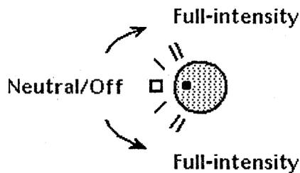
*Figure 1-5. Color Purity Correction Knob Settings*
