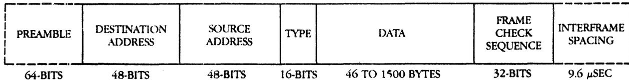
Figure 4-3, Ethernet Frame Format
