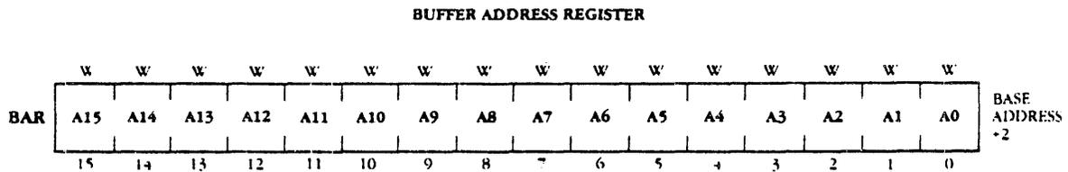
Figure 3-6. Buffer Address Register
