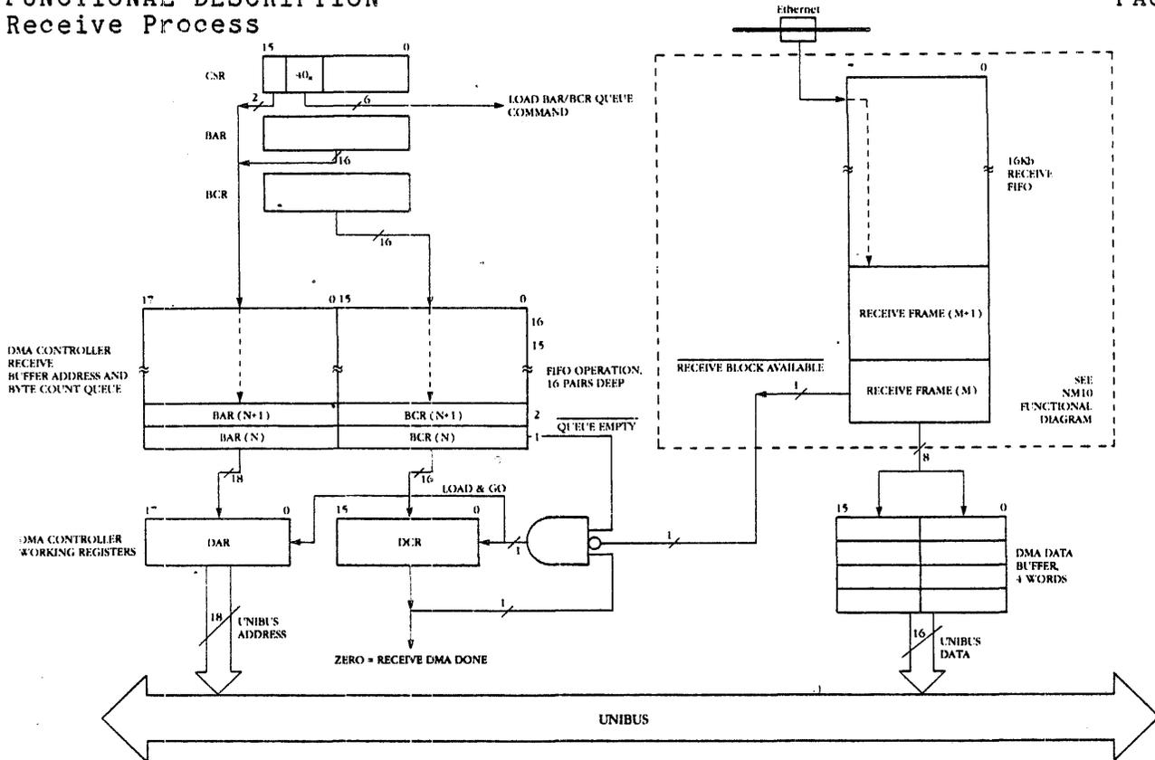
Figure 4-5. Functional Diagram of NI1010A Receive DMA Operation
