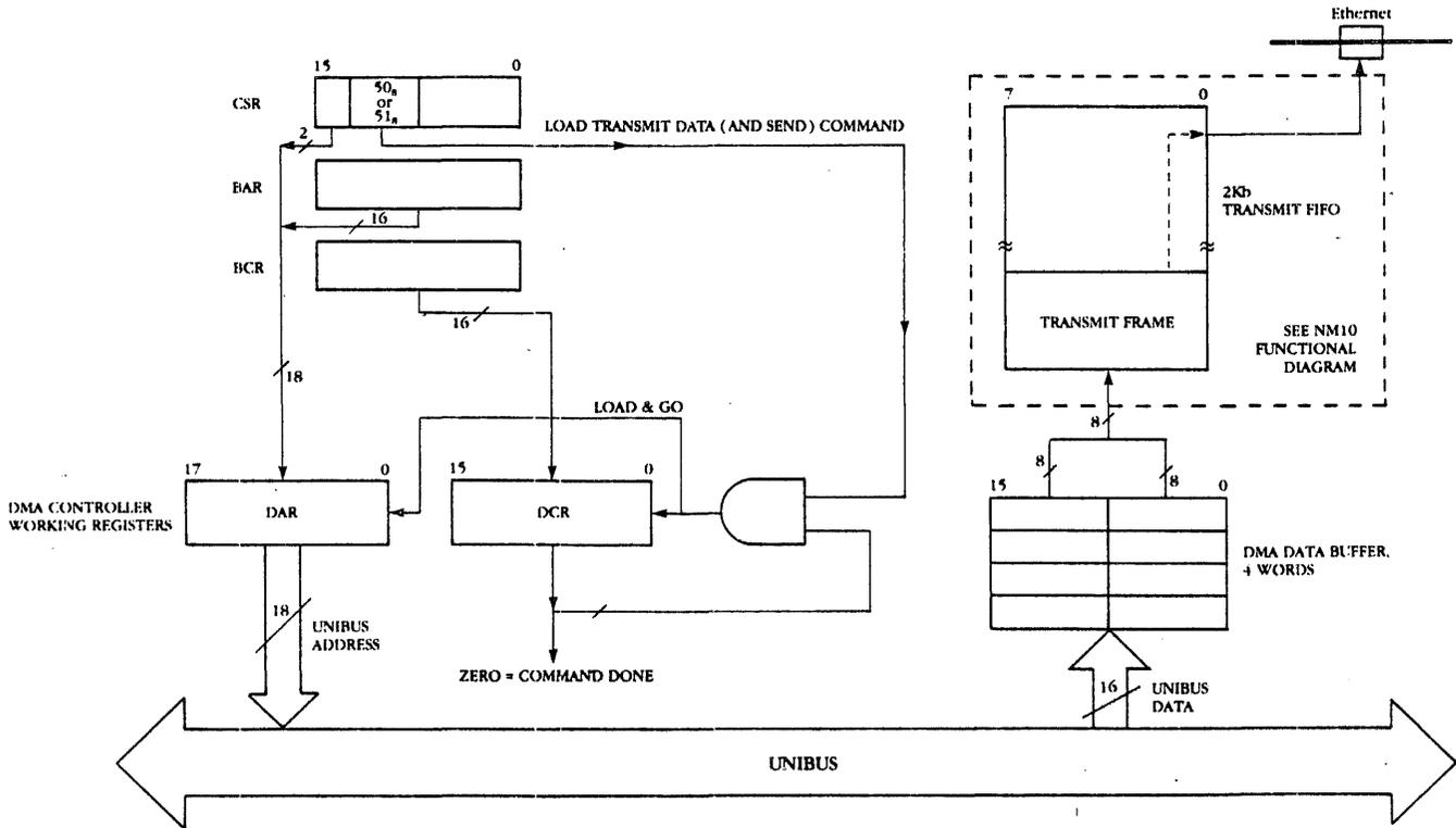
Figure 4-4. Functional Diagram of NI1010A Transmit DMA Operation
