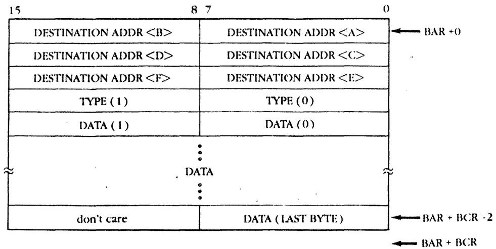
Figure 3-12. Transmit Data Format
