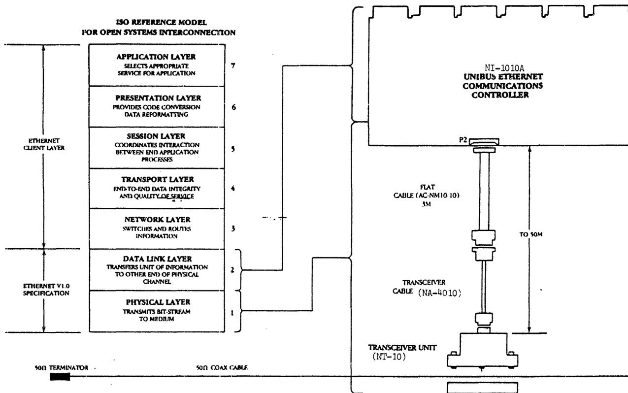
Figure 1-1. Ethernet Architecture and NI1010A Implementation
