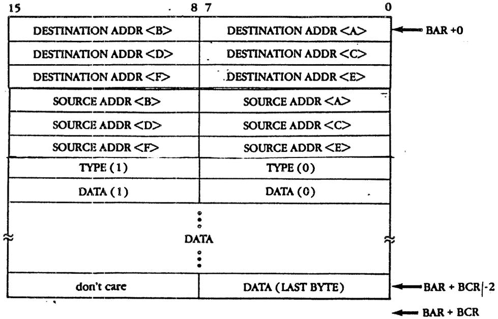
Figure 3-12a. Transmit Data Format
