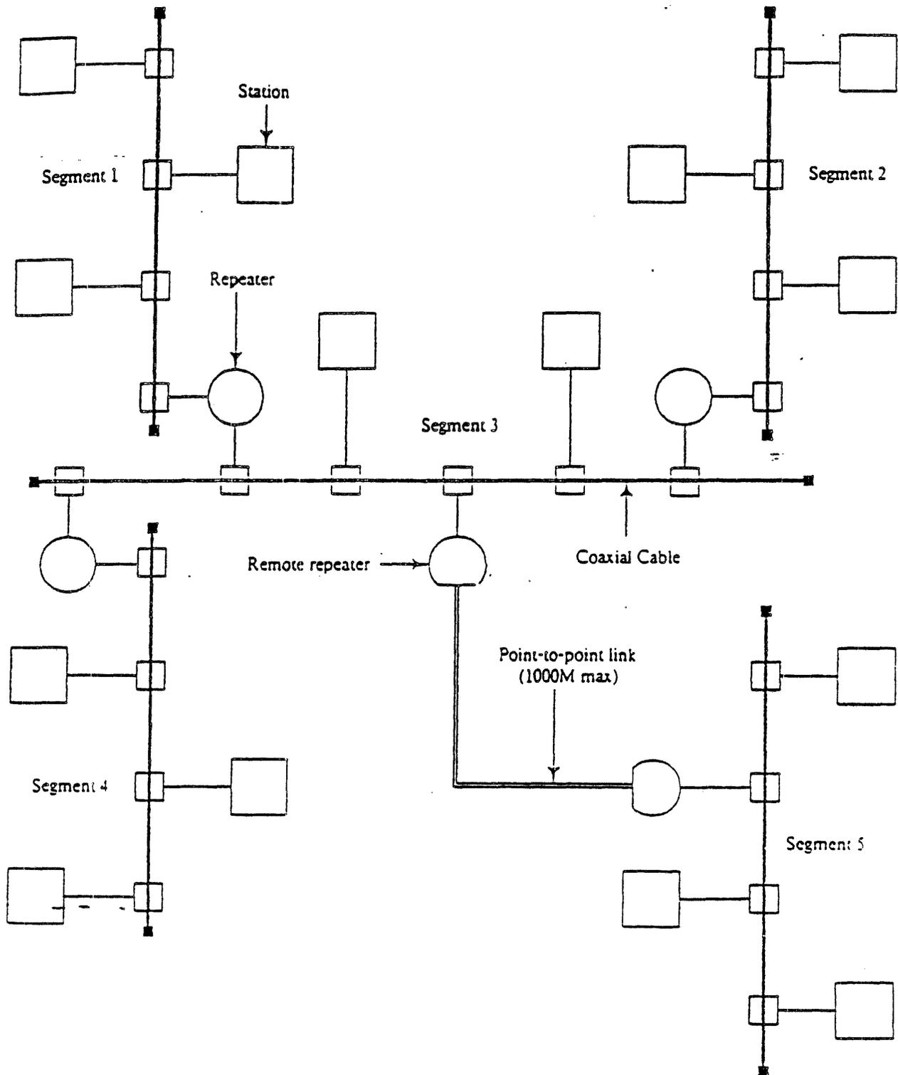
Figure A-1c: A Typical Large-Scale Configuration
