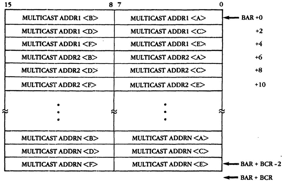
Figure 3-13. Multicast-Group Address Format
