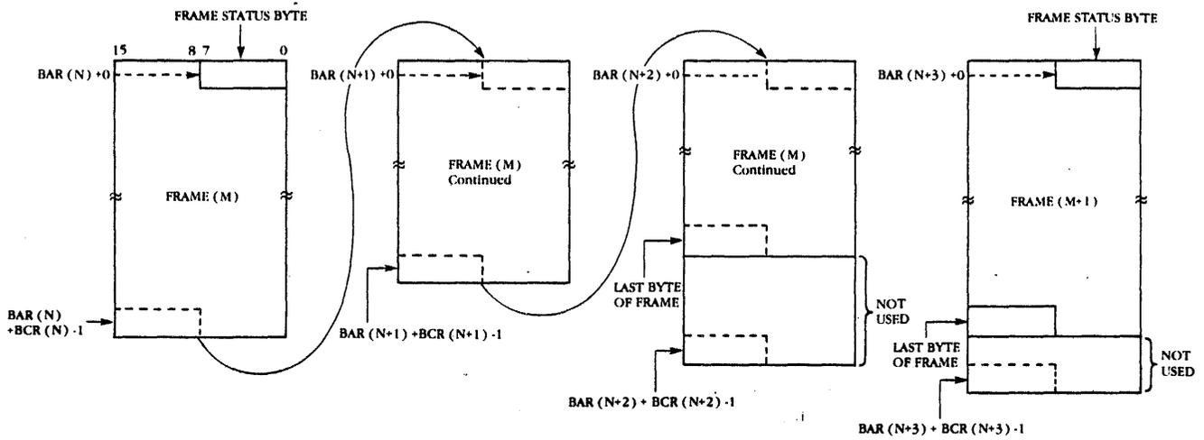
Figure 4-6. Receive DMA Buffer Chaining
