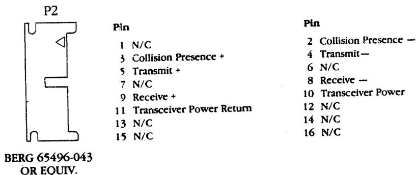
Figure 2-1. NI1010A Transceiver Cable Connector
