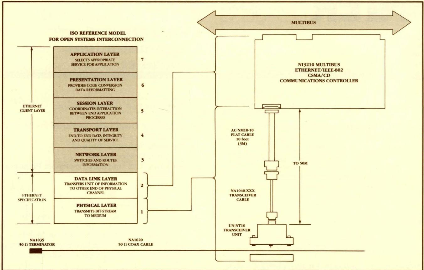
Figure 1. Ethernet Architecture and Implementation
