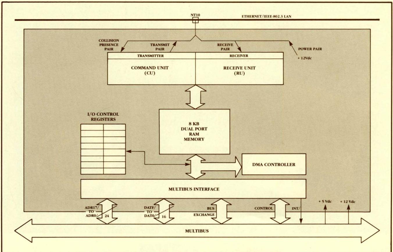
Figure 2. NI3210 Functional Block Diagram
