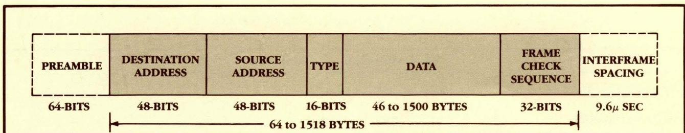
Figure 3. Ethernet Frame Format
