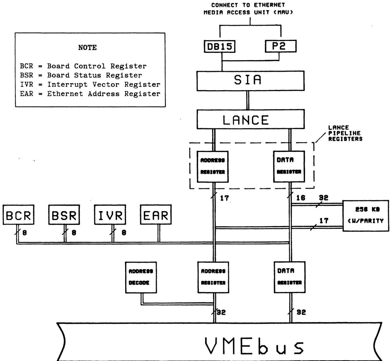
Figure 2. V/Ethernet 3207 Simplified Block Diagram
