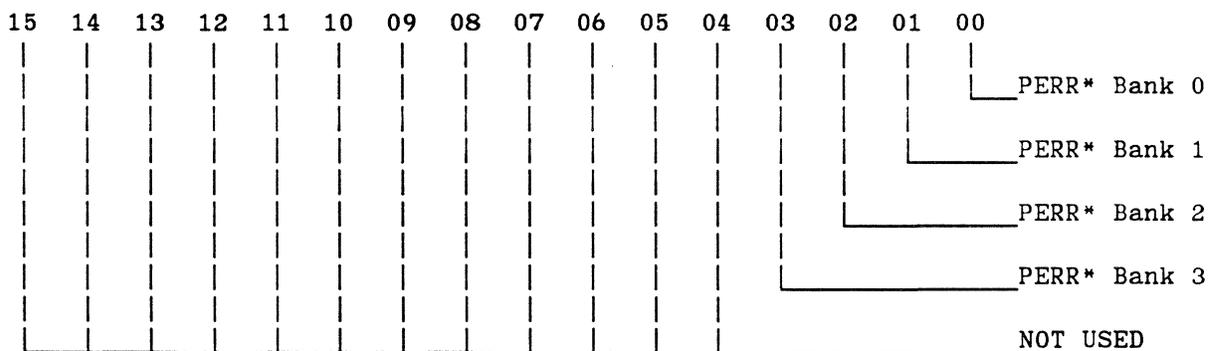
**Figure 4. Board Status Register Format**
