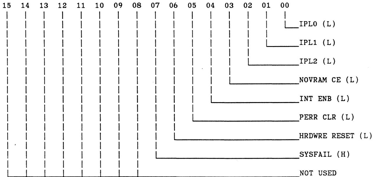
**Figure 3. Board Control Register Format**
