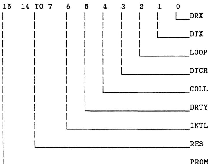
Figure 7. Mode Register Format
