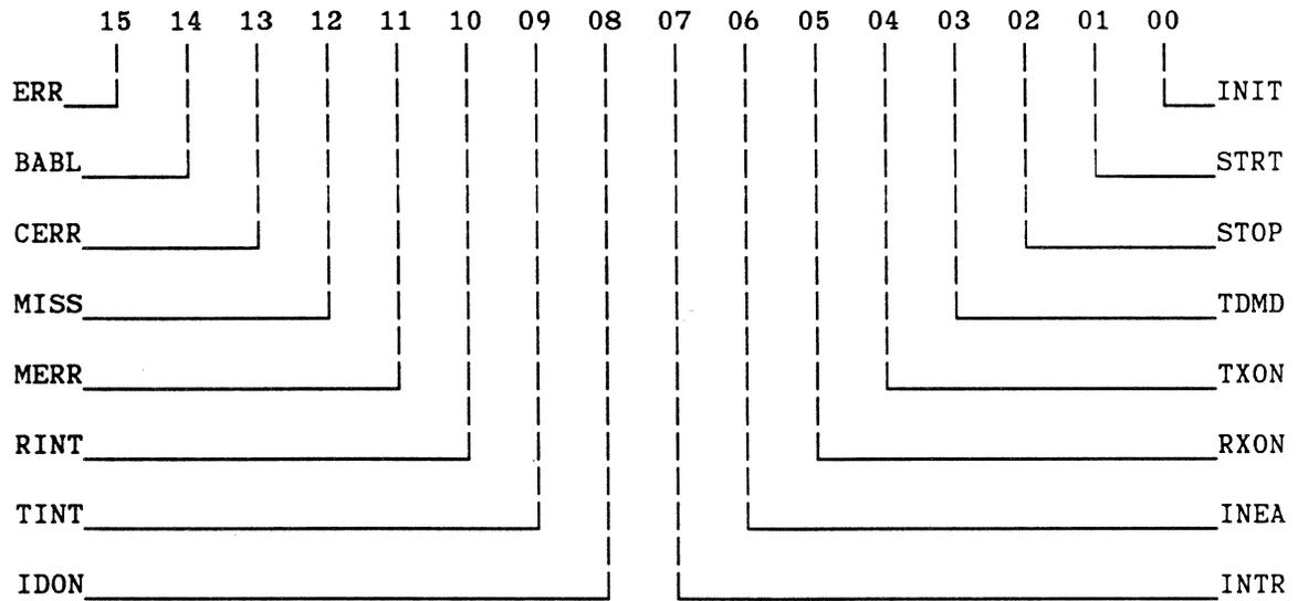
Figure 6. Control Status Register Zero (CSR0)
