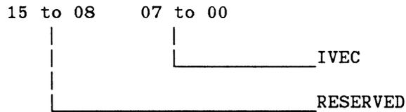
**Figure 5. Interrupt Vector Register Format**
