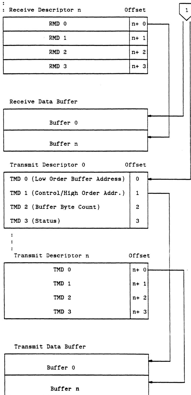
Figure 1. V/Ethernet 3207 Hawk Data Structures (cont.)
