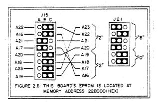
If 24-bit addressing is being used in the system, then J15 must also be set to correspond to address bits A16 through A23. See Figure 2.6.
