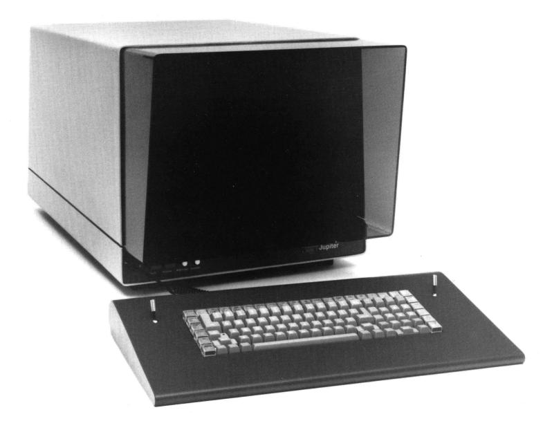
Jupiter 12 is a high resolution, high speed color graphics terminal that can also be used as a stand alone communicating workstation. It is based on the powerful MC68000 processor and has many graphics features available that until now have been found only on systems costing much more.
