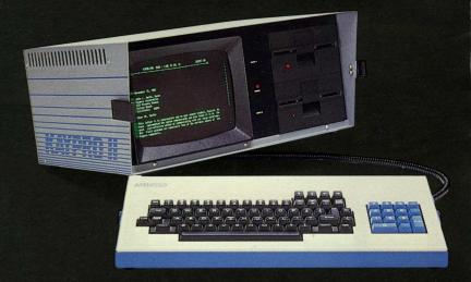
statistical data. Each KAYPRO contains the necessary input/ output connections for communications over the telephone line and utilization of a variety of printers. In short, the KAYPRO computers are designed with the features and reliability to continue working as long as you do.
