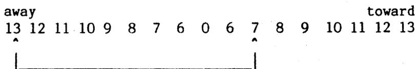
In this example the R/W head is far off track centerline. It may be from 2 to 4 mills outward, away from the spindle. The drive is usable as is, needs to be adjusted to prevent future problems. We are not sure about the size of the error because there is no way to read beyond 13 mills of radial displacement.
