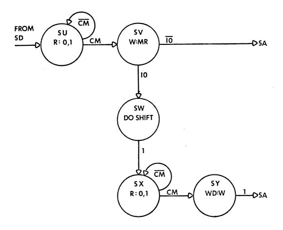
When the computer finishes any instruction, the SA state results. This may be regarded as the start of the next instruction. In state SA, the desired address is 3 which is the address of the P register. Therefore the function of state SA is to locate the P register. If, during T7, the comparison signal, CM, is false, state SA will be regenerated for another byte time. If the comparison signal is true, then the next state will be SB.
