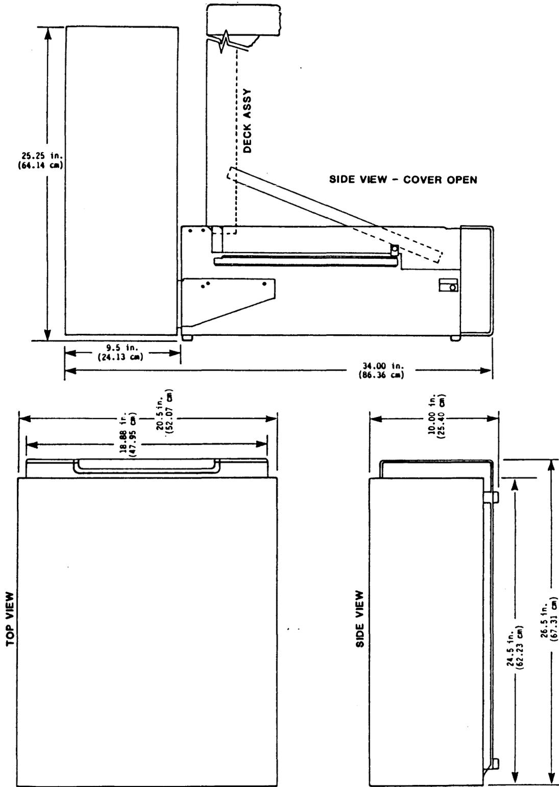
Figure 2-7. Outline and Installation Drawing, Model 9660
