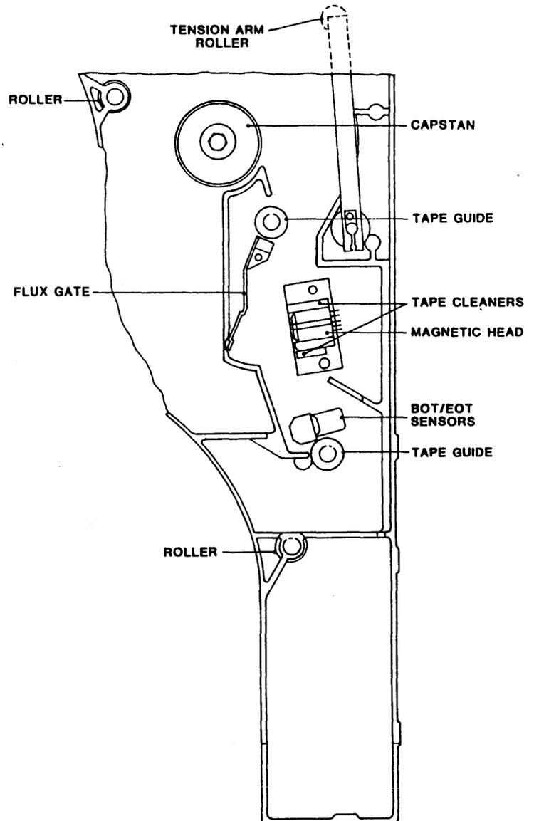
Figure 4-2. Tape Path Cleaning
