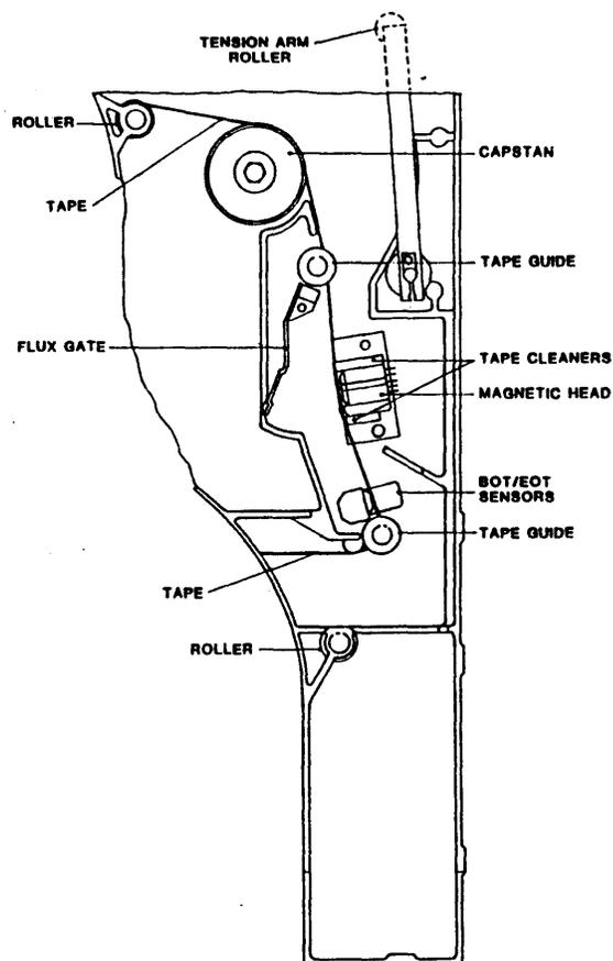
**Figure 2-12. Tape Threading**
