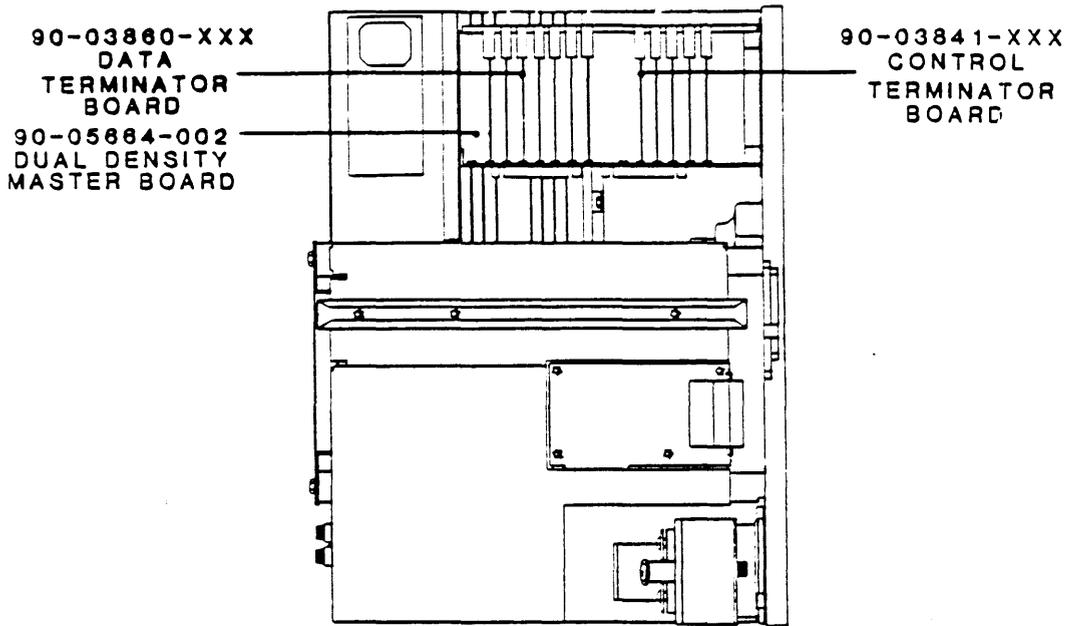
**Figure 2-18. Model 9100 (Left Side View),
