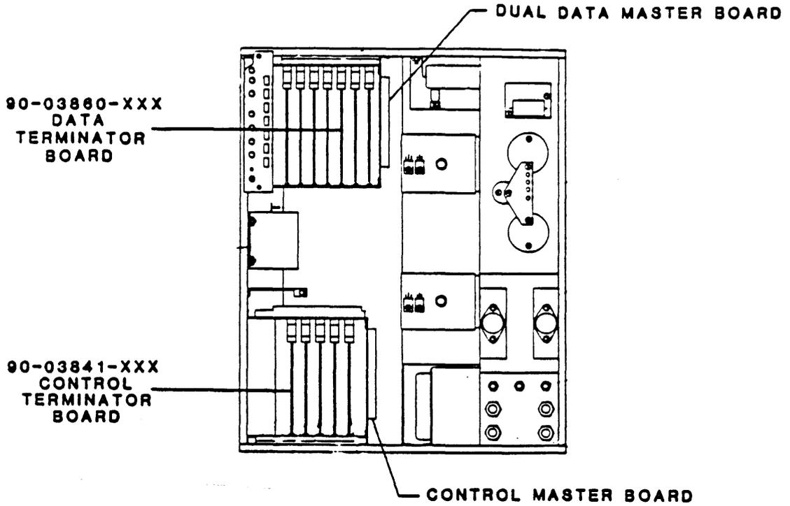
Figure 2-5. Model 9000 Drive Terminator Boards
