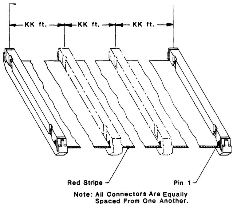
Figure 2-8. Cable Assembly P/N 90-04999-NLL For Daisy Chain, Typical For Models 9100, 9300, 9700 and/or 9800
