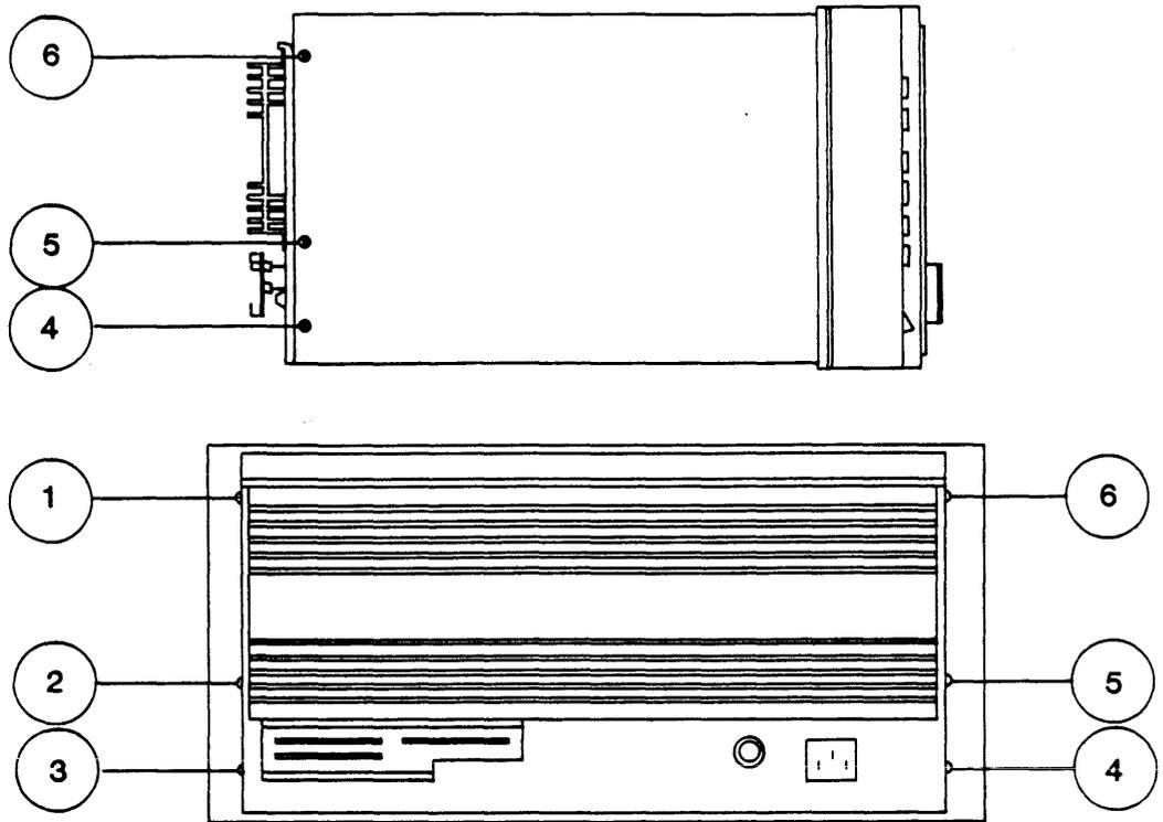
**Figure 2-14. Model 9700/9800 Drive and Formatter Mounting Screws**
