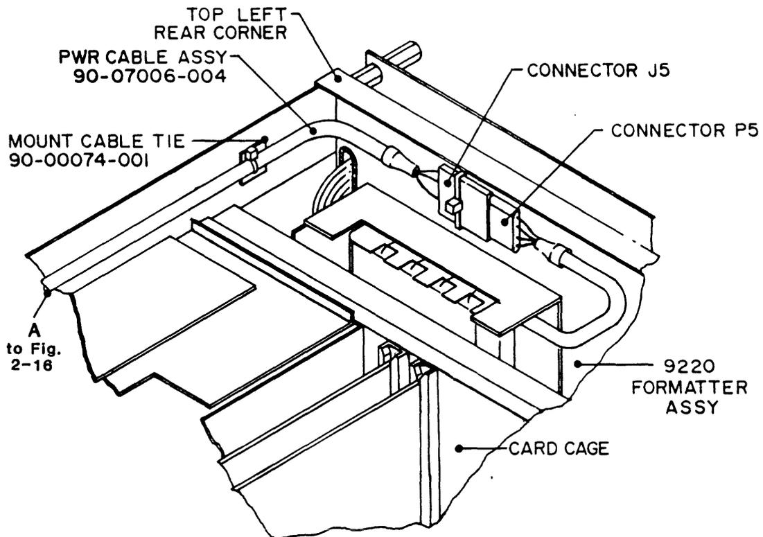
**Figure 2-17. Model 9700/9800 (Top Left Rear Corner View),
