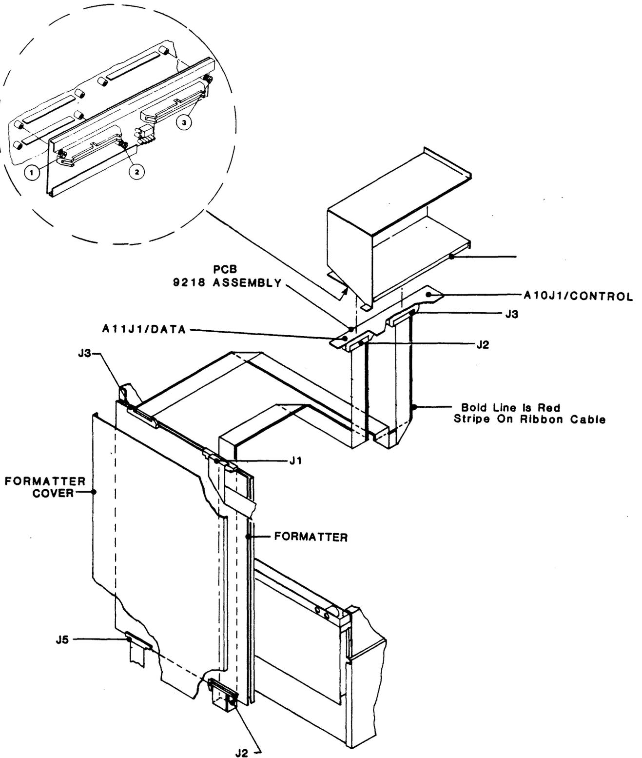
Figure 2-9. Model 9100 Drive to Formatter Interface (Rear View)
