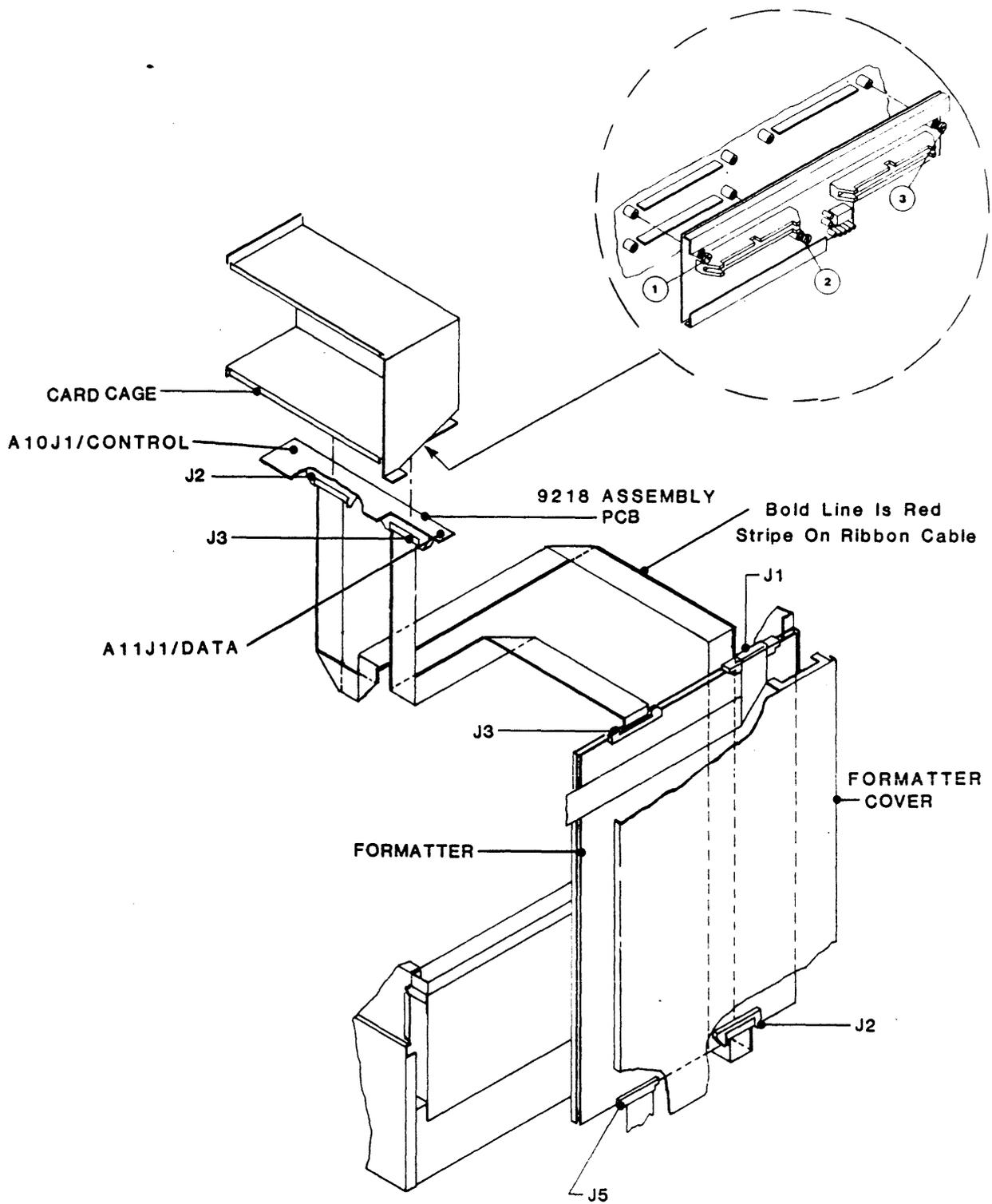
Figure 2-10. Model 9300 Drive to Formatter Interface (Rear View)
