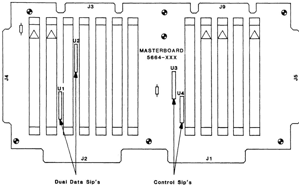
**Figure 2-22. 9100/9300 Drive Master Board, Terminator Single In-line Packages (SIP's)**
