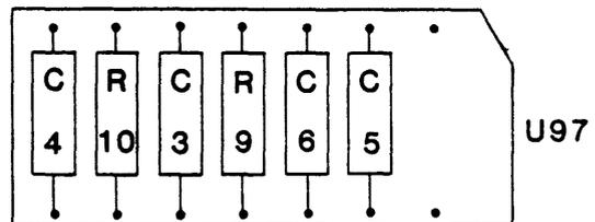
**Figure 1-3 Speed Selection Header**
