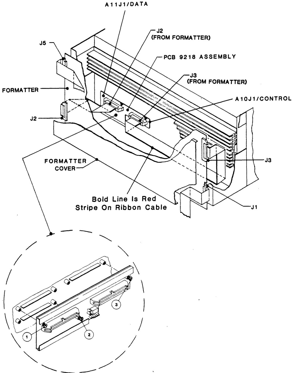
Figure 2-13. Models 9700/9800 Drives to Formatter Interface (Rear View)
