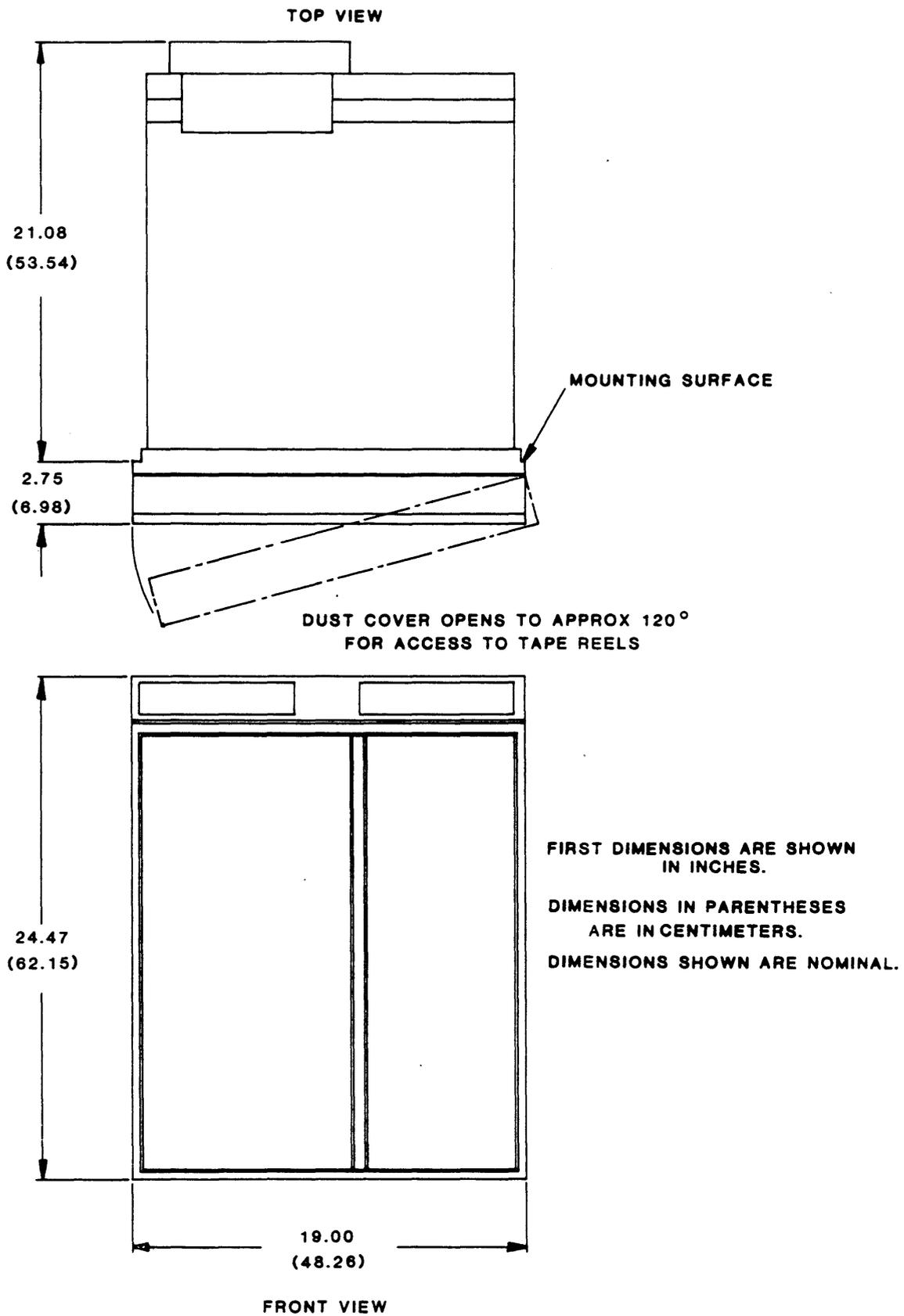
**Figure 2-25. Dimensions, Model 9300 with Embedded Formatter**
