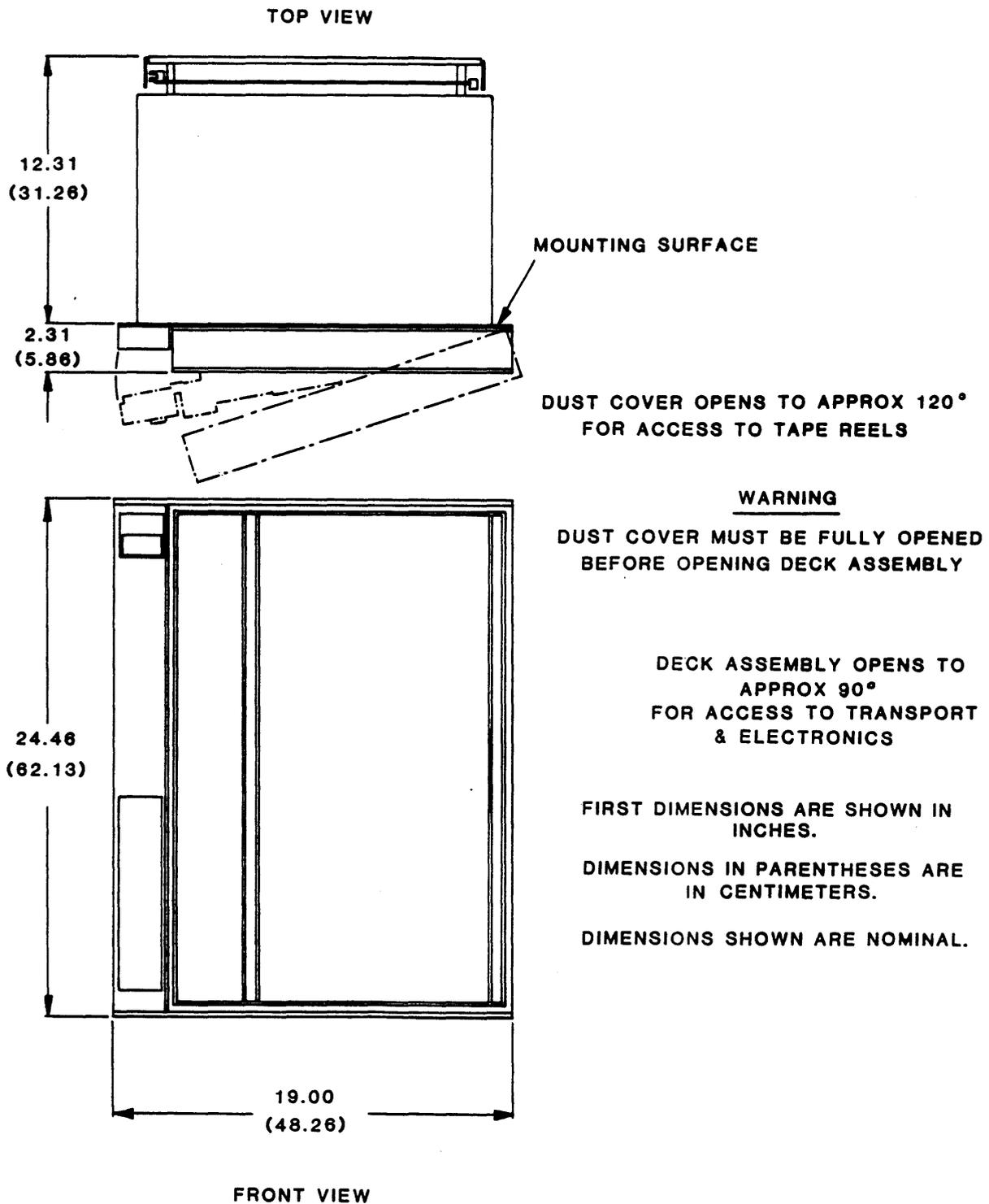
**Figure 2-23. Dimensions, Model 9000 with Embedded Formatter**
