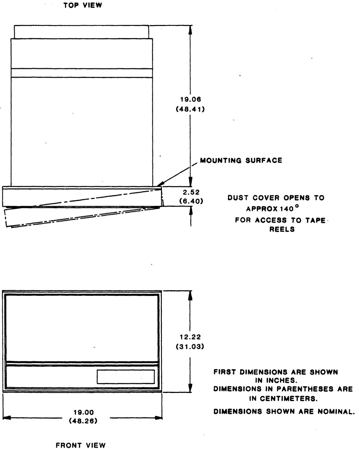
**Figure 2-27. Dimensions, Model 9800 with Embedded Formatter**
