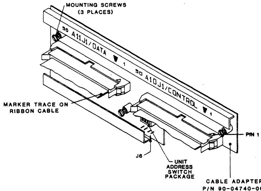
Figure 2-7. Cable Adapter Assembly (Kit) P/N 90-04970-NKK
