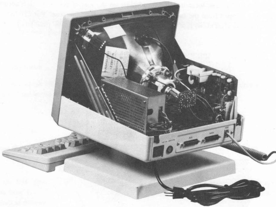
Figure 3-2: Kimtron Model KT-7 Video Terminal-Interior View
