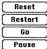
The **Reset** button clears all of the gateway's memory locations, leaving the gateway in the initial state. After resetting, the gateway waits for 25 seconds before it autoconfigures using PROM-resident AppleTalk Phase 1 protocols. When you click **Reset**, the following screen appears:
