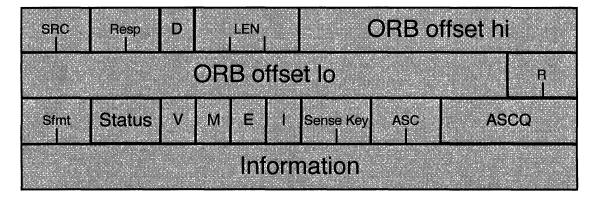
Sfmt **Status** 00 - only 1st 2 quadlets sent 02 - check condition 08 - busy V 0 M & E 0 ATAPI = 0ATA = attempted to move = more than 256 blocks Sense key ATAPI from request sense ATAPI from request sense ASC ATAPI from request sense ASCQ
