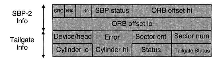
If a failure occurred before command completed SBP-2 Info contains the relevant information
