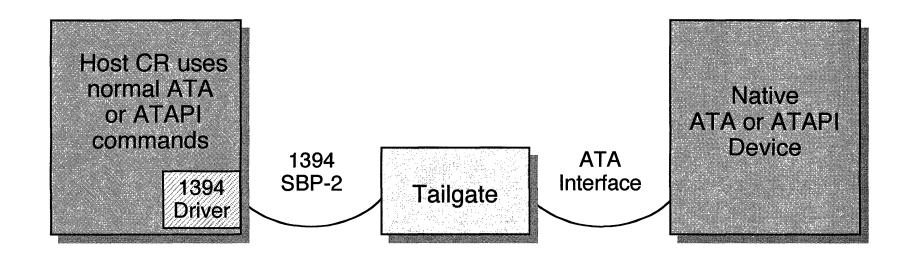
Translates between 1394 SBP-2 and ATA Separate board, chip on device, embedded in device controller
