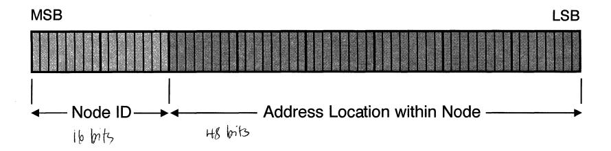
Each Node has 2<sup>48</sup> Bytes = 256 TeraBytes of Address Range
