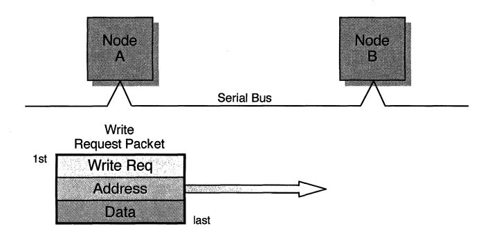
How does node A know if the packet is received correctly?
