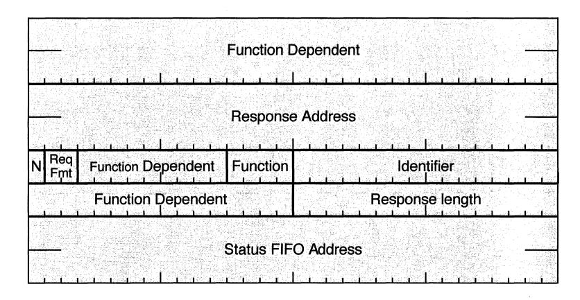
Note: All currently defined Management ORBs adhere to this format. However, the SBP-2 standard does not specify that future Management ORBs will necessarily follow this format. The standard specifies the format on a function by function basis.
